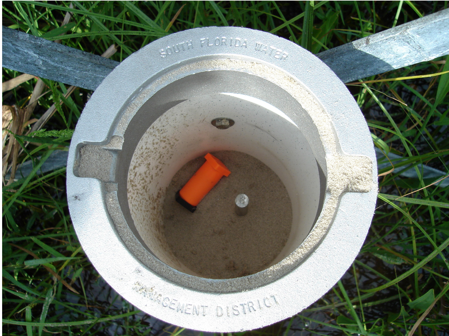
Nick Miller, Inc. Date of Photo: September 6, 2006 View: A top view of the benchmark
