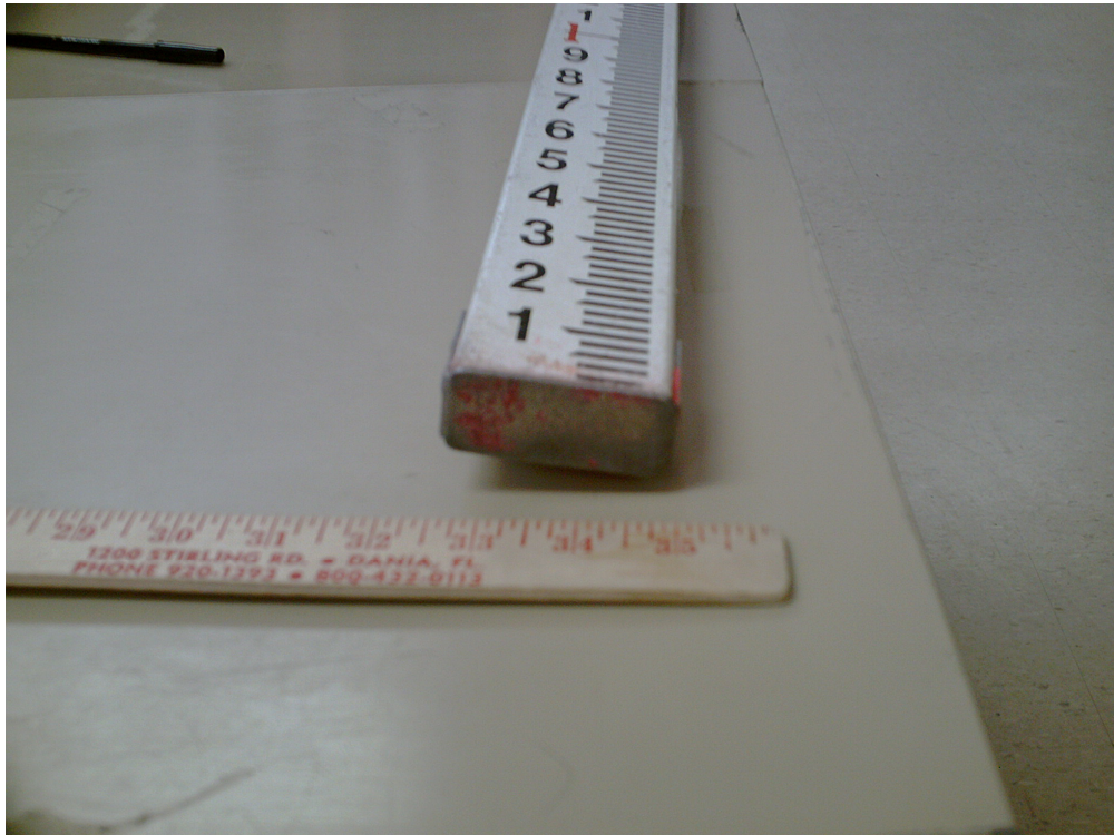
Figure 4: Foot of leveling staff
