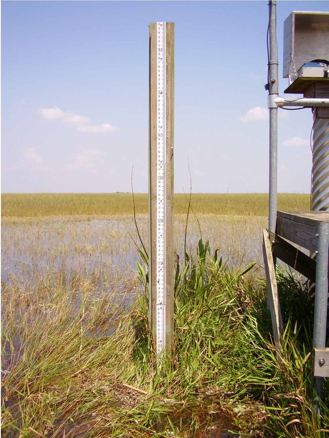
Figure 8: Photograph of the staff gauge at the northwest well cluster.
