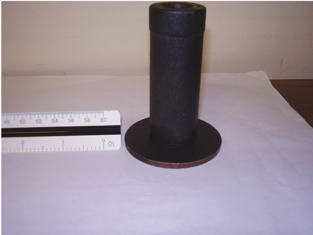
Figure 5: Side view of the prism pole shoe used for ground elevation measurement
