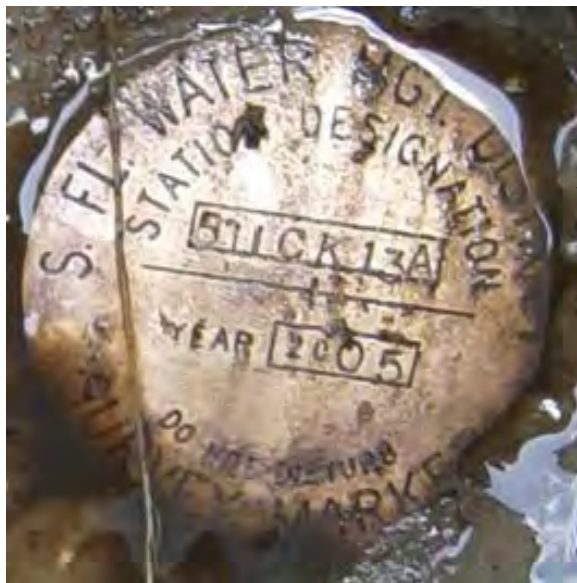
BUCK 13A 3" SURVEY DISK IN 12" CONCRETE MONUMENT
