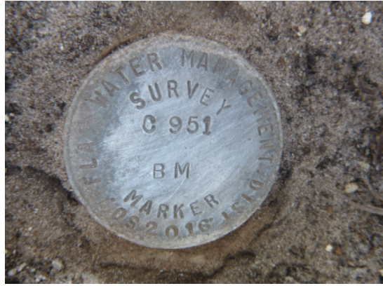
Benchmark set at wellsite for wells C-953, C-951 and C-948
