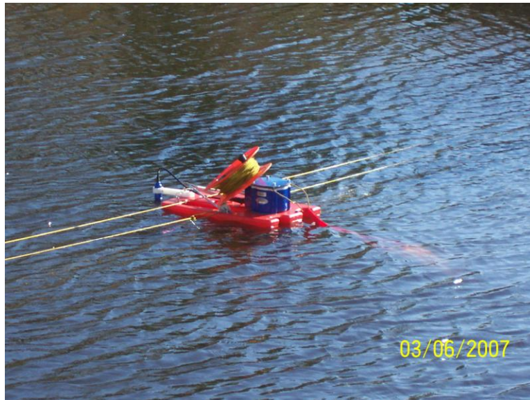
Figure 4. Launching of the StreamPro 2.4 MHz Acoustic Doppler
