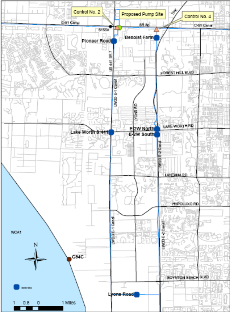
Figure 2. Project site and stage monitoring locations.
