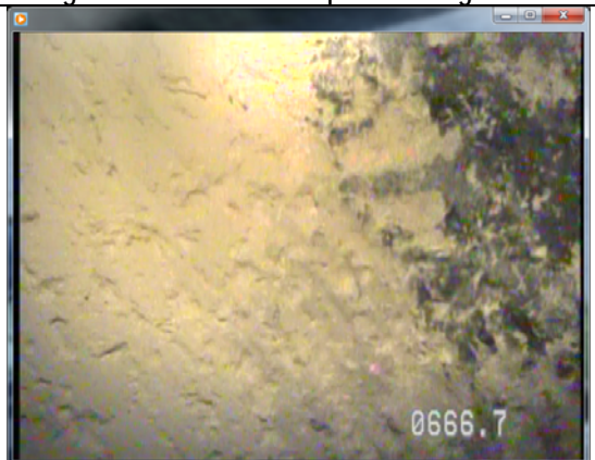
Depth: 666.7 Fine grained limestone with possible vugs.
