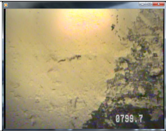
Depth: 799.7 Fine grained limestone with discoloration boundary.
