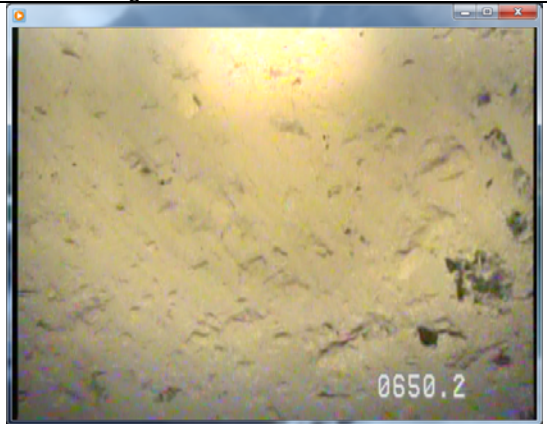
Depth: 650.2 Fine grained limestone with possible vugs.
