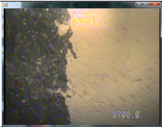
Depth: 700.0 Fine grained limestone with discoloration boundary.
