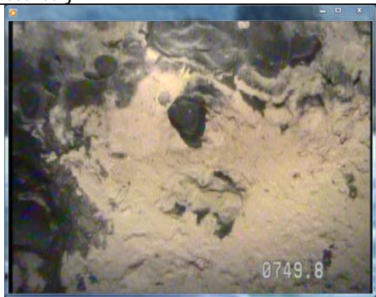
Depth: 749.8 Coarse grained limestone with moldic porosity.
