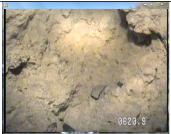
Depth: 620.9 Possible vugs or hollows.
