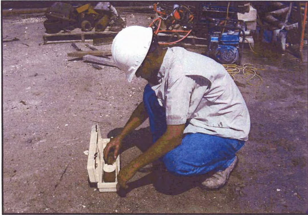
Figure 10 – Measuring Weight of Cement Grout Slurry
