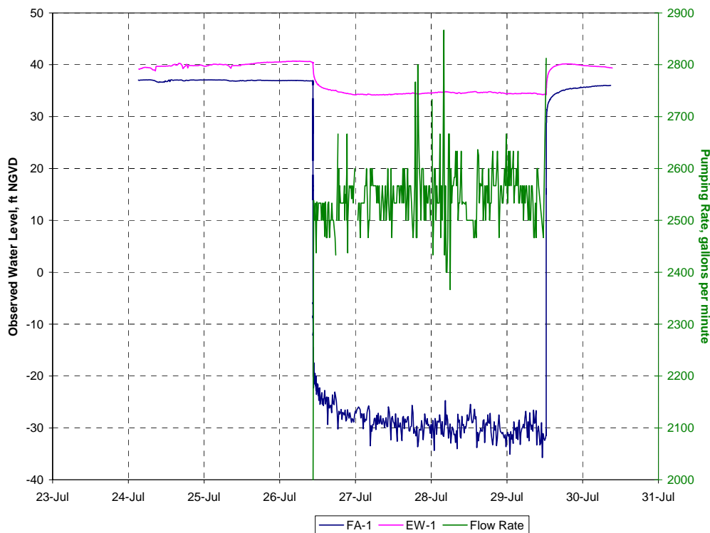
EXHIBIT 4-14 Water Levels Observed During Aquifer Performance Test
