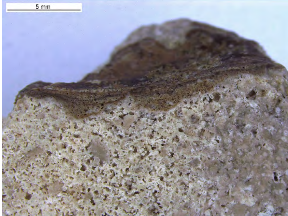
Photograph of slabbed core that shows the uppermost core sample of the Avon Park Formation with thin bands of dark coloration bounded by thin dished-shaped desiccation joint planes along the uppermost 2 millimeters (mm) and less of the Avon Park Formation. This is a depositional sequence boundary and corresponds to the depositional sequence boundary AP3.
