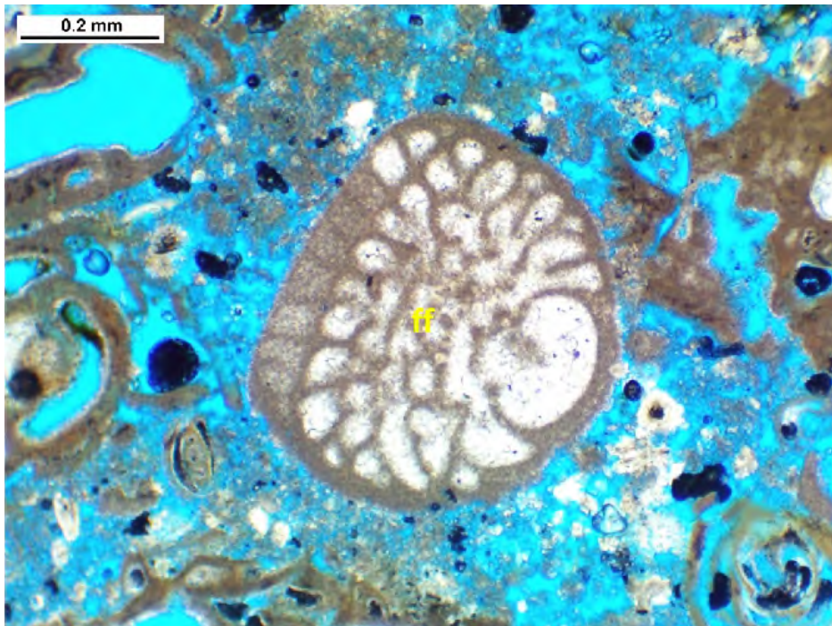
Photomicrograph from thin section G2984–1270.60 that shows a specimen of Fallotella floridana (ff). Driller's depth of thin section is 1,270.60 ft bls.
