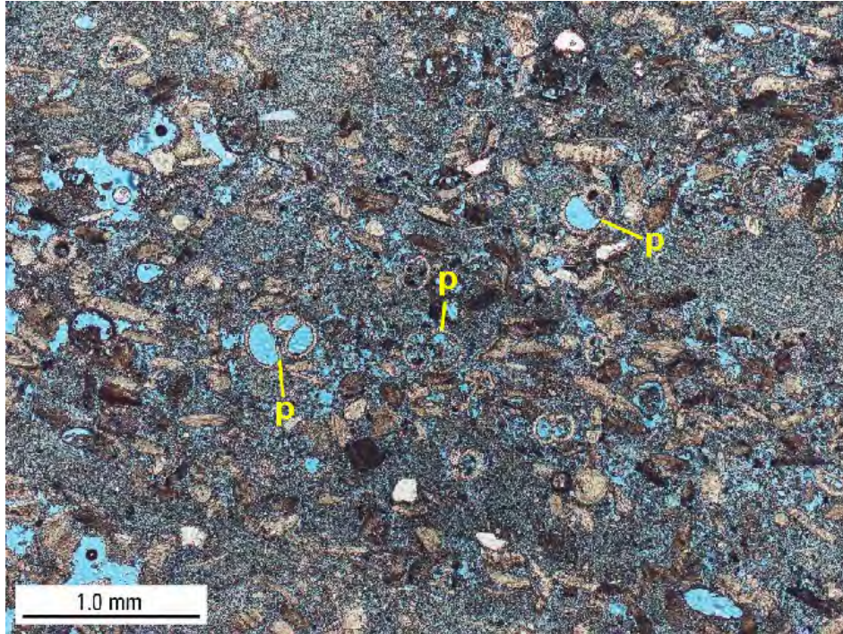
Photomicrograph from thin section G2984–817.57 that shows a skeletal and foraminifer wackestone and packstone lithofacies with planktic foraminifera (p). Driller's depth of thin section is 817.57 ft bls.
