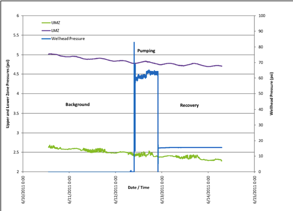
Figure 4-3 IW-1 Wellhead and UMZ and LMZ Pressures
