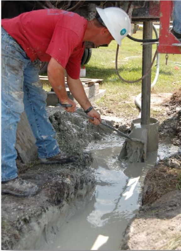
Collection of drill cutting samples during pilot hole of JE-1503.
