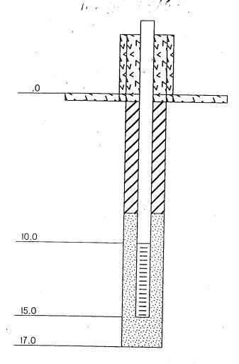
2" PVC riser with 1' stickup above 8" PVC casing filled with concrete
