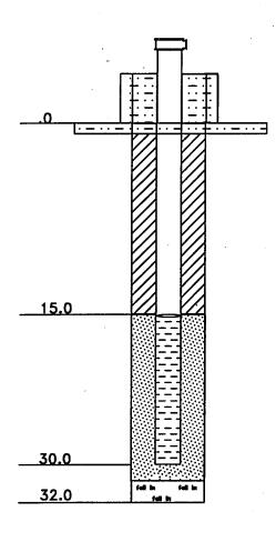
2" PVC riser with 1' stickup above 8" PVC casing filled with concrete.
