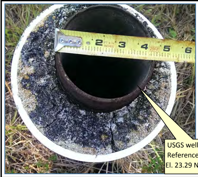
USGS well L-1137 Reference Point El. 22.94
