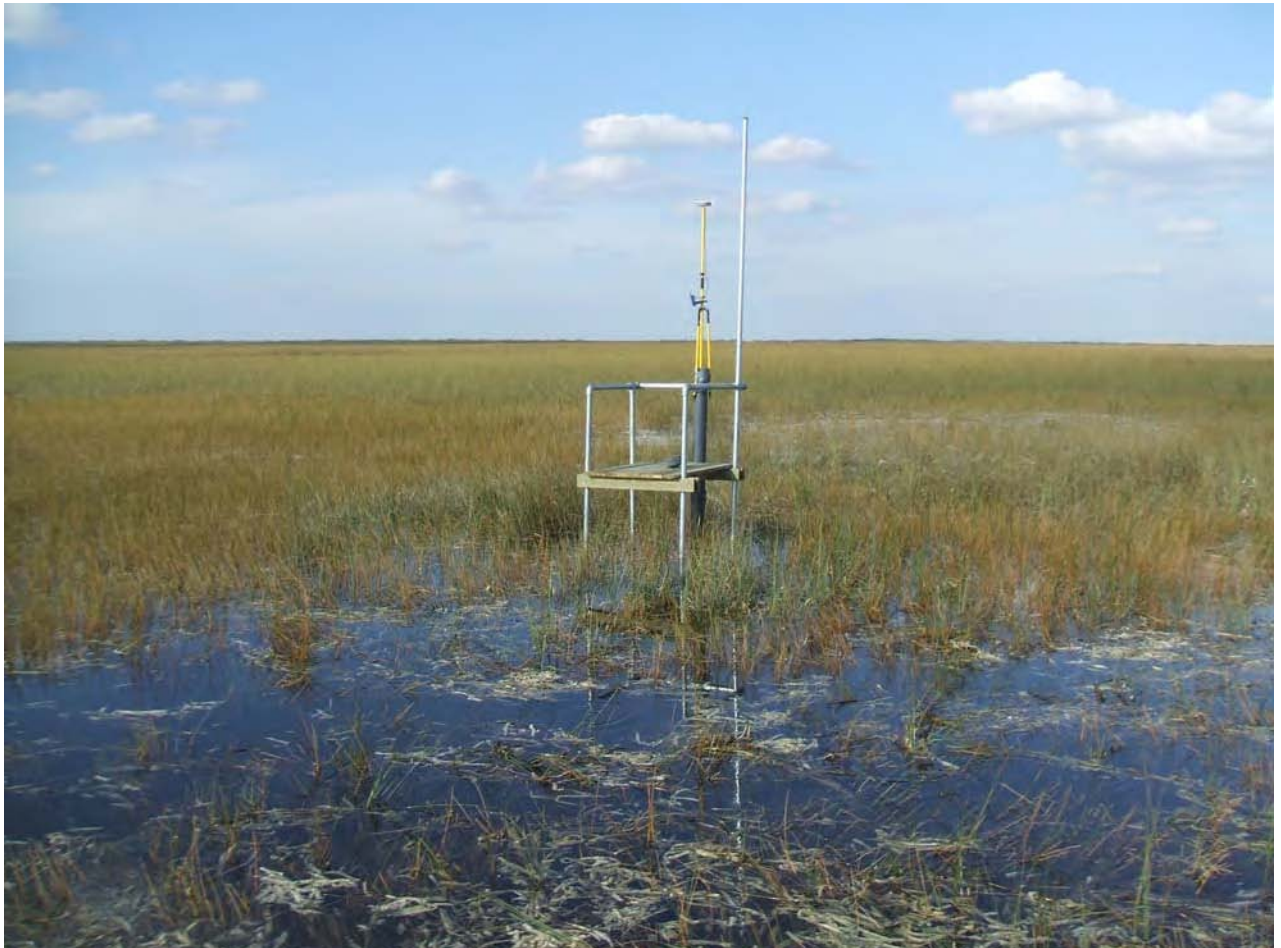
MONITORING WELL PLATFORM
