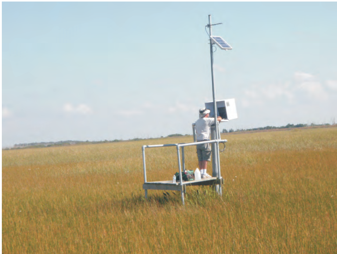
Dave Hire performs probe calibration at MW-5. The station transmits data to the telemetry base station at MW-1, located 4,800 ft away on the L-30 Levee.
