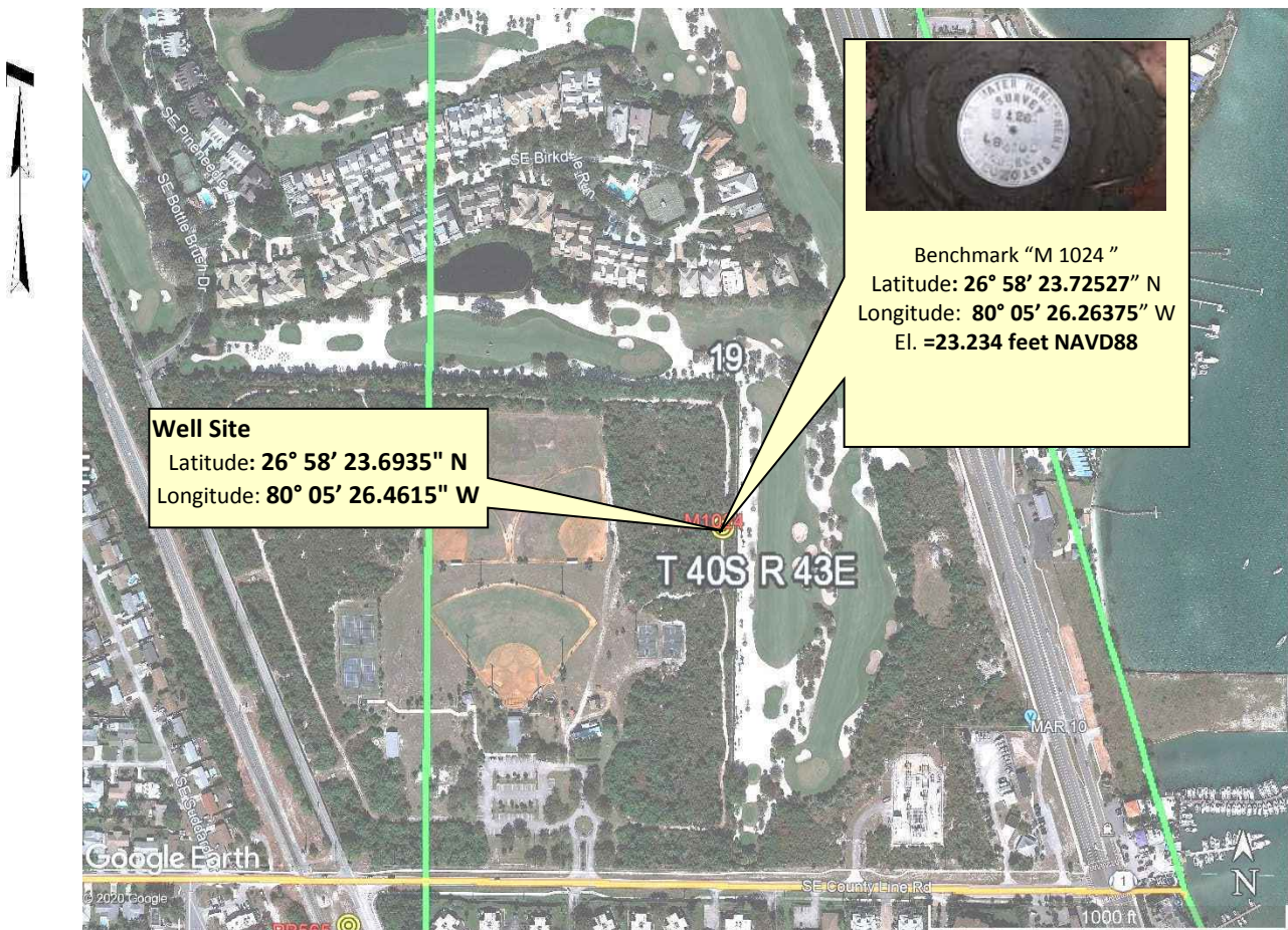
Aerial of Overall Well Site
