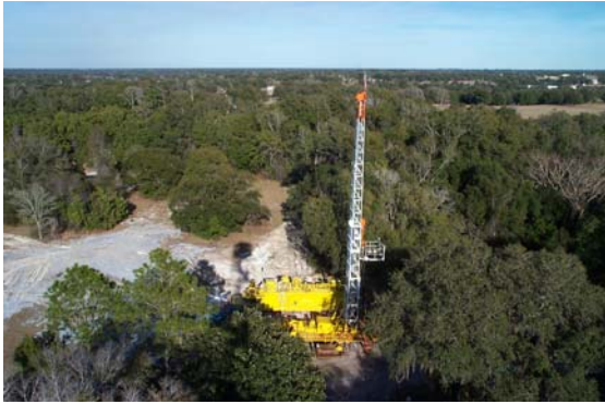
Gardner Denver 3500 drill rig, mud system and site as viewed from atop Forestry Fire Tower.
