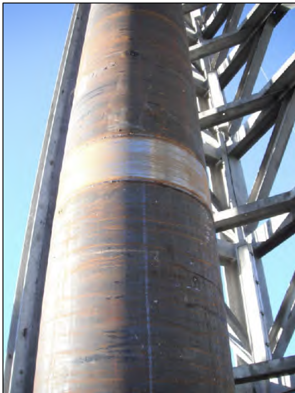
FIGURE 2-22: FEMALE PACKER PBR WELDED INSIDE 28-INCH CASING
