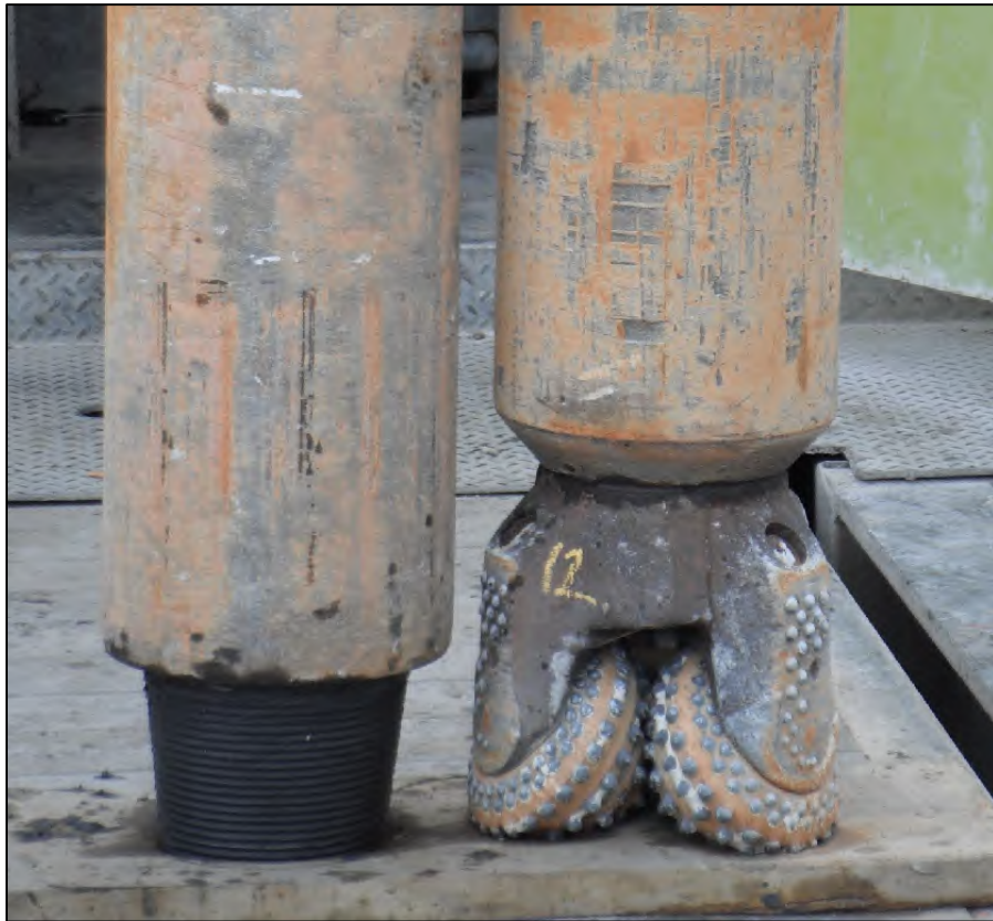
FIGURE 2-4: 12-INCH TRICONE DRILLING BIT
