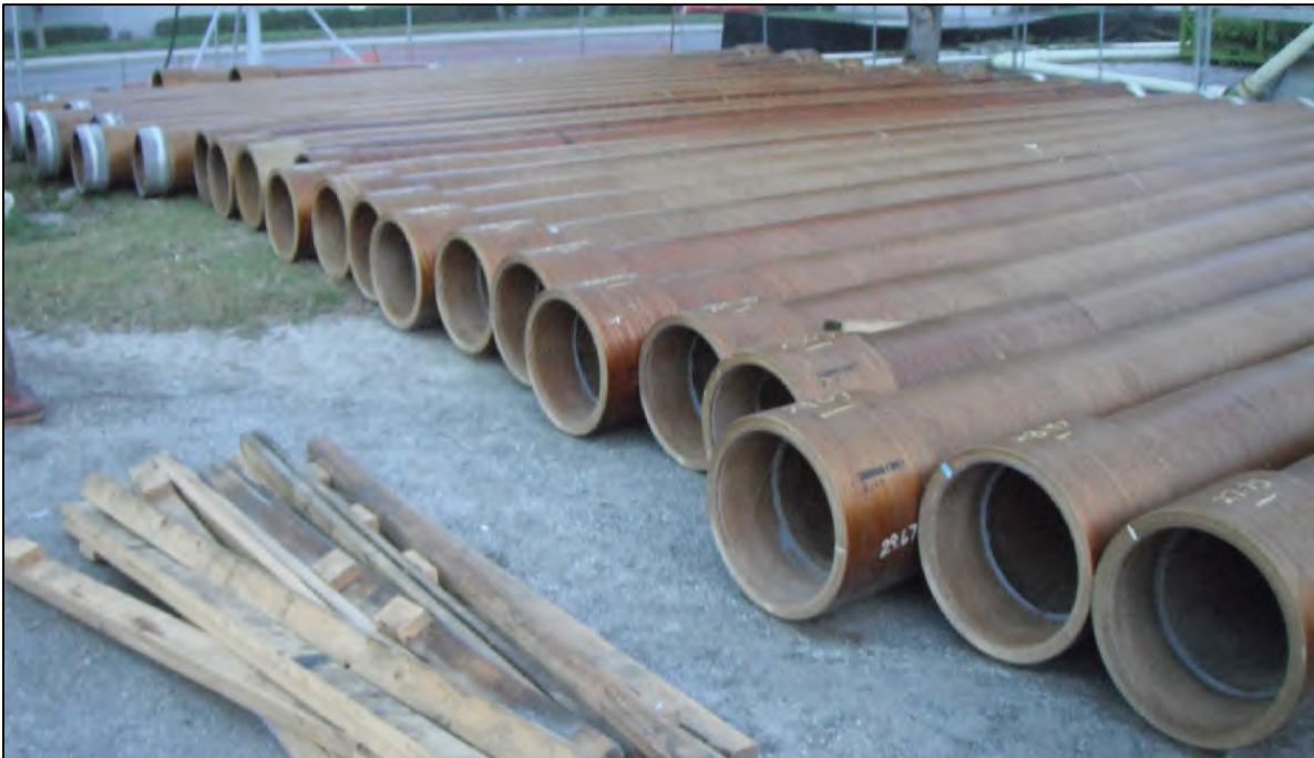
FIGURE 2-12: 18-INCH INJECTION WELL FRP TUBING
