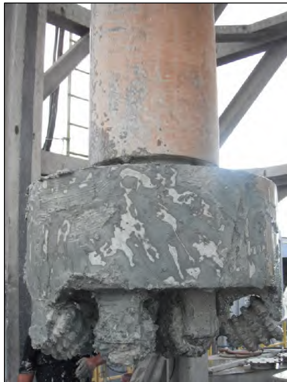
FIGURE 2-5: 56-INCH REAMING BIT
