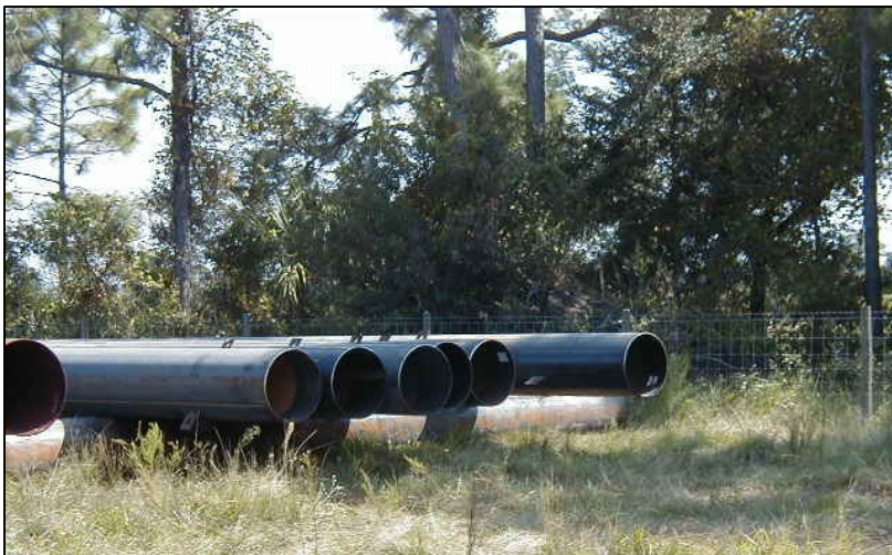
STEEL CASING : 20-INCH
