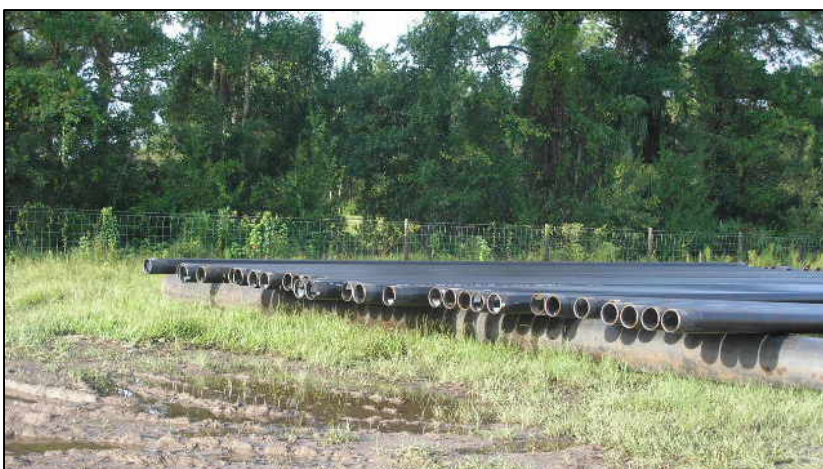
STEEL CASING : 8-INCH
