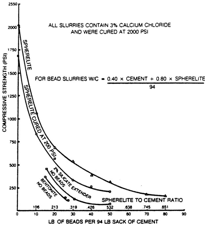
Fig. 1 - 24 hr 80°F (26°C) compressive strength for light weight slurries.
