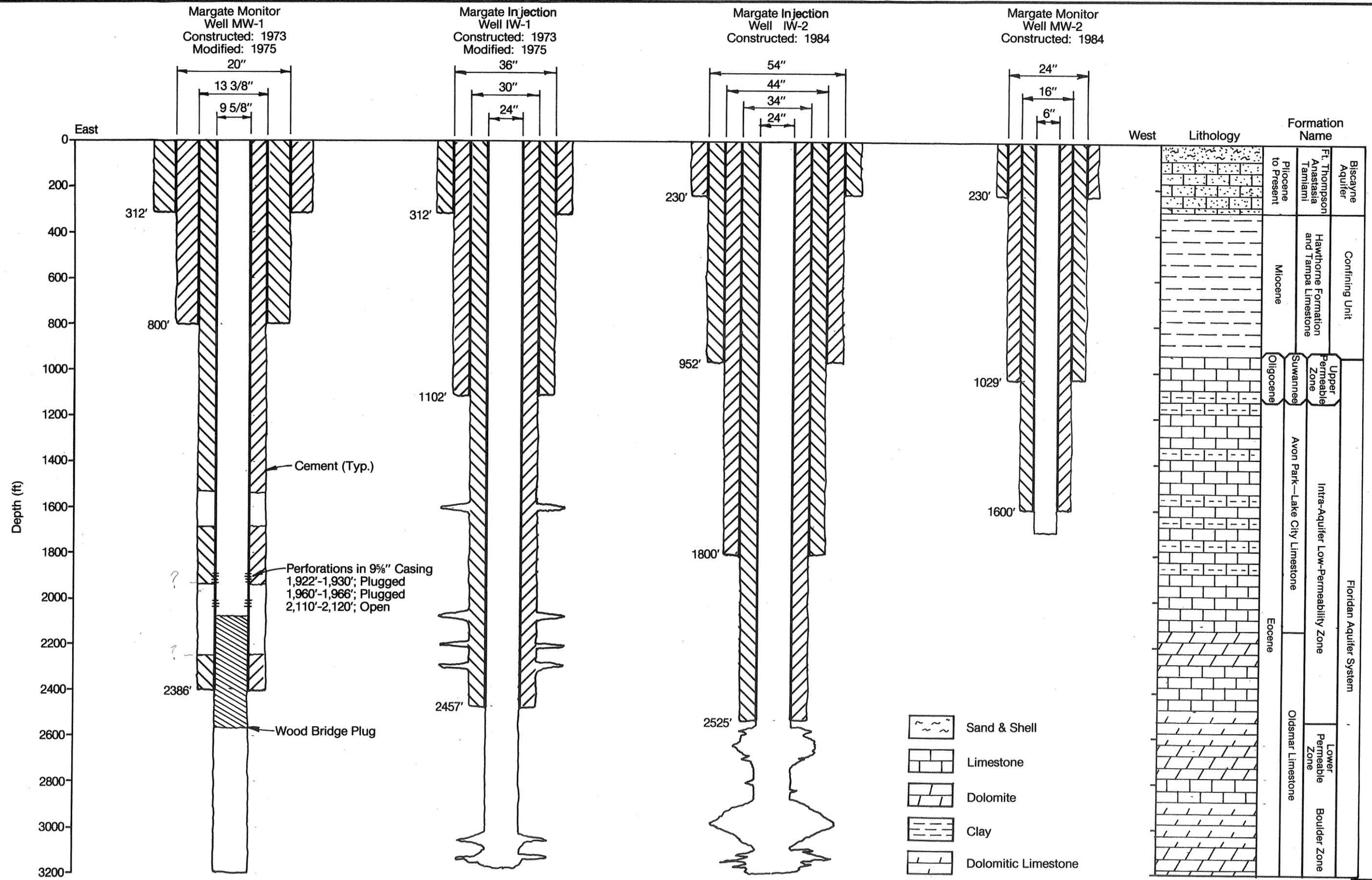
**FIGURE 6.** City of Margate Injection and Monitoring Wells, Summary of Construction Details.
