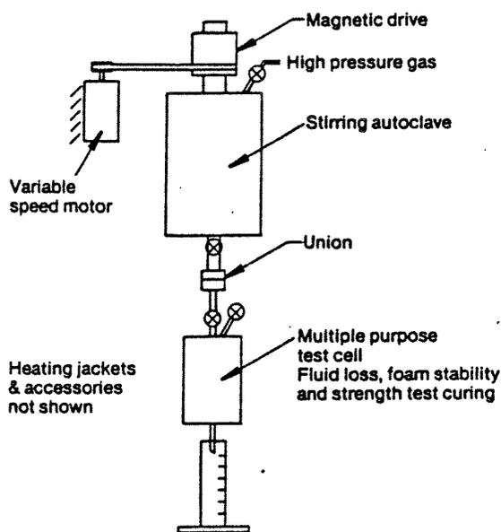
Fig. 2—Although most testing has been done under atmospheric preparation conditions, this high pressure foam slurry generation and testing apparatus has been used to confirm results. Few major differences have been noted between the two testing conditions.
