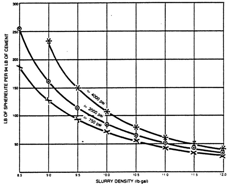
Fig. 3 - Pounds of Spherelite required per sack of cement to prepare lightweight cement slurries under varying pressures.
