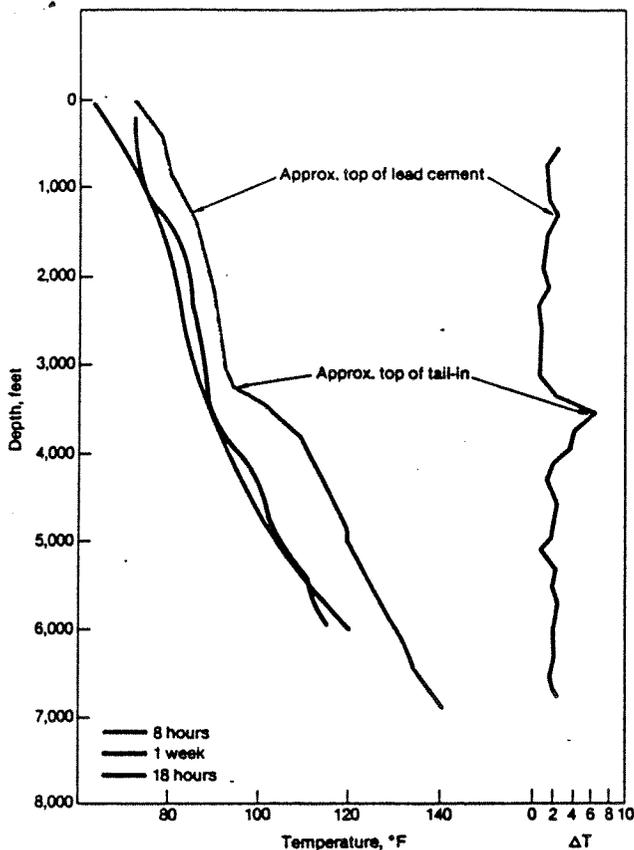
Fig. 10—Typical temperature survey of a West Texas Spraberry well shows how various cement interfaces are located behind casing.
