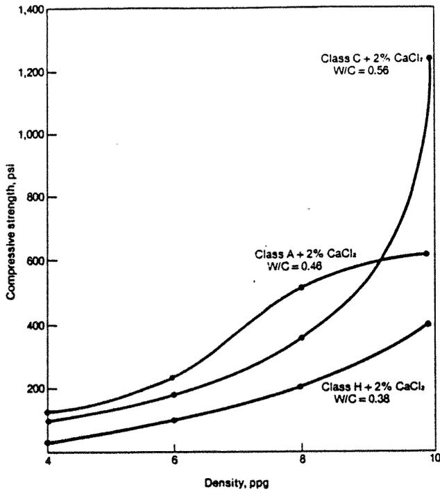
Fig. 3—This graph of results from a 24-hour compressive strength development test run at 100° F illustrates how physical and chemical properties can affect foam cement strength development.
