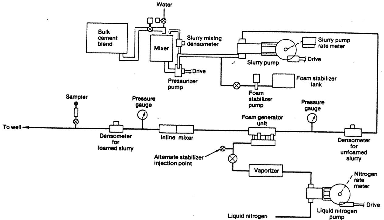
Fig. 5—Equipment needed in the field to mix and monitor foam cements is very similar to that used in conventional jobs. The major exceptions are the foam generator inserted into the slurry discharge line and the nitrogen unit.
