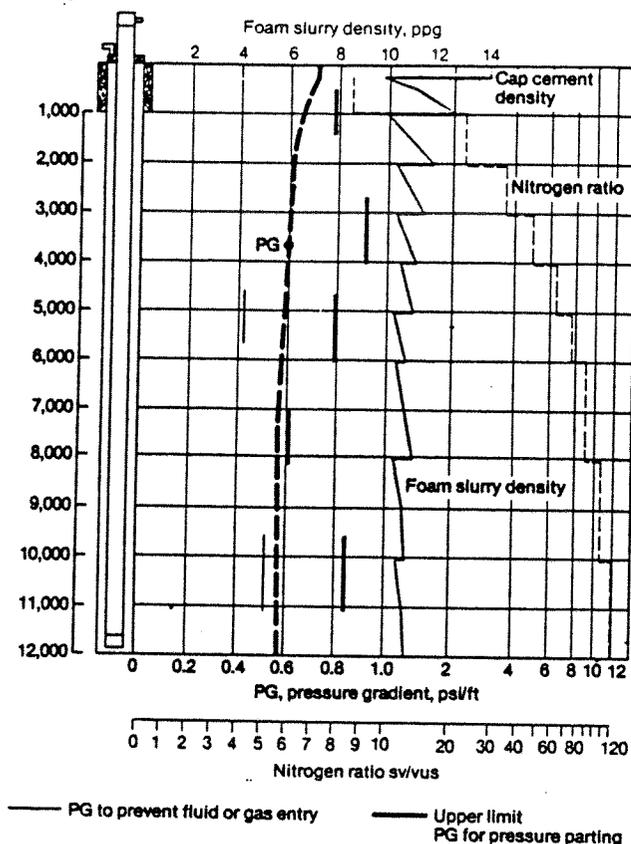
Fig. 9—In this example, the nitrogen ratio was adjusted with depth, but a 200-ft, 14.1 ppg cement cap was also used.
