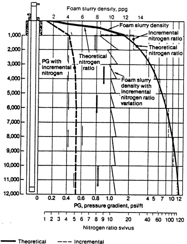
Fig. 8—To obtain a constant density foam cement, the nitrogen ratio must be adjusted with depth. In this example, the ratio is changed every 1,000 ft at shallower depths and at every 2,000 ft at greater depths to obtain an average slurry density of 10.5 ppg.
