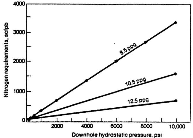
Fig. 4.—Nitrogen requirements for preparing an 8.5 ppg foam cement. Values are in standard cubic feet of N<sub>2</sub> per barrel of 14.8 ppg cement.
