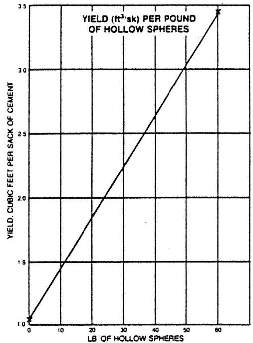
Fig. 2 - Yield (ft³/sk) per pound of Spherelite additive.
