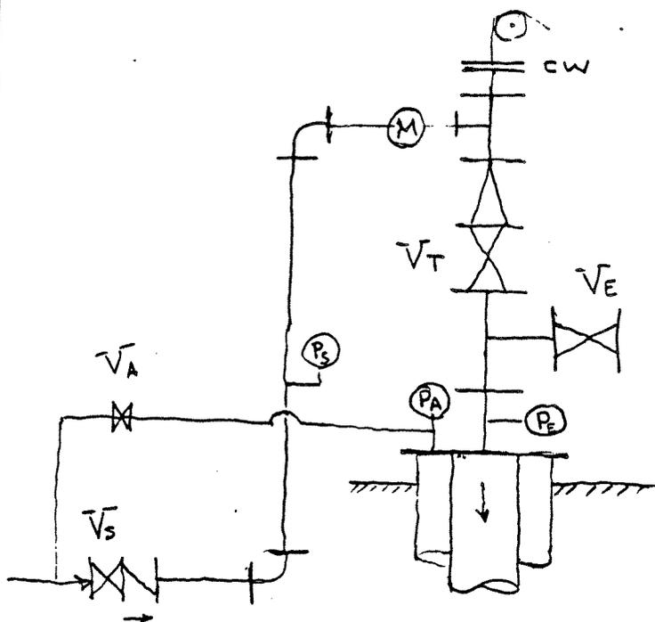
Program: Start with  $V_A$ ,  $V_S$  and  $V_T$  closed,  $V_E$  open. Then:
