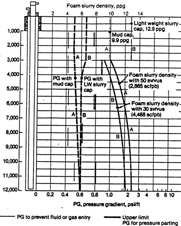
Fig. 7—To overcome problems illustrated by Fig. 6, a cap of mud or heavier cement can be used with constant gas rate foam cements.
