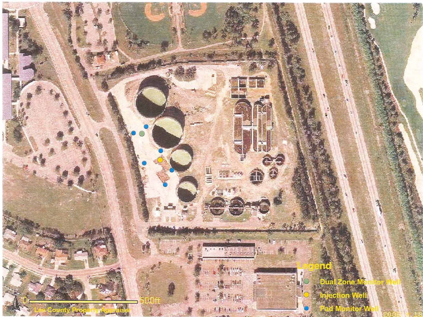
Figure 2-1 Locations of IW-1, DZMW-1, and Pad Monitor Wells at the Three Oaks WWTTP Site
