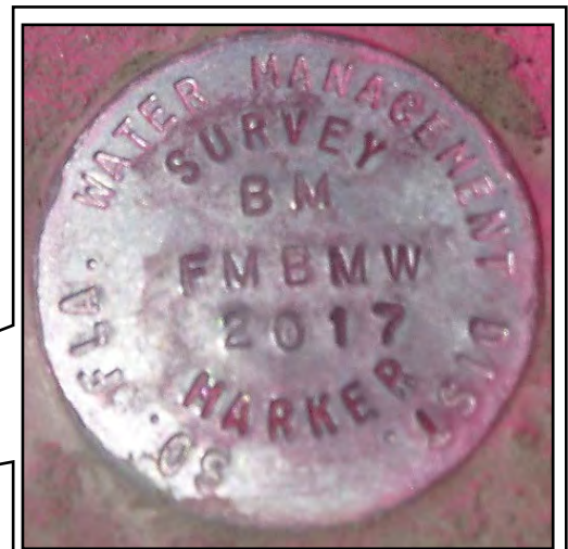
Aluminum cap stamped "FMBMW 2017" El. 6.201 NAVD88 El. 7.376 NGVD29 (Corpscon)
