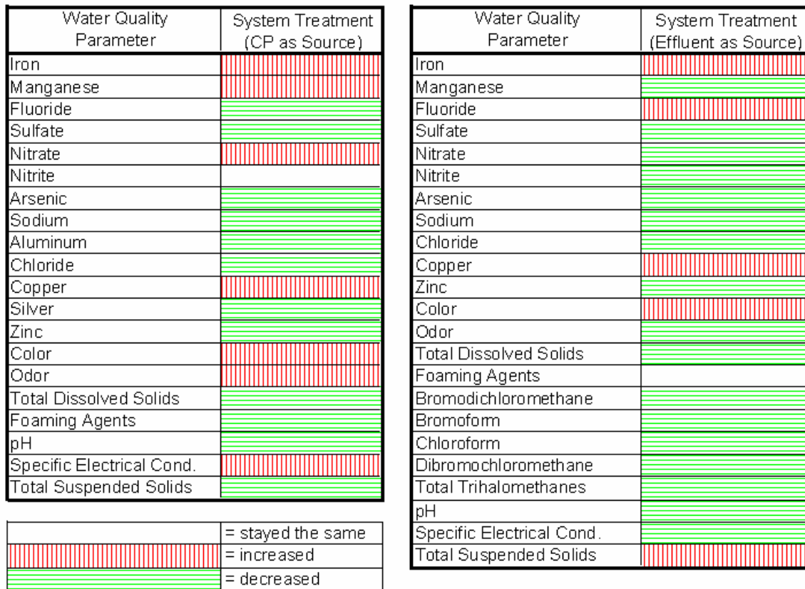
Figures 19 (left) and 20 (right). Changes in Water Quality in the Water Flowing through the System Using Cooling Pond Water or Effluent as Source Water.
