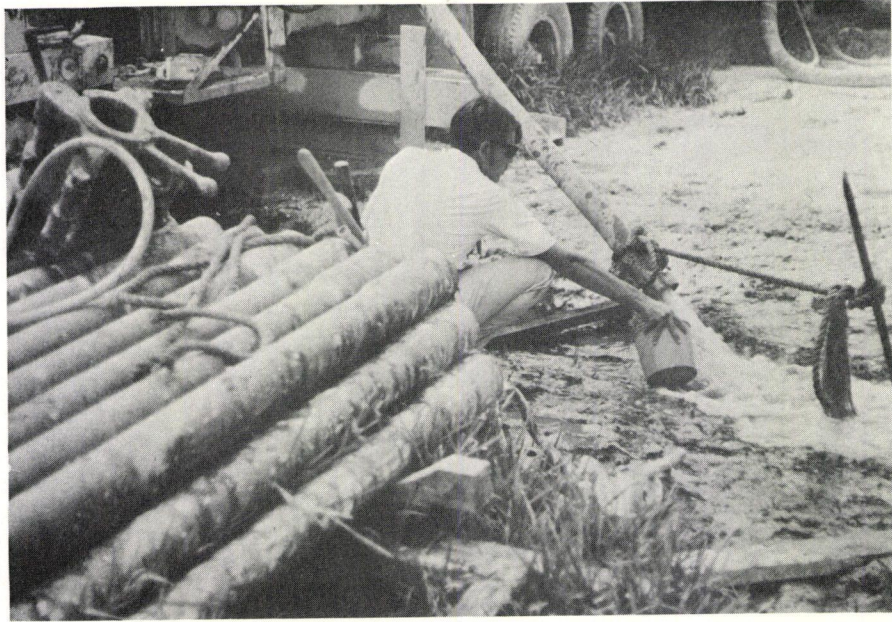
Collection of Water Samples from Reverse-Circulation Discharge
