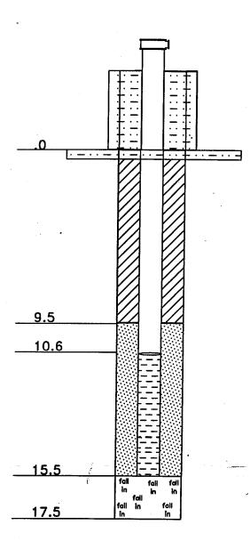
2" PVC riser with 1' stickup above 8" PVC casing filled with concrete
