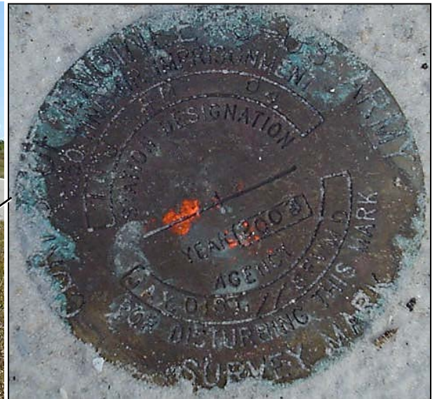
Bronze C. of E. Disk stamped "INJ BM O4" El. 4.976 NAVD88 El. 6.161 NGVD29
