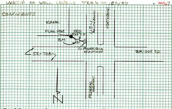
BH BRIDGE RD#1 IS A S. B. D. SXS "CONC RIW MON AT THE N.W. COE OF US-1 (FERERAL HIGHWAY)+ SE-708 (BRIDGE RD) ELEU. IS ON TOP OF S.W. COR OF MON MON IS 2. ABOVE GIRND LEVEL AT THE S.E. COR. OF BANK PARKING LOT MON IS 12.0' S.E OF A FLAGE POLE AND 7.0' N.W. OF APOWER POLE W/AGUY WIRE
