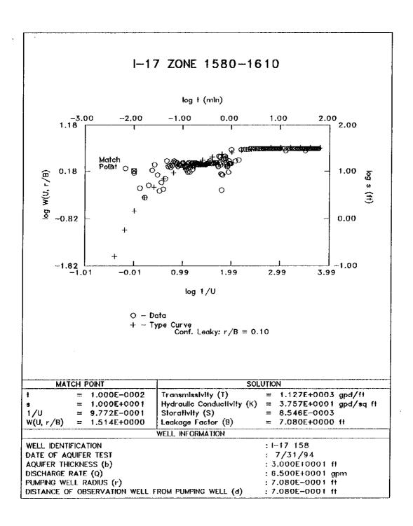
Figure 3.--Theis Leaky Curve Analysis I-17, zone 1580 to 1610
