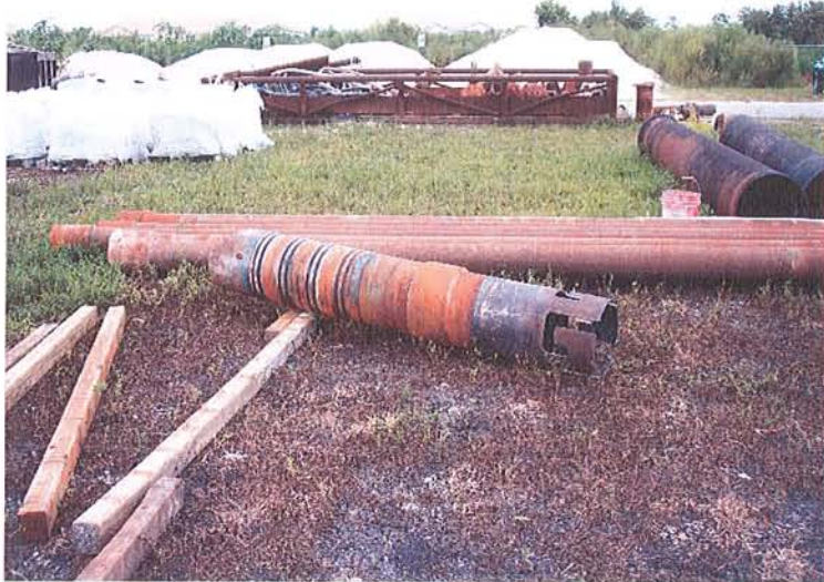
Liner Hanger Packer removed from IW-1 to be filled with cement and used as a bridge plug.
