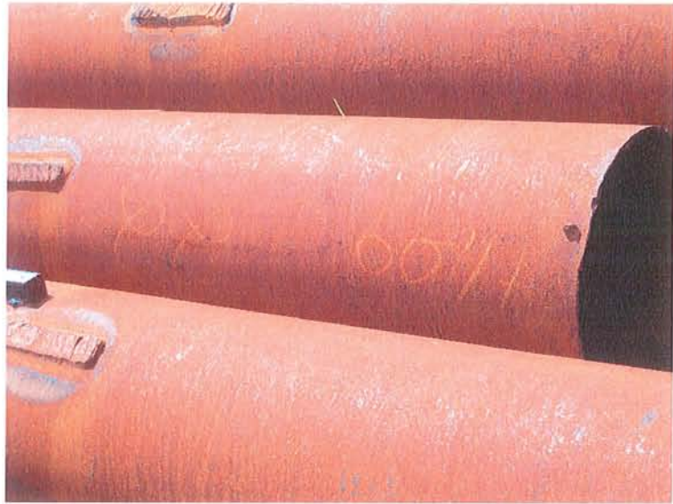
Original grease marker numbers on steel tubing removed from IW-2.
