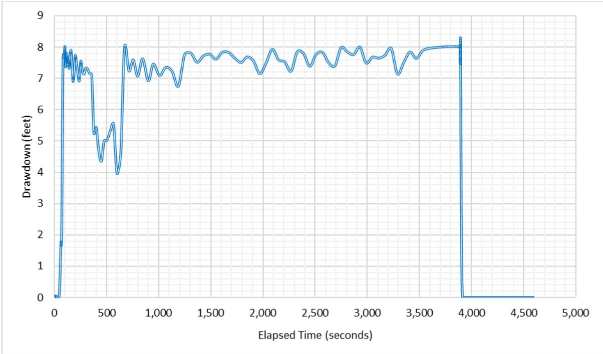
Figure 5. Drawdown and recovery graph of the M-1236 test.
