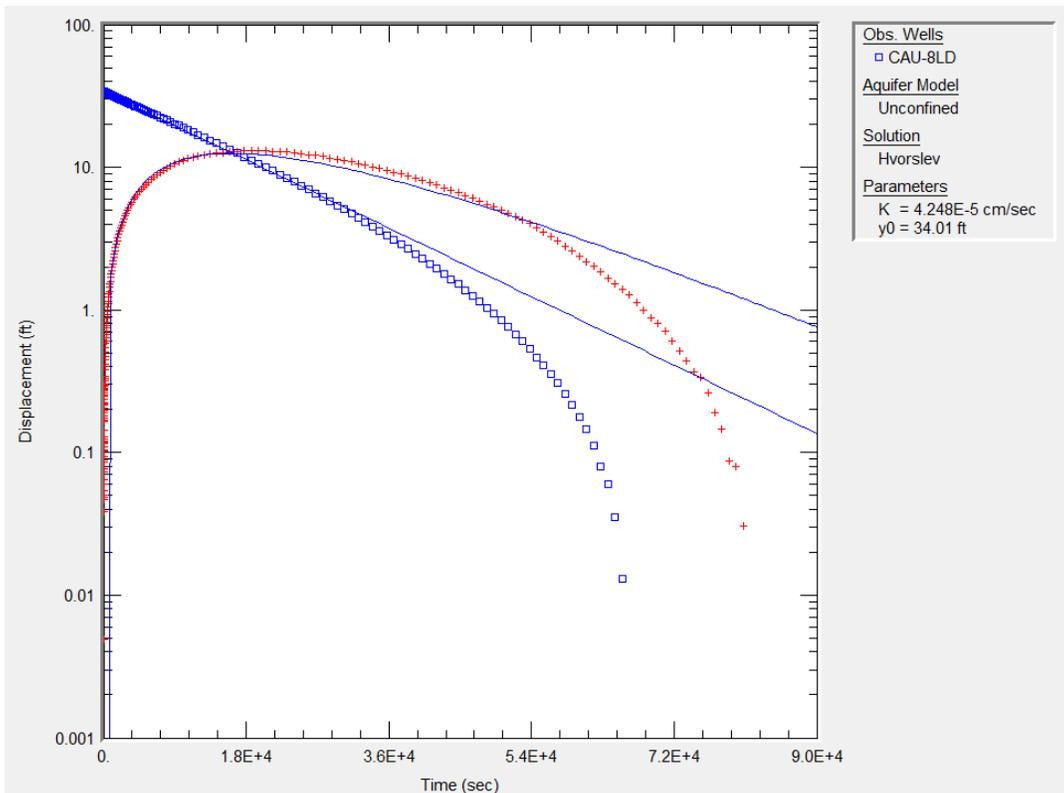
Figure 9. Analysis of CAU-8LD repeat test data using the Hvorslev (1951) solution.
