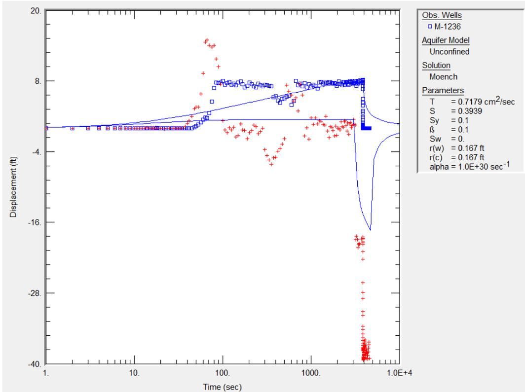
Figure 8. Analysis of M-1236 test data using the Moench (1997) solution.
