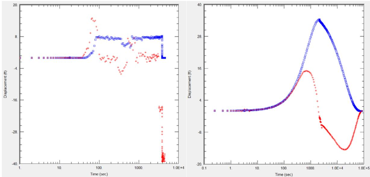
Figure 7. Displacement (blue) versus time with derivative (red) for M-1236 (left) and CAU-8LD repeat test (right).
