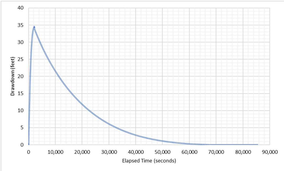
Figure 6. Drawdown and recovery graph of the CAU-8LD repeat test.
