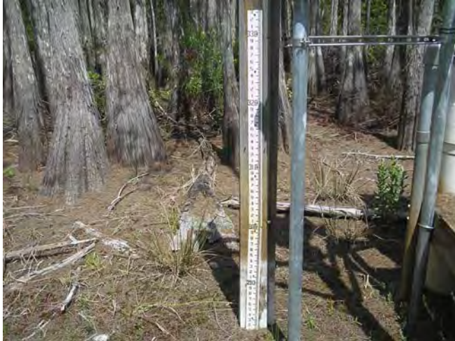
STG1 & STG2 STAFF GAUGE LOOKING NORTH
