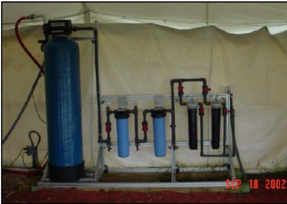
Figure 4-6 -- Photo showing Ionics serial filtration system with 20-, 5-, 1-, and 0.45- \mu m cartridge filters (left to right).
