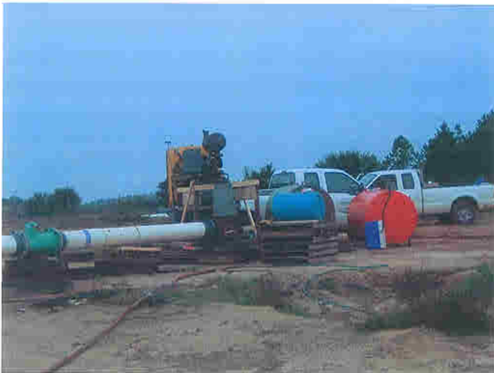
Photograph D-14 Pumping test set-up
