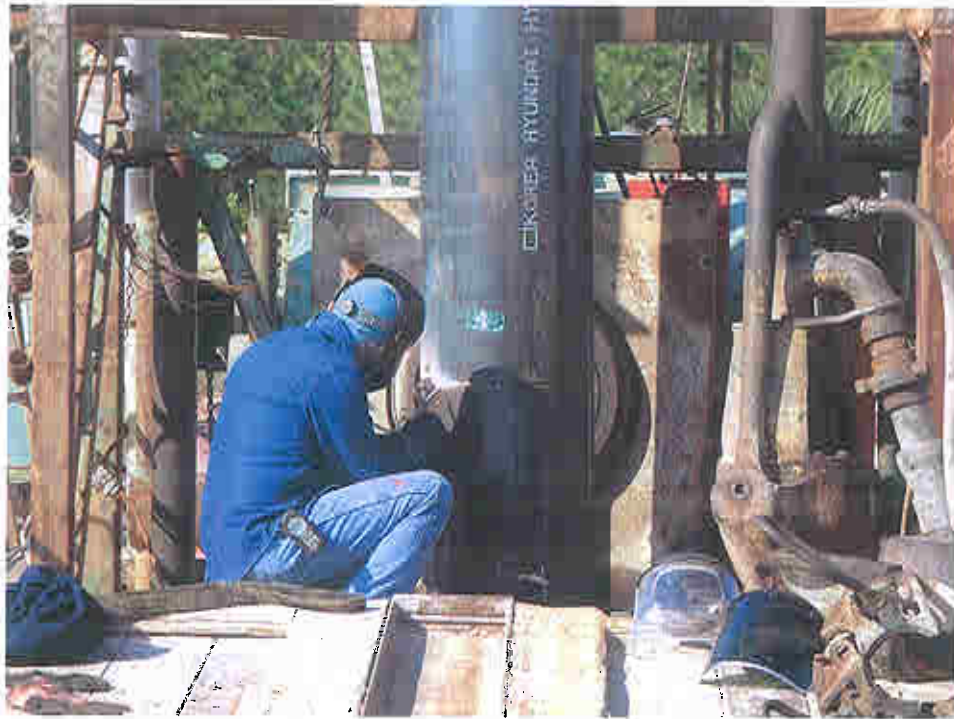
Photograph D-12 - Left-hand back-off casing tool
