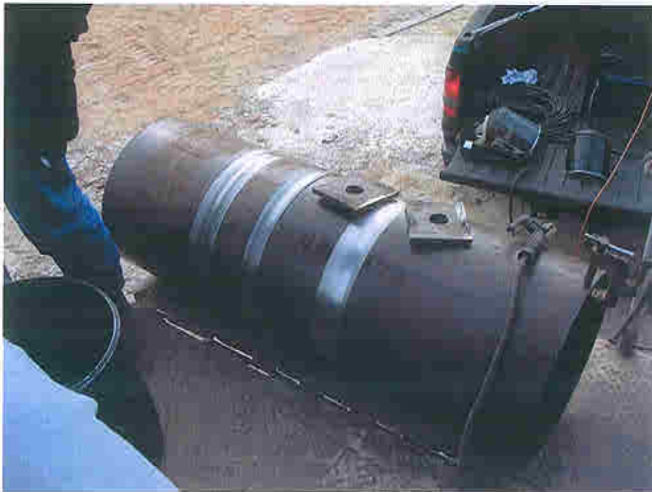
Photograph D-12 - Left-hand back-off casing tool
