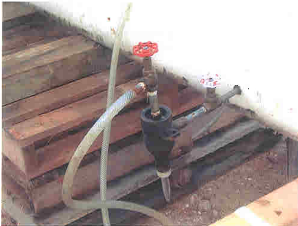
Photograph D-16 - Pumping test Rossum sand sampler
