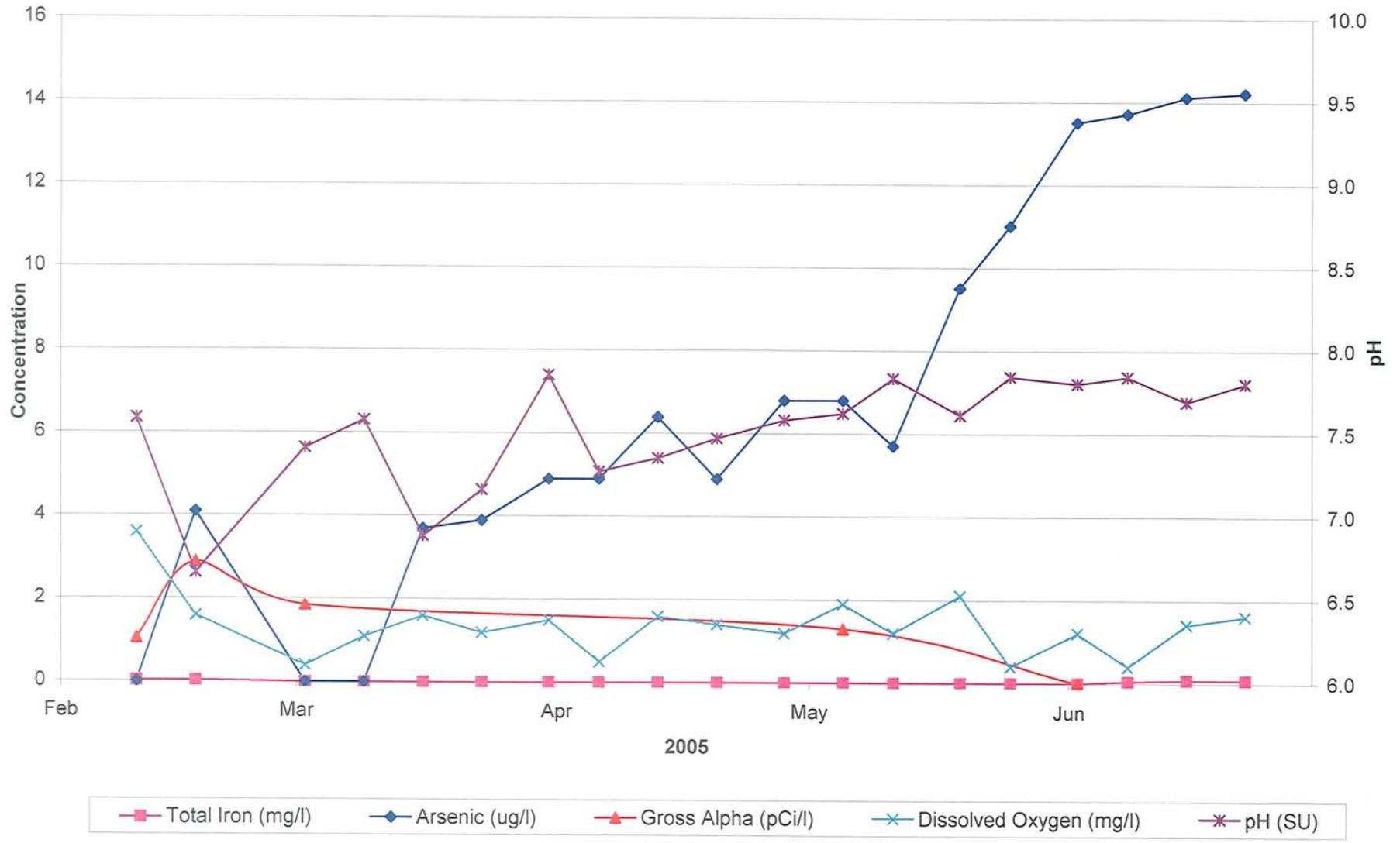
FIGURE 2-17. PLOT OF RECOVERED WATER QUALITY FROM WELL ASR-2 DURING CYCLE 4 (PART 1)
