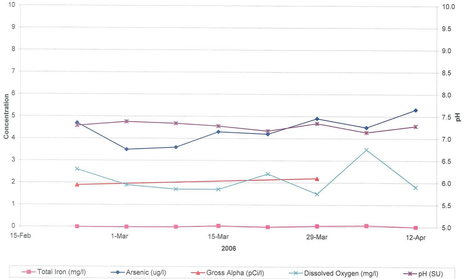
FIGURE 3-25. PLOT OF RECOVERED WATER QUALITY FROM WELL ASR-5 DURING CYCLE 5
