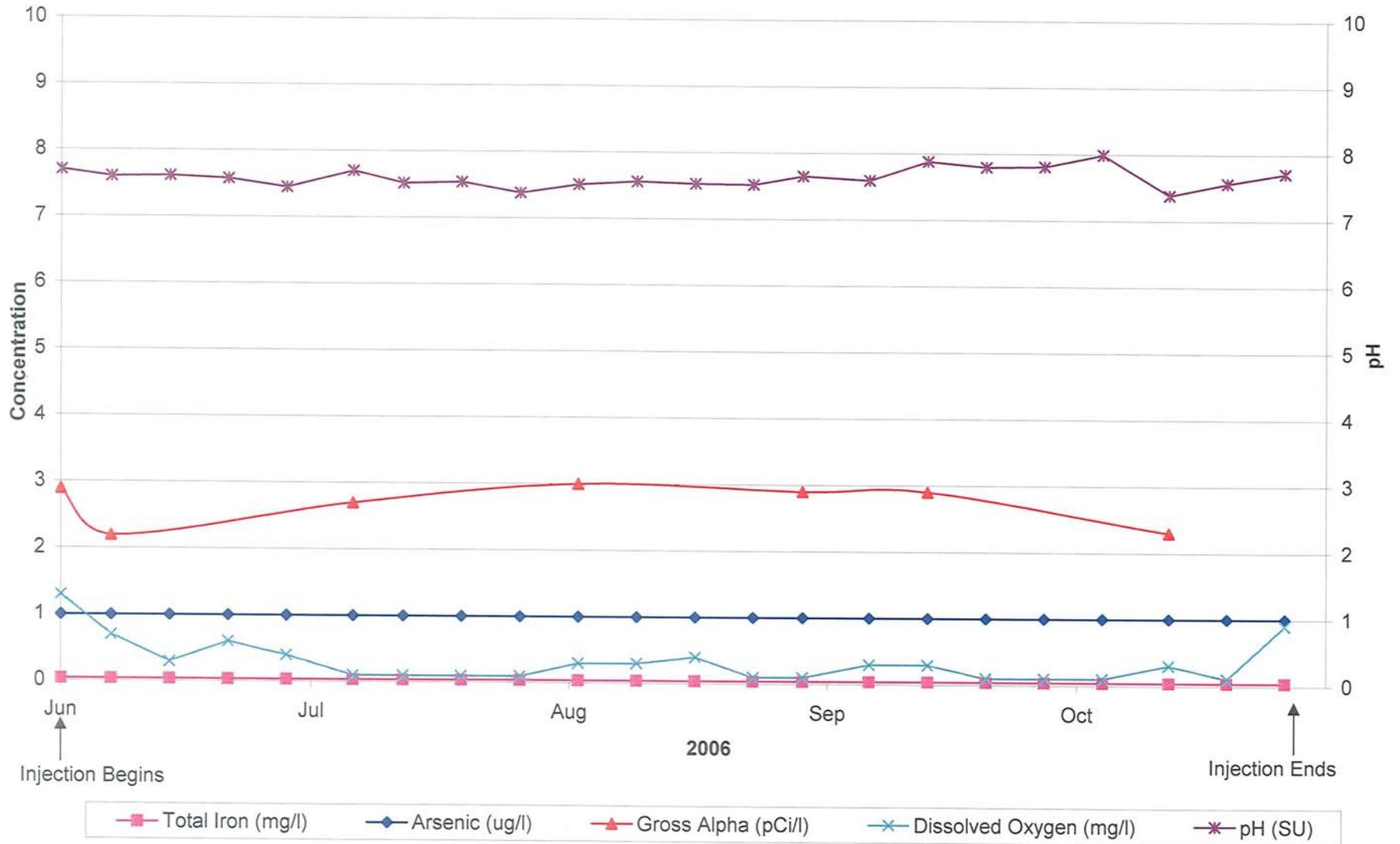
FIGURE 4-15. PLOT OF WATER QUALITY IN STORAGE ZONE OBSERVATION WELL 3 DURING CYCLE 6 (PART 1)
