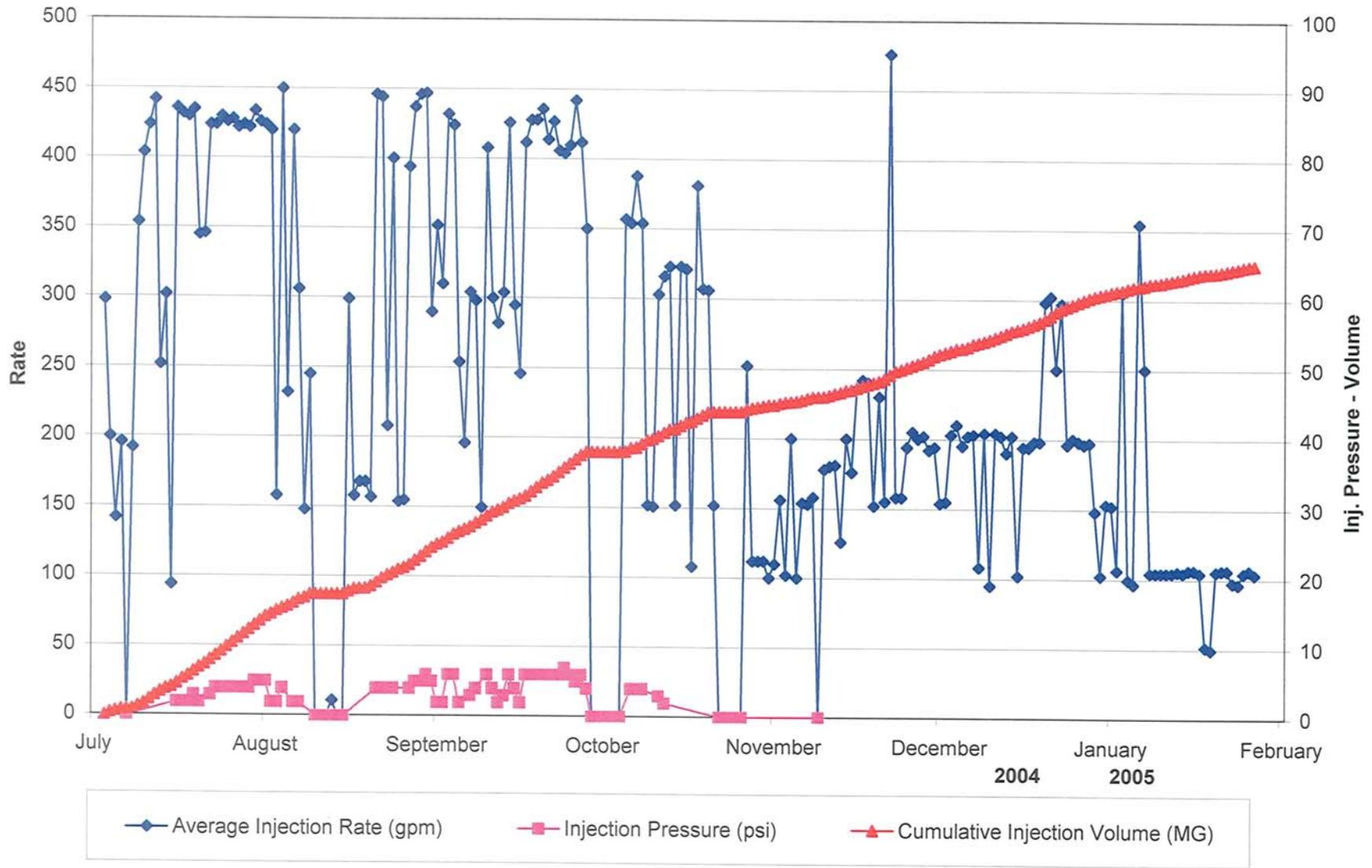
FIGURE 2-6. PLOT OF INJECTION PRESSURE, RATE, AND CUMULATIVE VOLUME INJECTED INTO ASR WELL 4 DURING CYCLE 4
