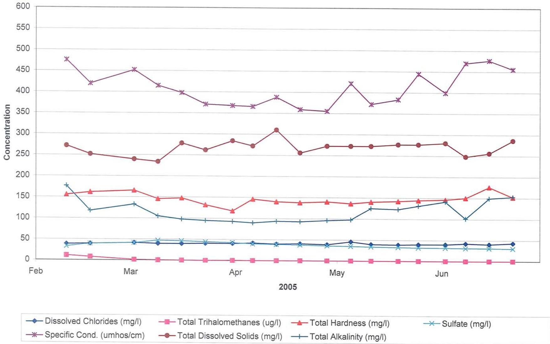
FIGURE 2-24. PLOT OF RECOVERED WATER QUALITY FROM WELL ASR-5 DURING CYCLE 4 (PART 2)
