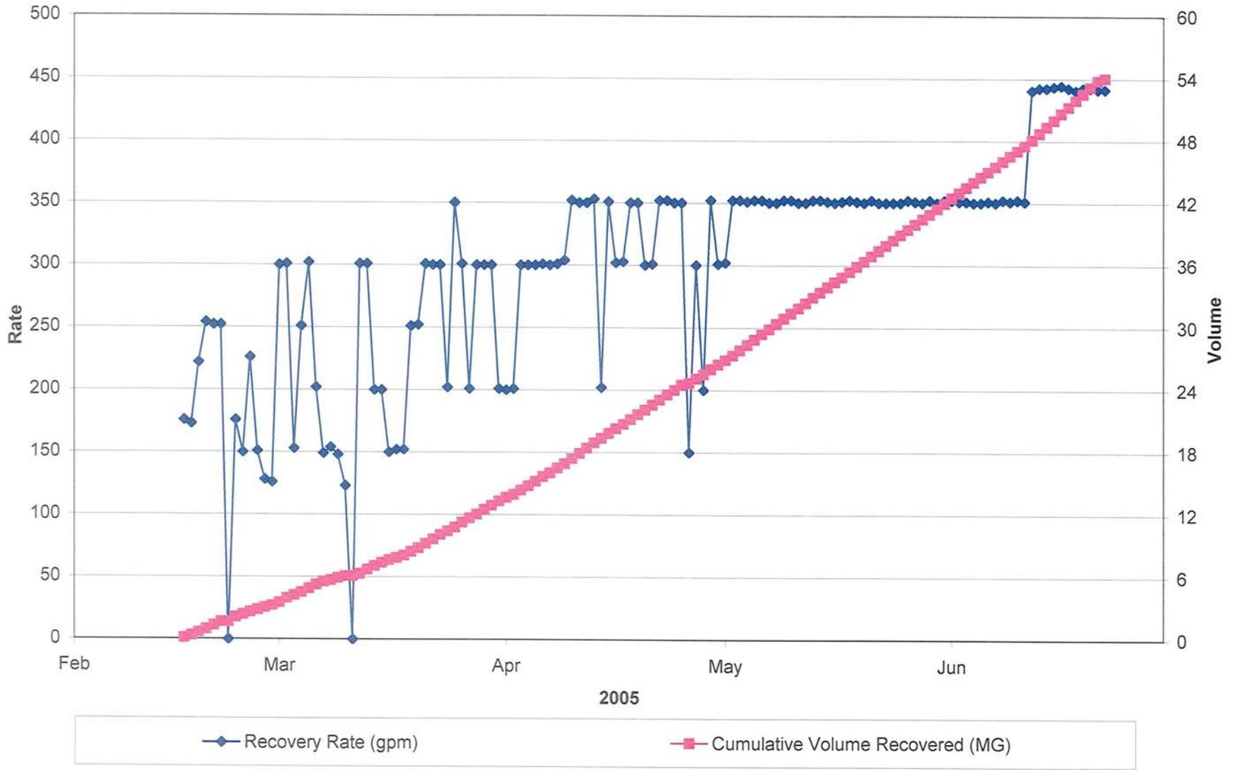
FIGURE 2-31. PLOT OF RECOVERY RATE AND CUMULATIVE VOLUME RECOVERED FOR ASR WELL 5 DURING CYCLE 4
