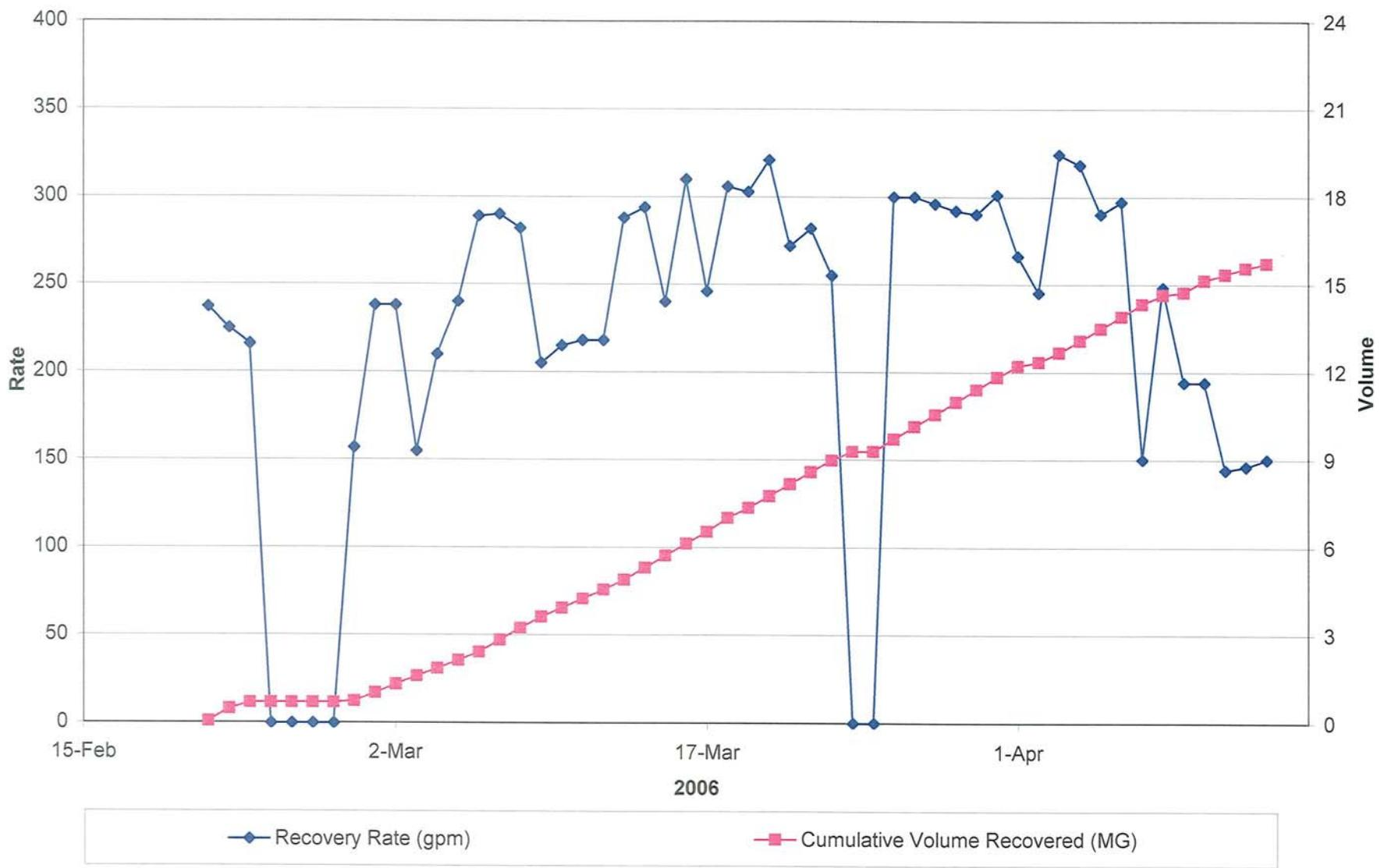
FIGURE 3-31. PLOT OF RECOVERY RATE AND CUMULATIVE VOLUME RECOVERED FOR ASR WELL 3 DURING CYCLE 5
