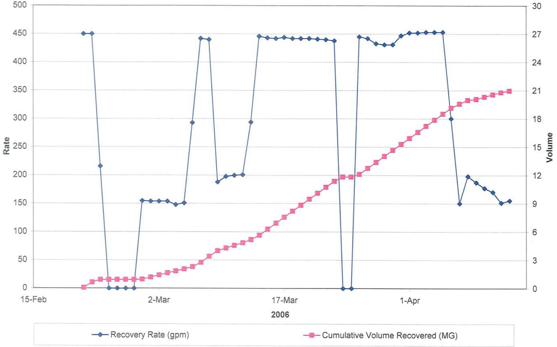
FIGURE 3-32. PLOT OF RECOVERY RATE AND CUMULATIVE VOLUME RECOVERED FOR ASR WELL 4 DURING CYCLE 5
