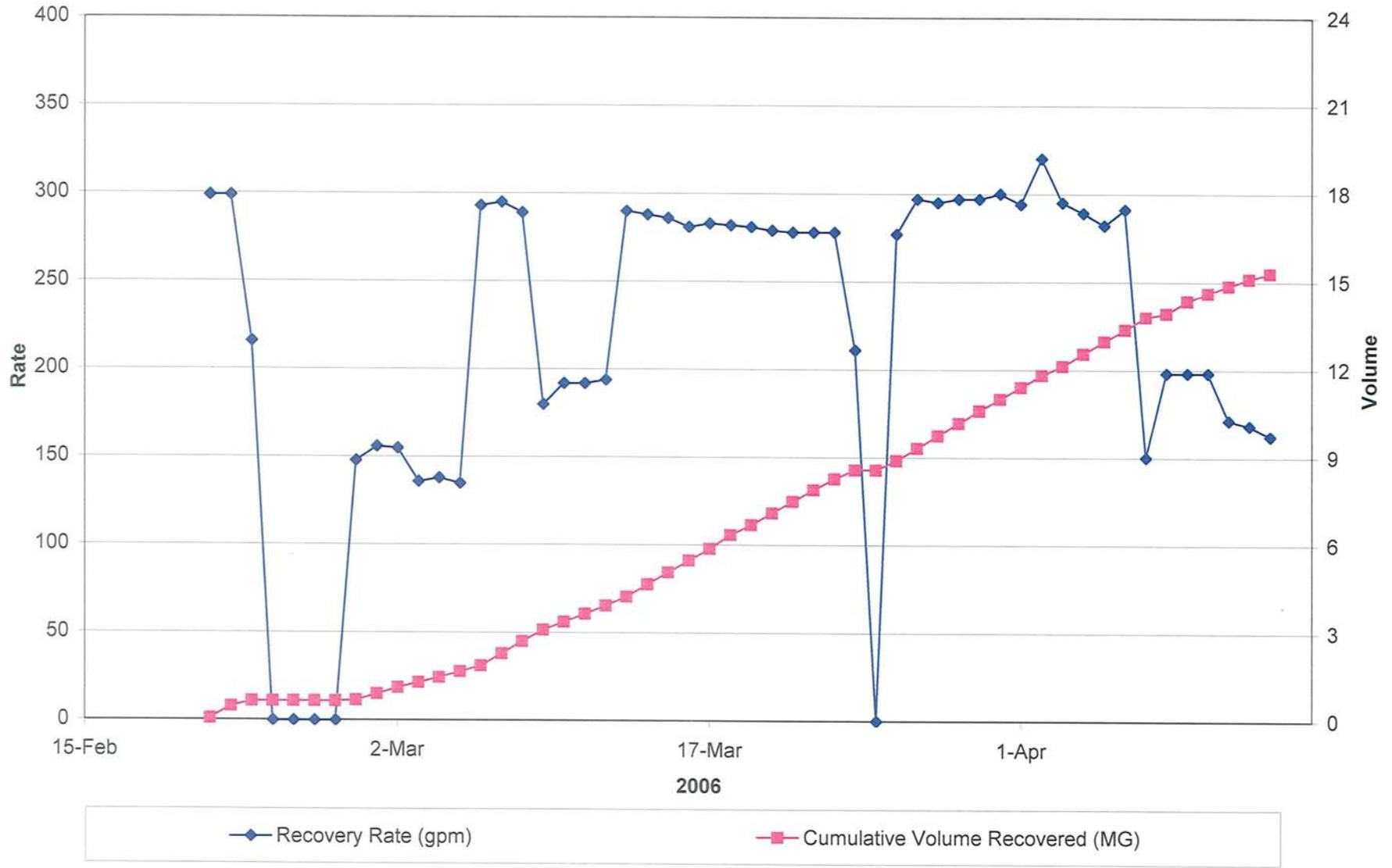
FIGURE 3-30. PLOT OF RECOVERY RATE AND CUMULATIVE VOLUME RECOVERED FOR ASR WELL 2 DURING CYCLE 5
