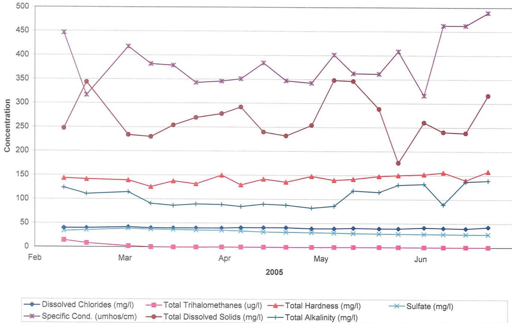
FIGURE 2-16. PLOT OF RECOVERED WATER QUALITY FROM WELL ASR-1 DURING CYCLE 4 (PART 2)
