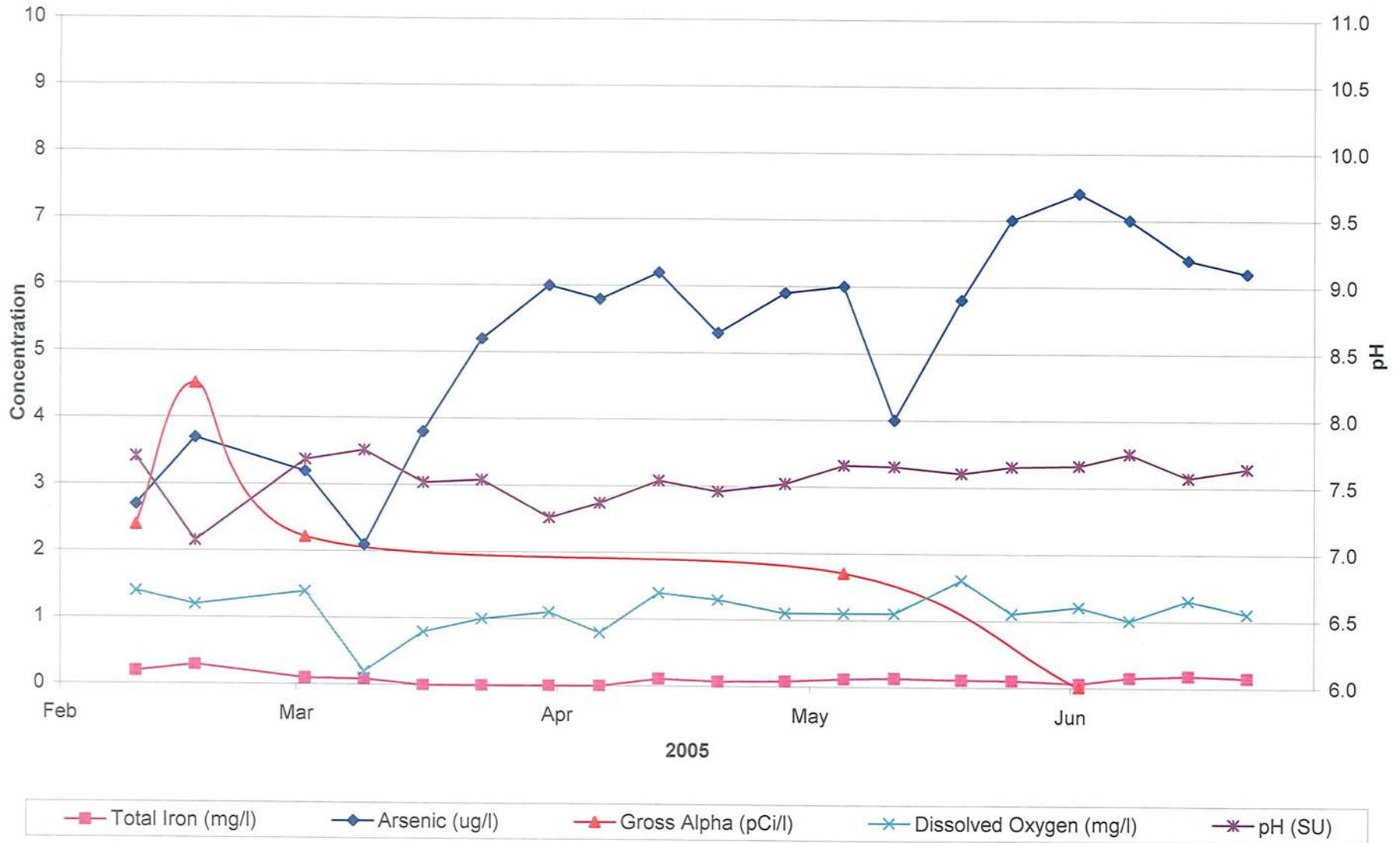
FIGURE 2-23. PLOT OF RECOVERED WATER QUALITY FROM WELL ASR-5 DURING CYCLE 4 (PART 1)
