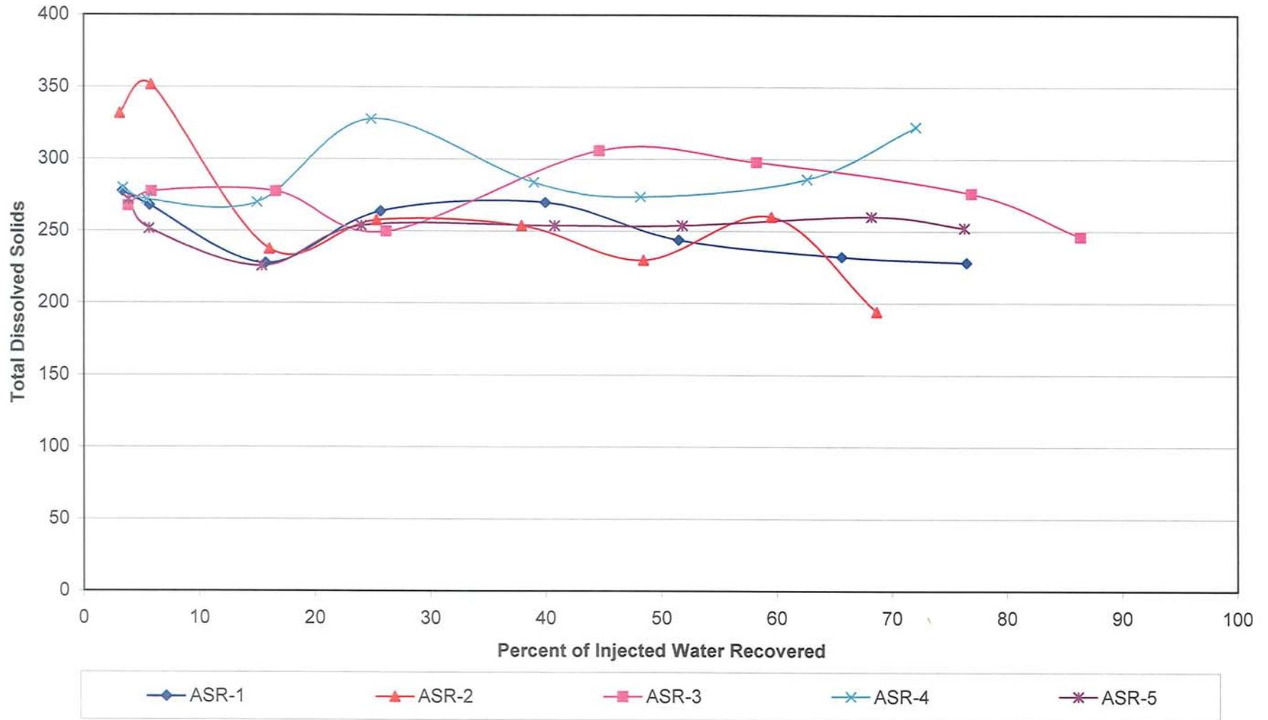
FIGURE 3-28. PLOT OF TOTAL DISSOLVED SOLIDS VERSUS VOLUME OF INJECTED WATER RECOVERED FOR THE ASR WELLS FOR CYCLE 5
