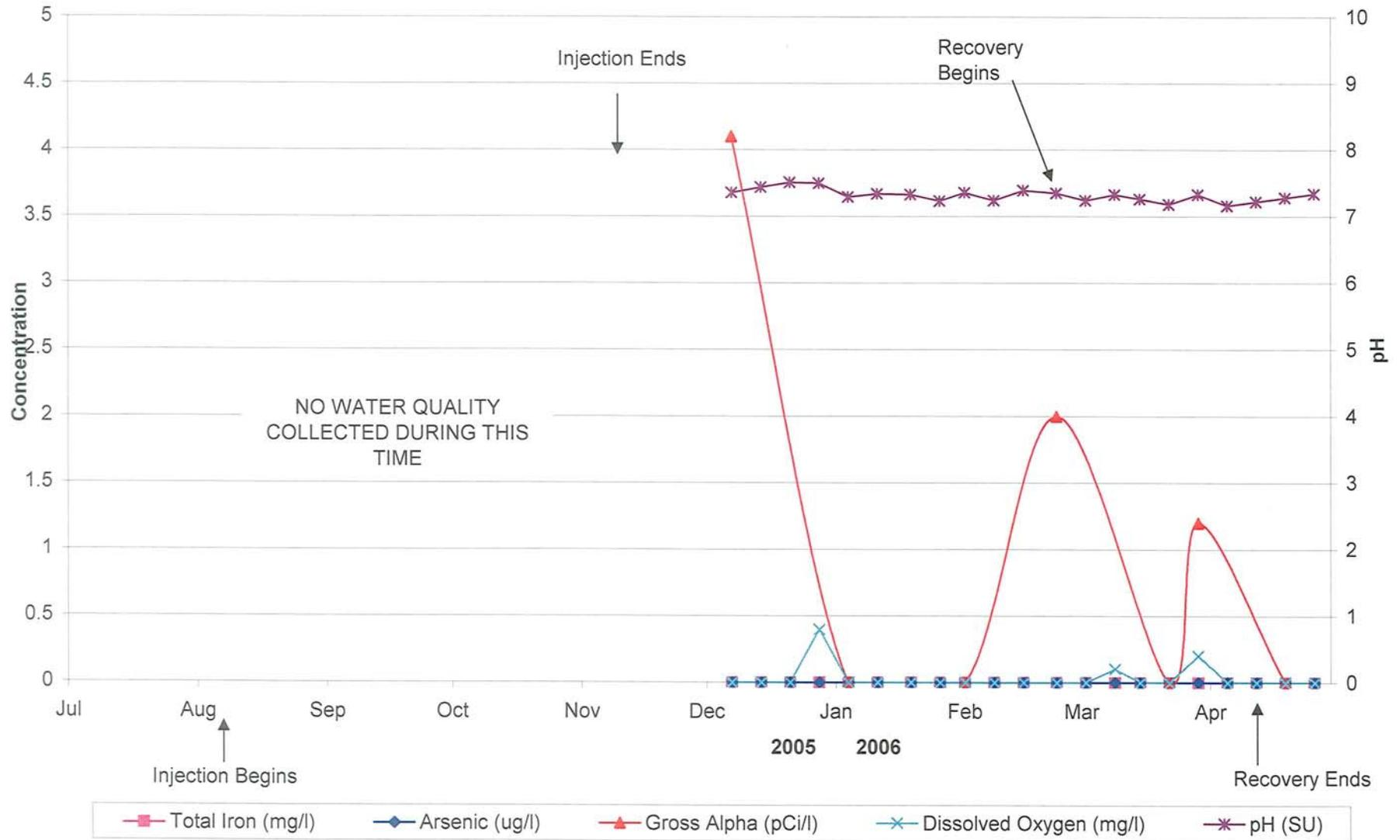
**FIGURE 3-13. PLOT OF WATER QUALITY IN STORAGE ZONE OBSERVATION WELL 2 DURING CYCLE 5 (PART 1)**
