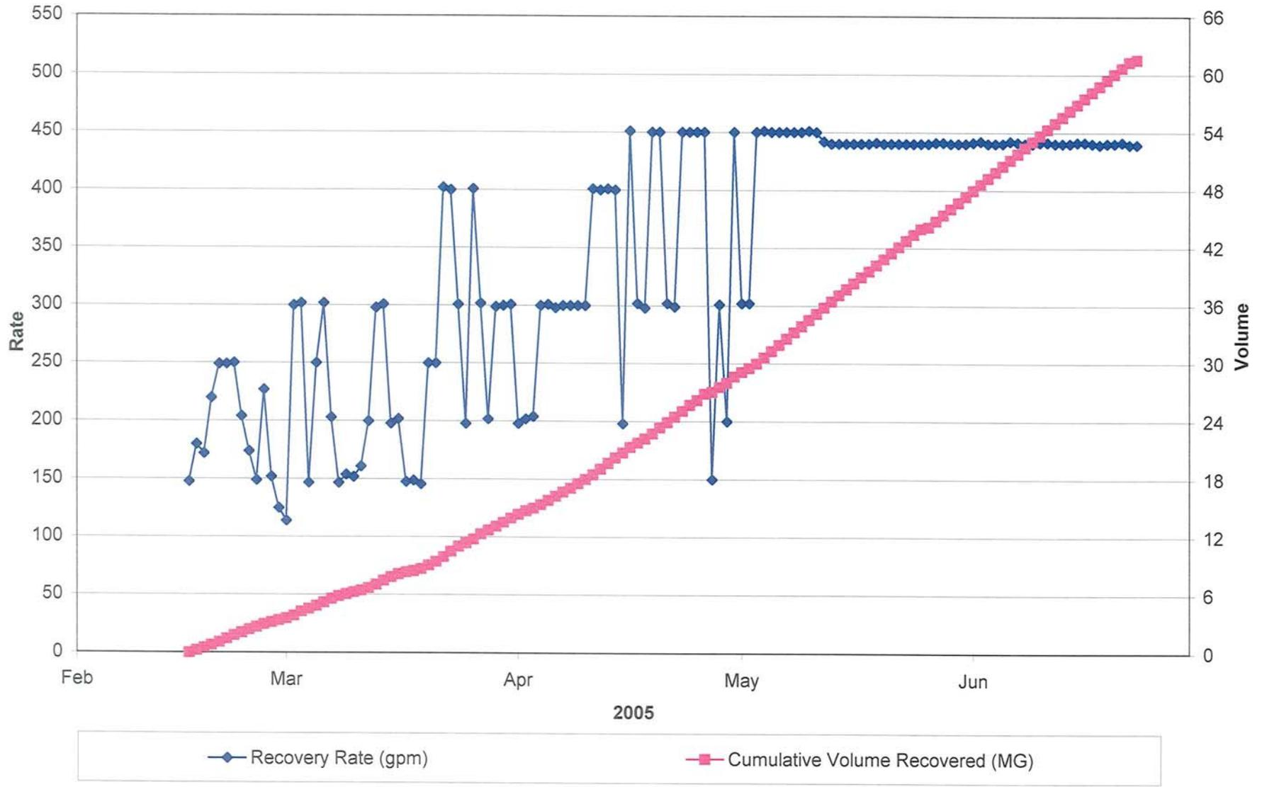
FIGURE 2-30. PLOT OF RECOVERY RATE AND CUMULATIVE VOLUME RECOVERED FOR ASR WELL 4 DURING CYCLE 4
