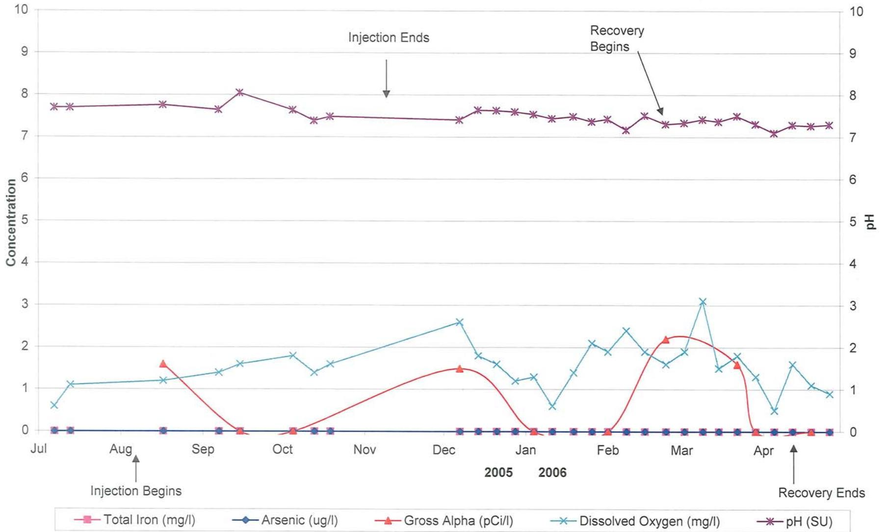
**FIGURE 3-11. PLOT OF WATER QUALITY IN STORAGE ZONE OBSERVATION WELL 1 DURING CYCLE 5 (PART 1)**
