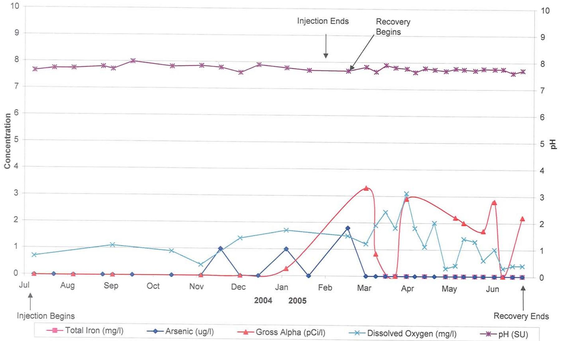
**FIGURE 2-11. PLOT OF WATER QUALITY IN STORAGE ZONE OBSERVATION WELL 2 DURING CYCLE 4 (PART 1)**
