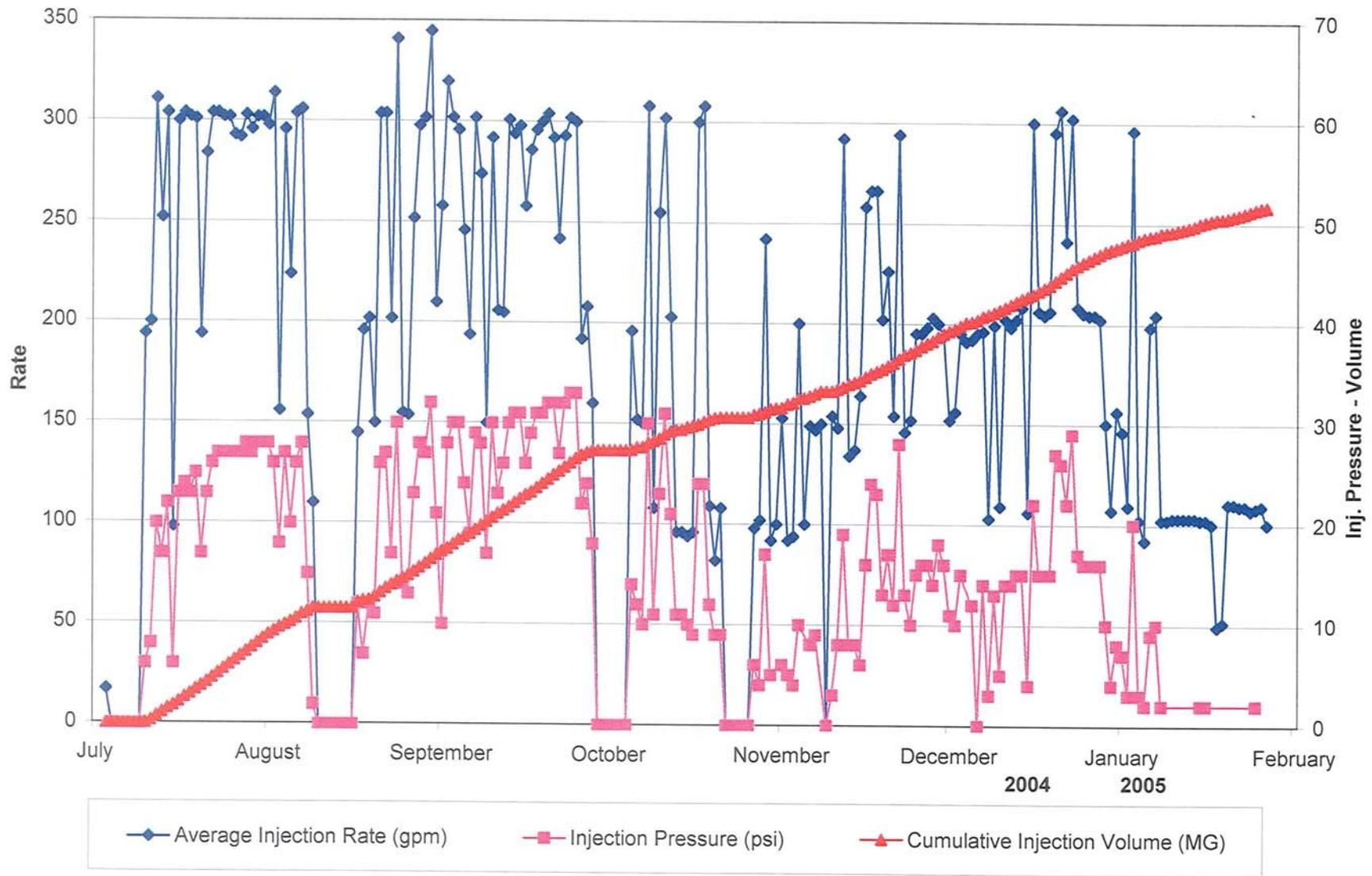
FIGURE 2-5. PLOT OF INJECTION PRESSURE, RATE, AND CUMULATIVE VOLUME INJECTED INTO ASR WELL 3 DURING CYCLE 4
