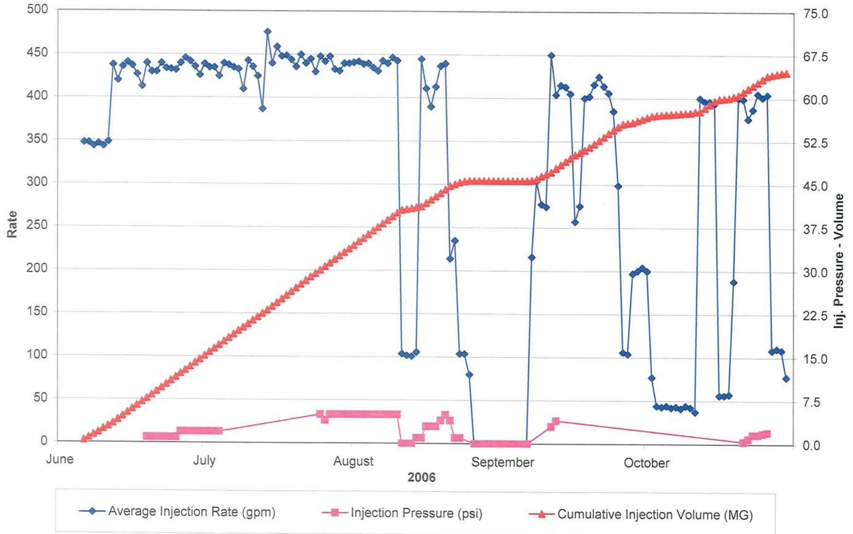
FIGURE 4-7. PLOT OF INJECTION PRESSURE, RATE, AND CUMULATIVE VOLUME INJECTED INTO ASR WELL 5 DURING CYCLE 6
