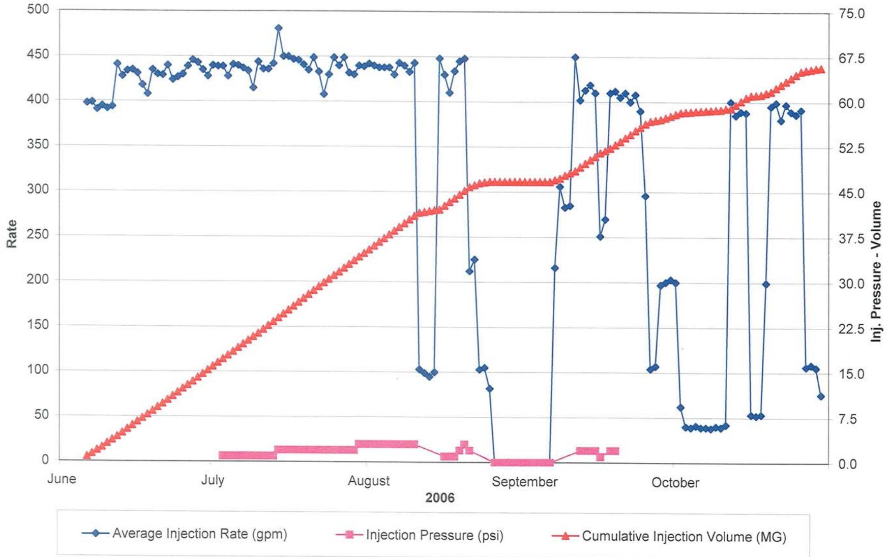
FIGURE 4-6. PLOT OF INJECTION PRESSURE, RATE, AND CUMULATIVE VOLUME INJECTED INTO ASR WELL 4 DURING CYCLE 6
