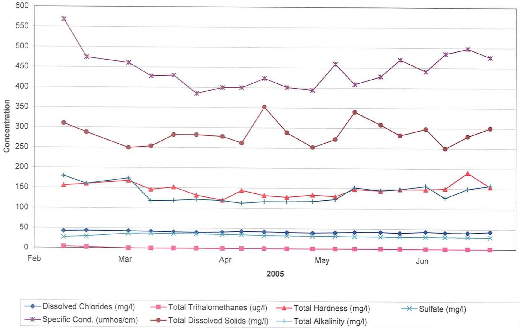
FIGURE 2-22. PLOT OF RECOVERED WATER QUALITY FROM WELL ASR-4 DURING CYCLE 4 (PART 2)
