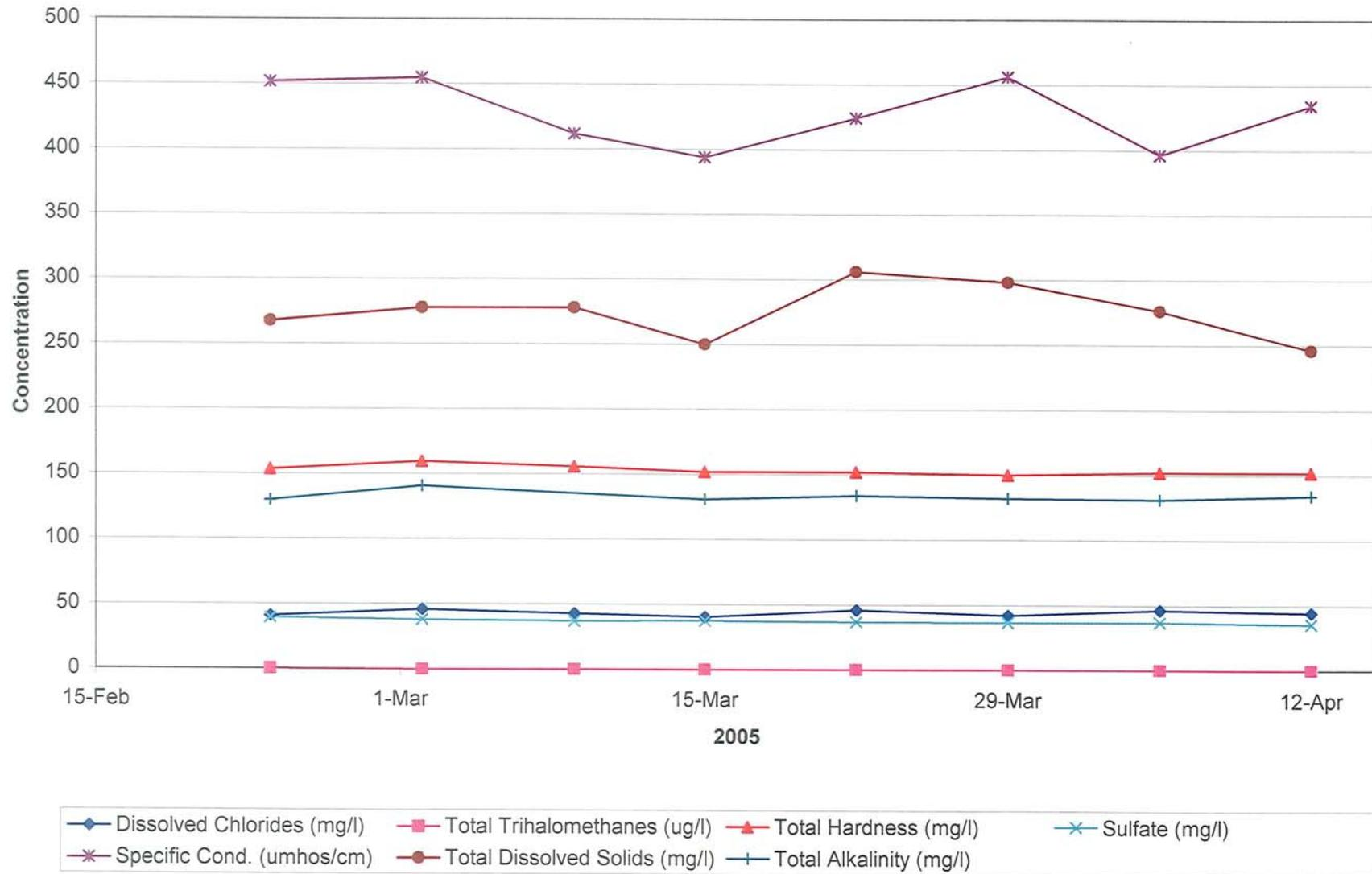
FIGURE 3-22. PLOT OF RECOVERED WATER QUALITY FROM WELL ASR-3 DURING CYCLE 5 (PART 2)
