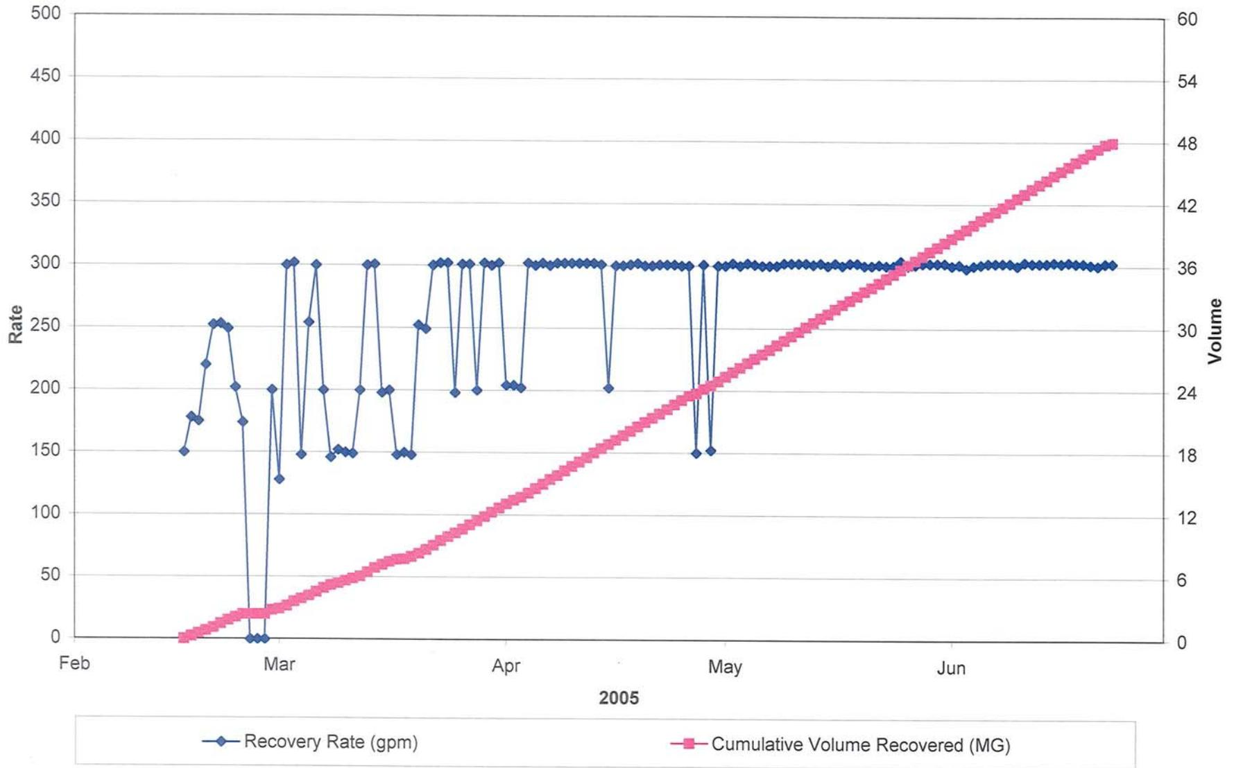
FIGURE 2-29. PLOT OF RECOVERY RATE AND CUMULATIVE VOLUME RECOVERED FOR ASR WELL 3 DURING CYCLE 4
