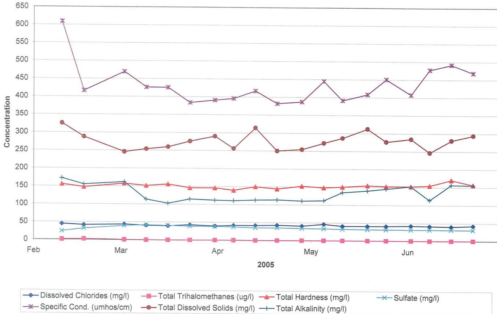
FIGURE 2-20. PLOT OF RECOVERED WATER QUALITY FROM WELL ASR-3 DURING CYCLE 4 (PART 2)
