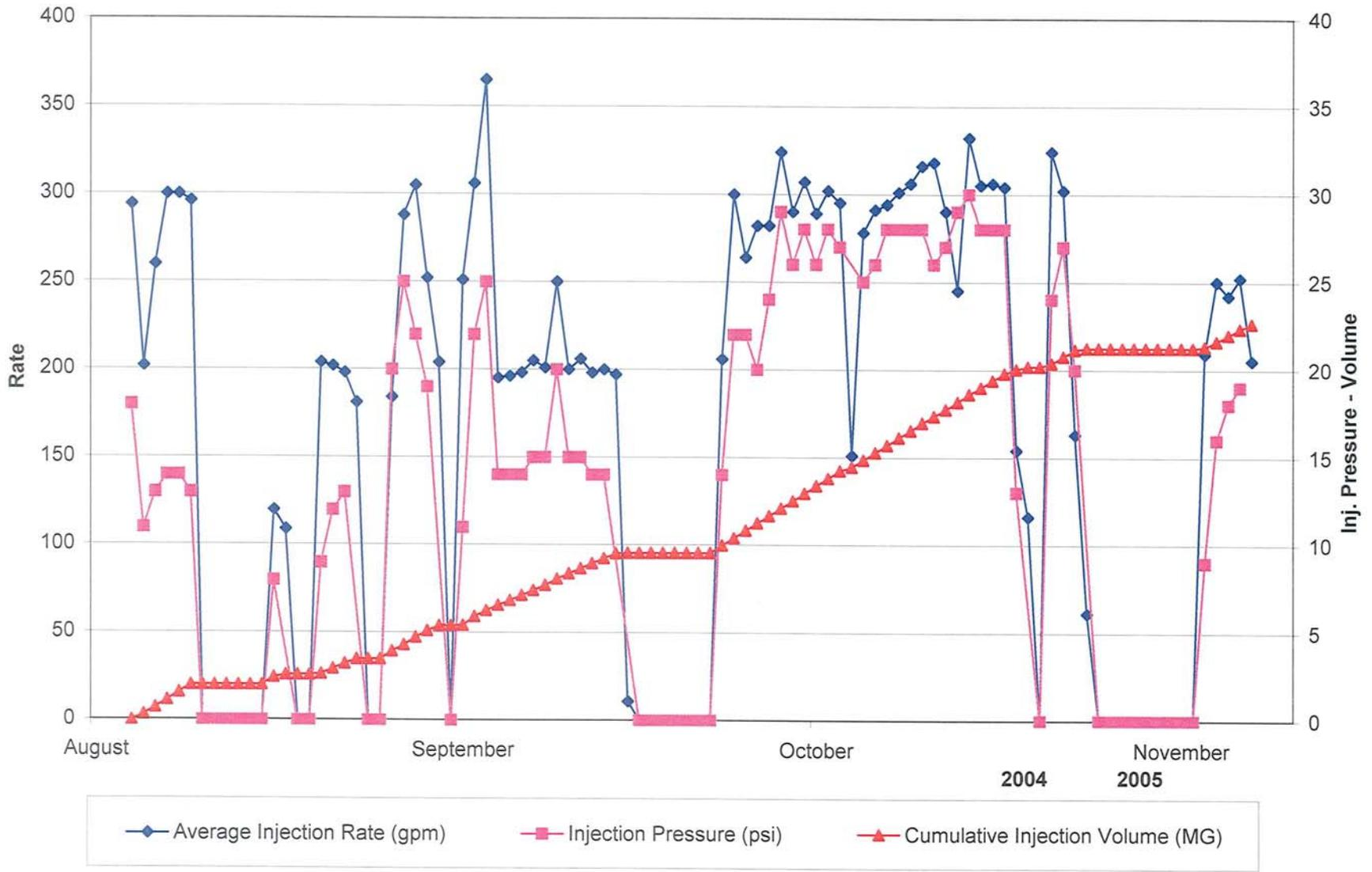
**FIGURE 3-5. PLOT OF INJECTION PRESSURE, RATE, AND CUMULATIVE VOLUME INJECTED INTO ASR WELL 3 DURING CYCLE 5**
