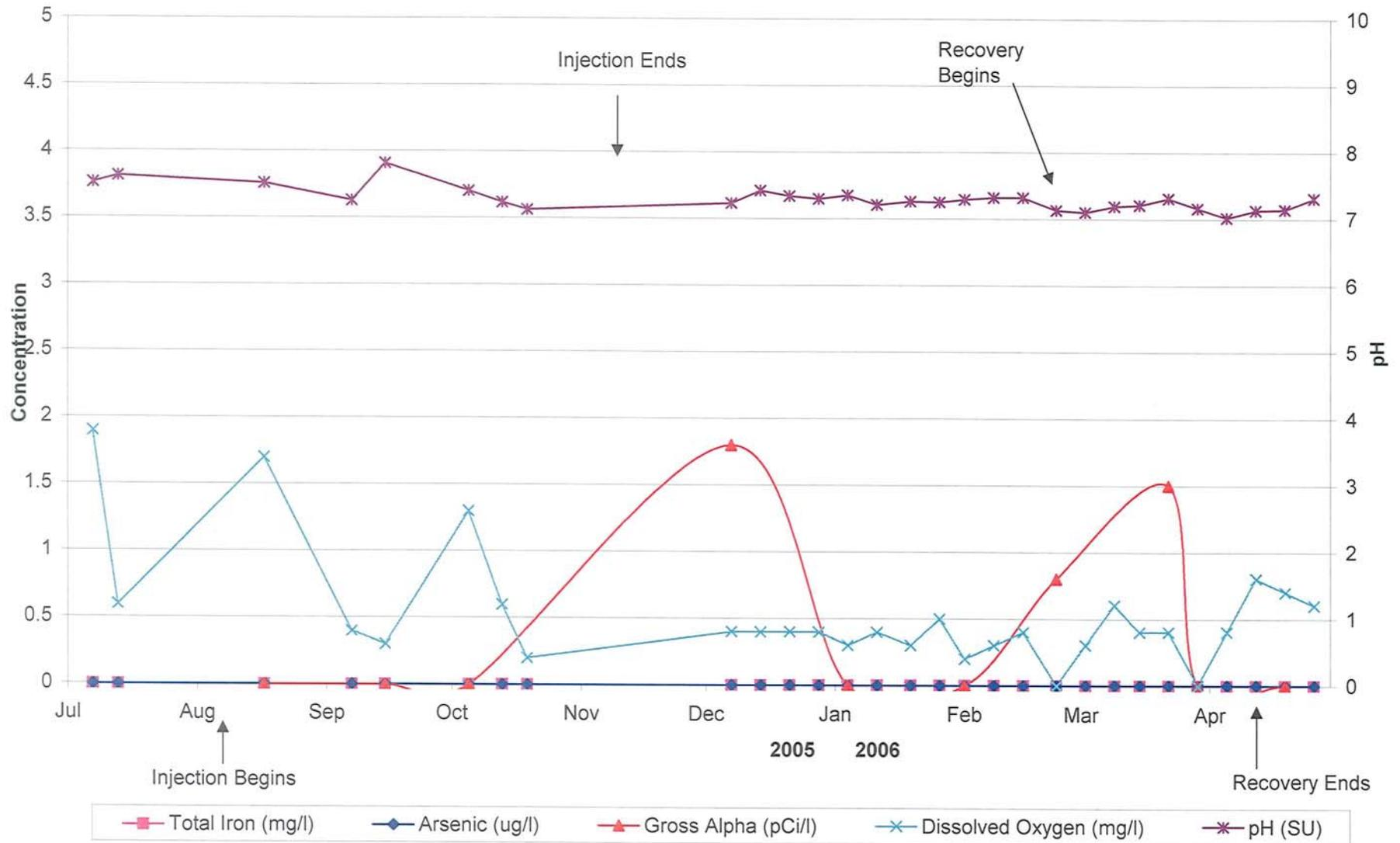
**FIGURE 3-15. PLOT OF WATER QUALITY IN STORAGE ZONE OBSERVATION WELL 3 DURING CYCLE 5 (PART 1)**
