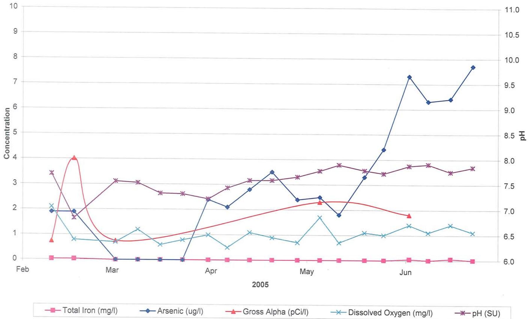
FIGURE 2-19. PLOT OF RECOVERED WATER QUALITY FROM WELL ASR-3 DURING CYCLE 4 (PART 1)
