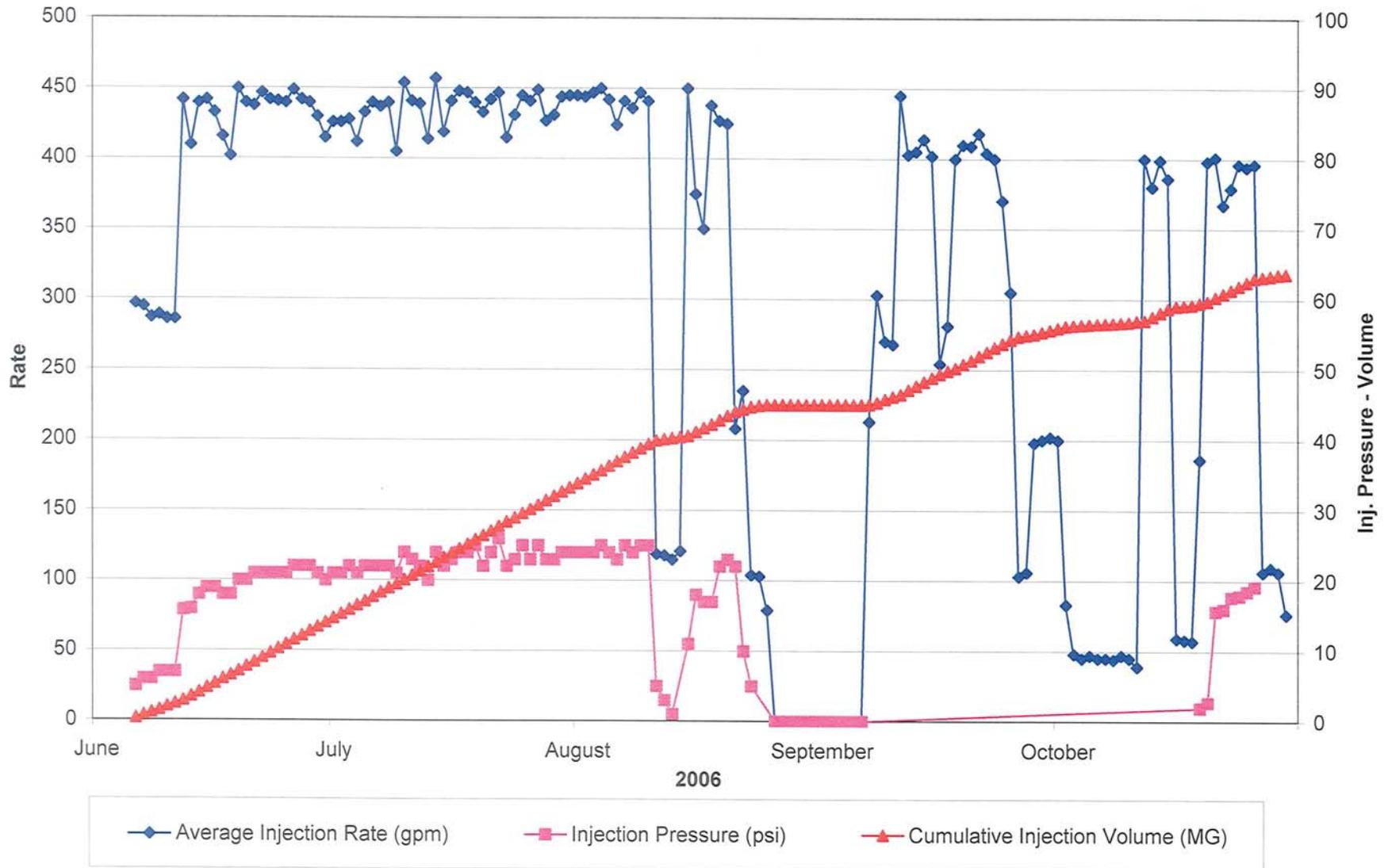
**FIGURE 4-4. PLOT OF INJECTION PRESSURE, RATE, AND CUMULATIVE VOLUME INJECTED INTO ASR WELL 2 DURING CYCLE 6**
