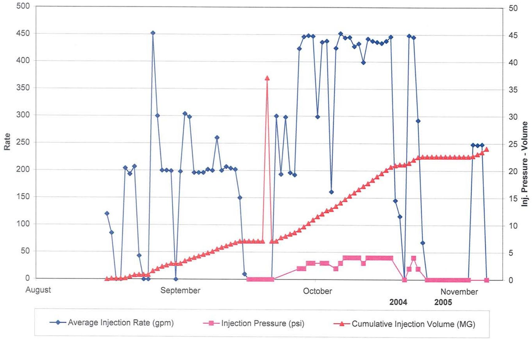
**FIGURE 3-6. PLOT OF INJECTION PRESSURE, RATE, AND CUMULATIVE VOLUME INJECTED INTO ASR WELL 4 DURING CYCLE 5**
