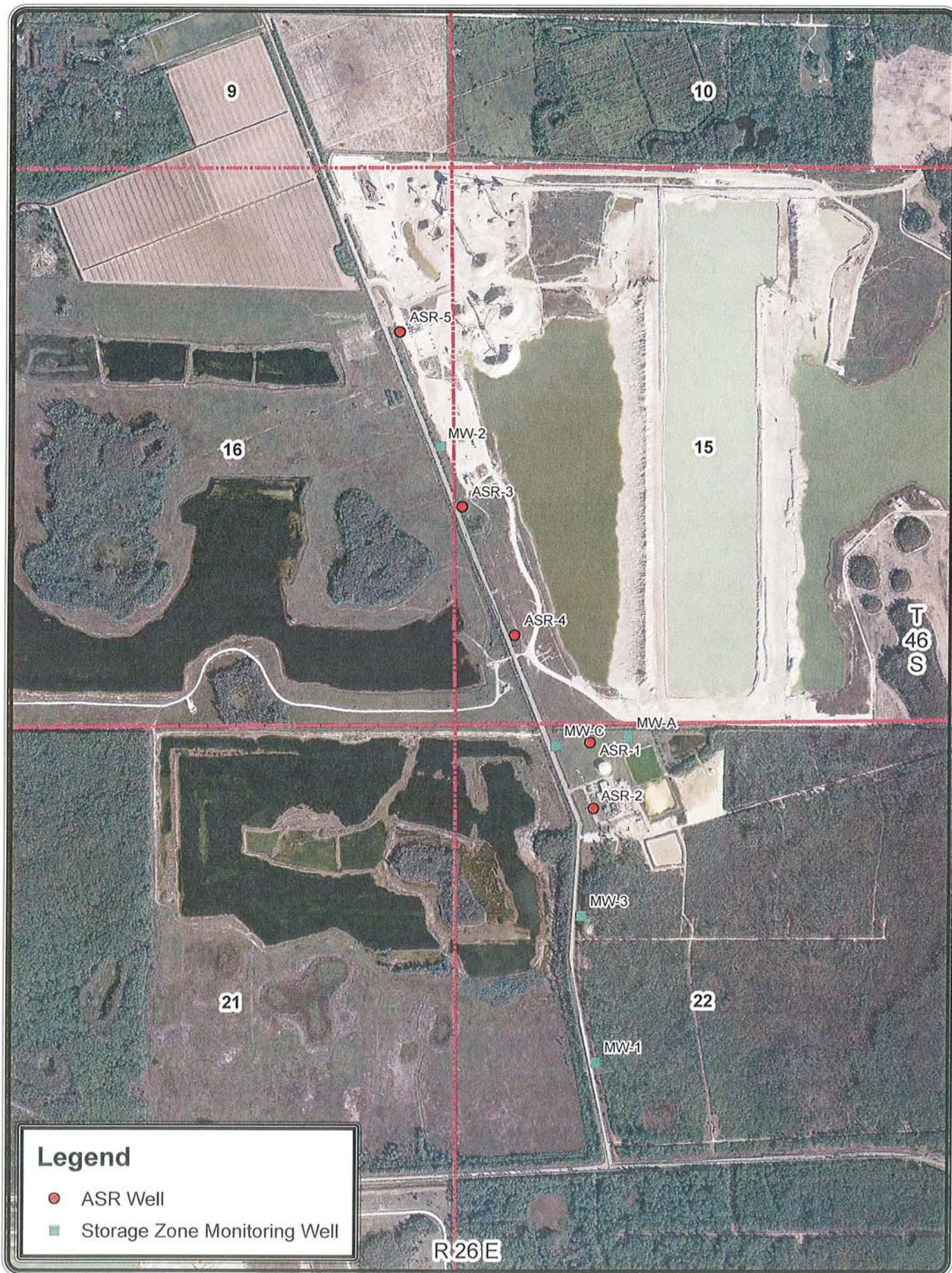
FIGURE 1-2. AERIAL PHOTO SHIOWING LOCATIONS OF ASR AND STORAGE ZONE MONITORING WELLS.
