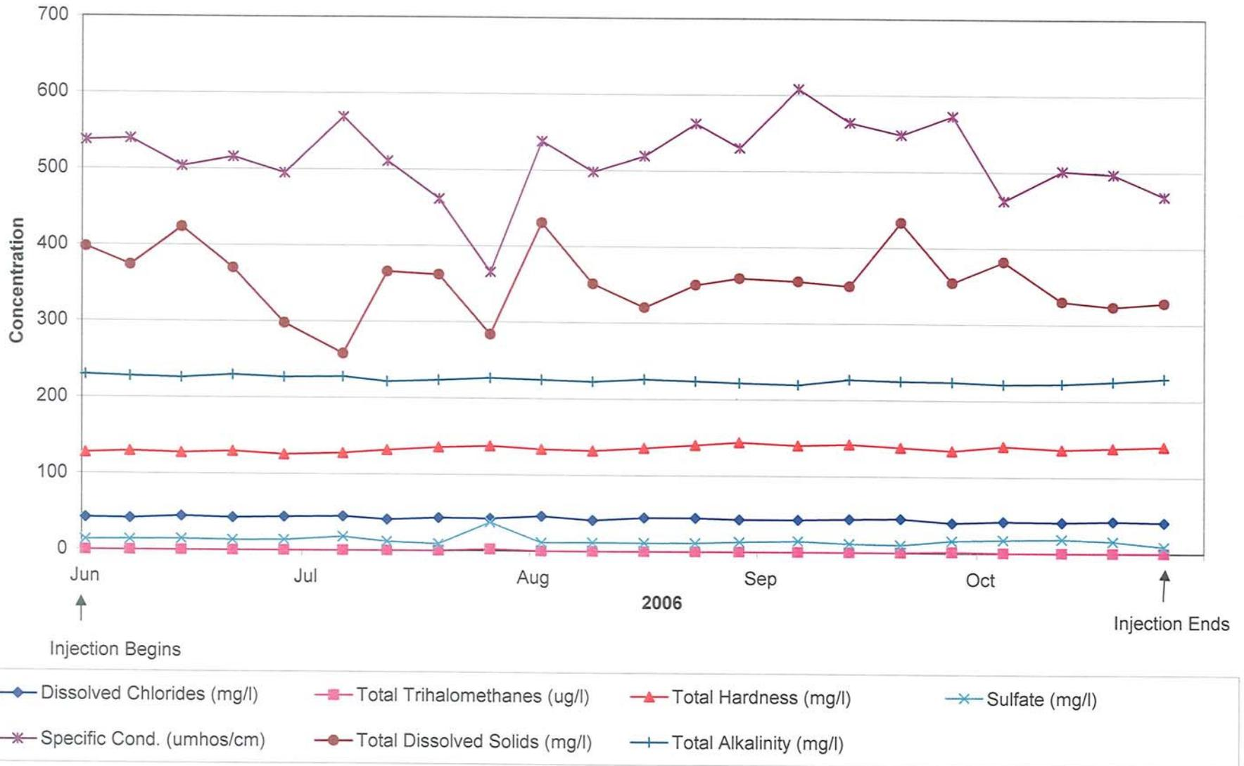
FIGURE 4-12. PLOT OF WATER QUALITY IN STORAGE ZONE OBSERVATION WELL 1 DURING CYCLE 6 (PART 2)
