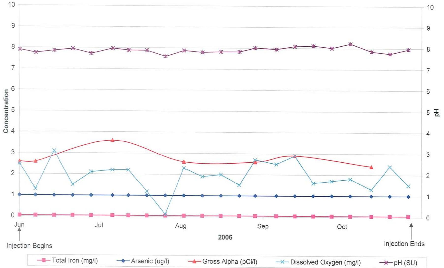
FIGURE 4-11. PLOT OF WATER QUALITY IN STORAGE ZONE OBSERVATION WELL 1 DURING CYCLE 6 (PART 1)
