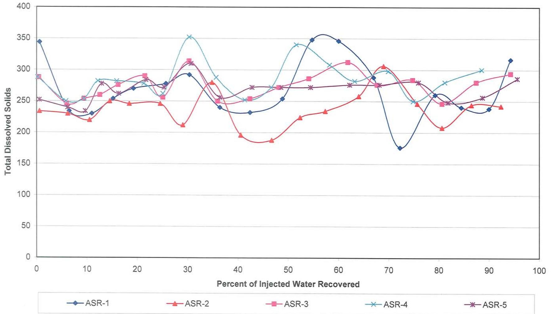
FIGURE 2-26. PLOT OF TOTAL DISSOLVED SOLIDS VERSUS VOLUME OF INJECTED WATER RECOVERED FOR THE ASR WELLS FOR CYCLE 4
