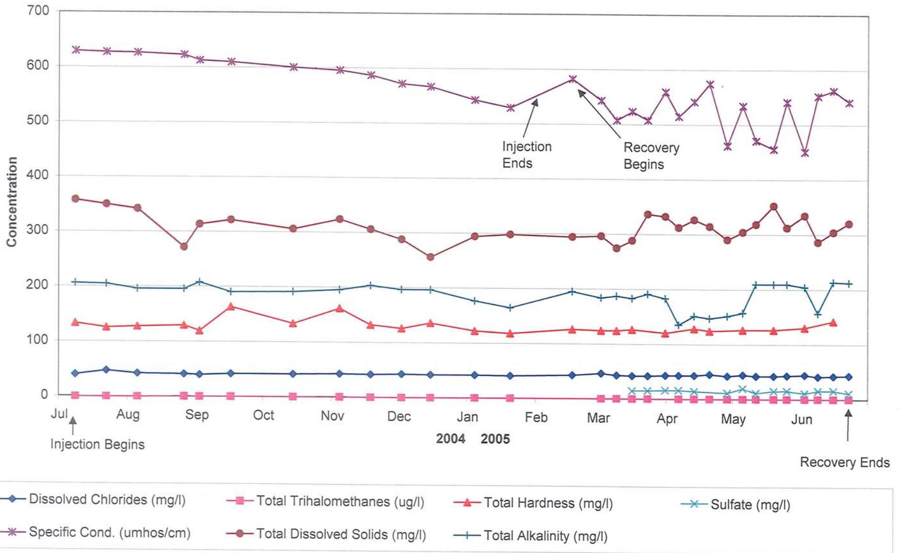
FIGURE 2-14. PLOT OF WATER QUALITY IN STORAGE ZONE OBSERVATION WELL 3 DURING CYCLE 4 (PART 2)
