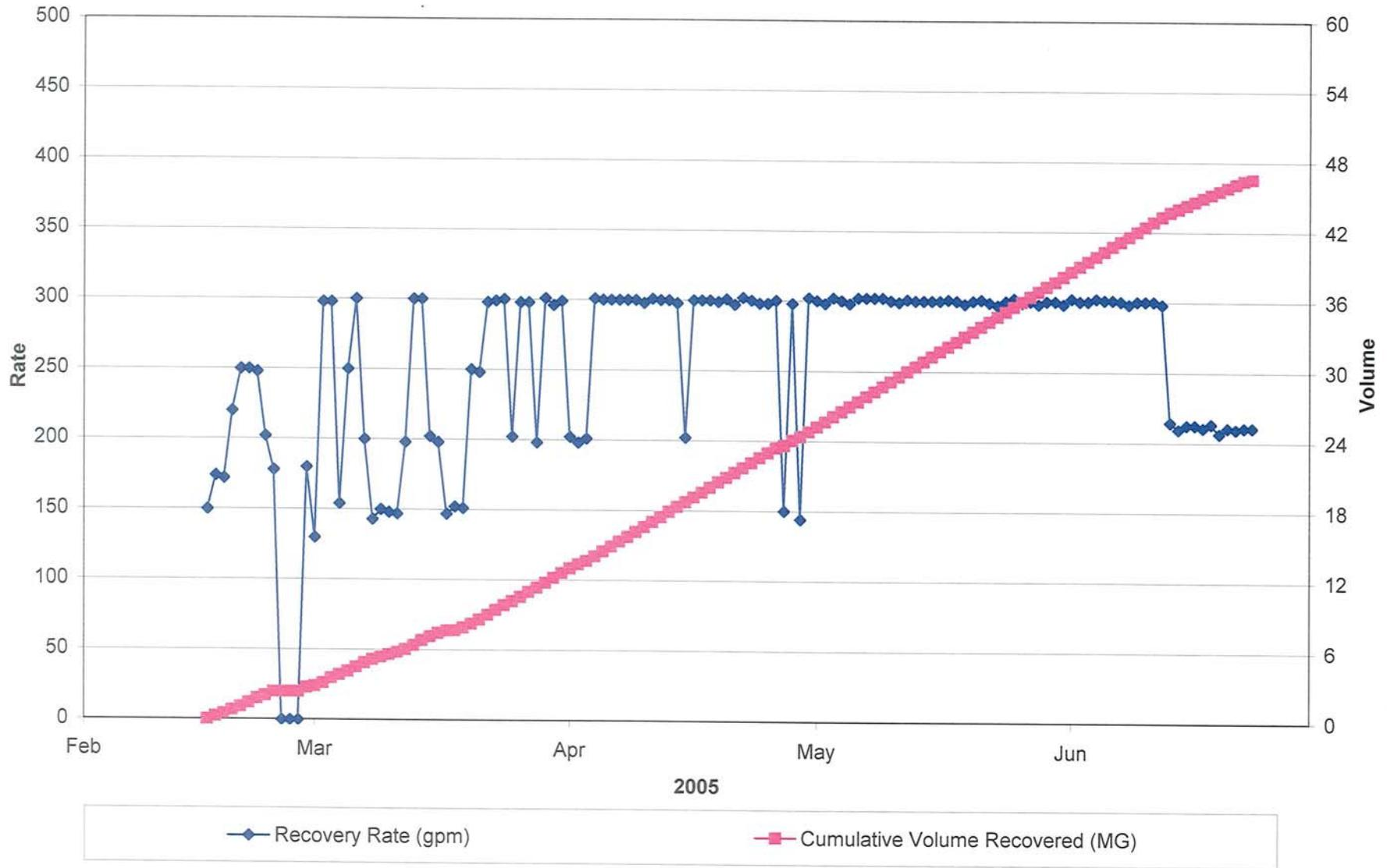
FIGURE 2-28. PLOT OF RECOVERY RATE AND CUMULATIVE VOLUME RECOVERED FOR ASR WELL 2 DURING CYCLE 4
