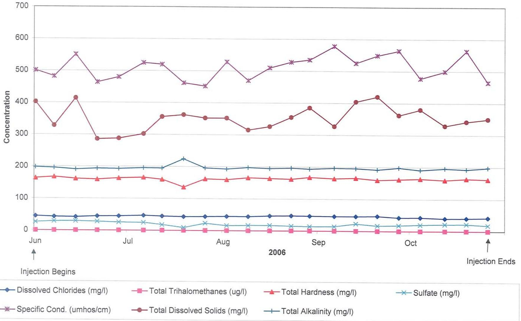
FIGURE 4-14. PLOT OF WATER QUALITY IN STORAGE ZONE OBSERVATION WELL 2 DURING CYCLE 6 (PART 2)
