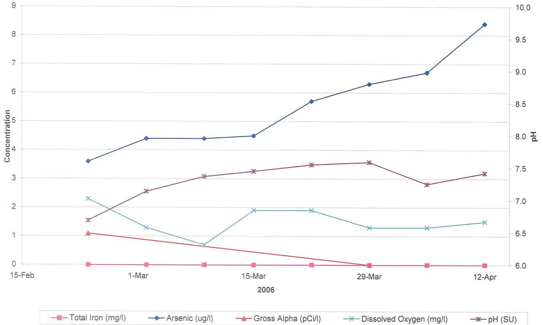
FIGURE 3-19. PLOT OF RECOVERED WATER QUALITY FROM WELL ASR-2 DURING CYCLE 5
