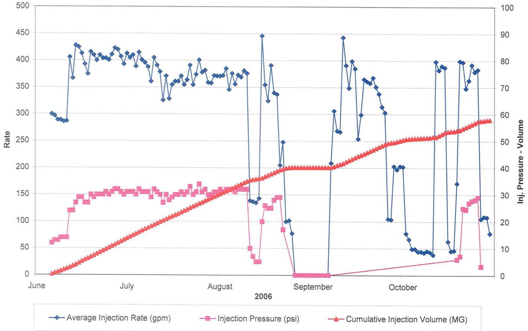
FIGURE 4-5. PLOT OF INJECTION PRESSURE, RATE, AND CUMULATIVE VOLUME INJECTED INTO ASR WELL 3 DURING CYCLE 6
