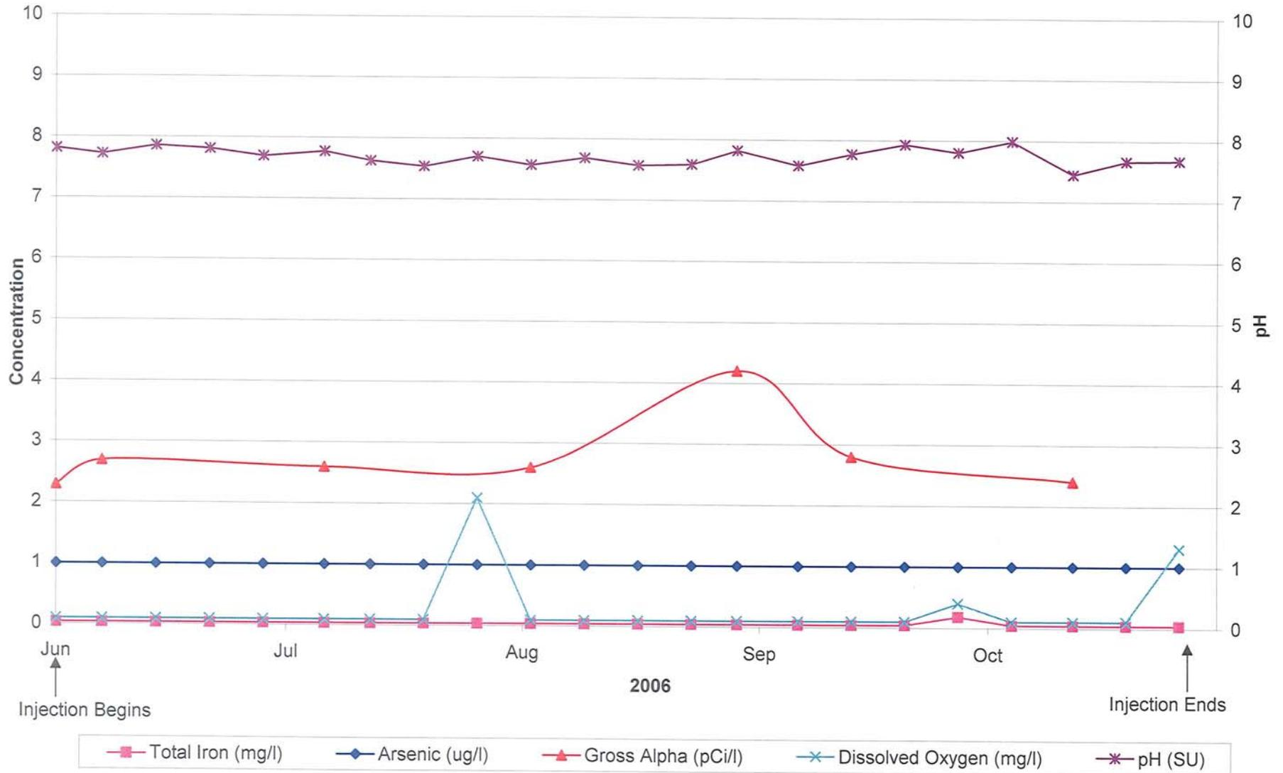
FIGURE 4-13. PLOT OF WATER QUALITY IN STORAGE ZONE OBSERVATION WELL 2 DURING CYCLE 6 (PART 1)
