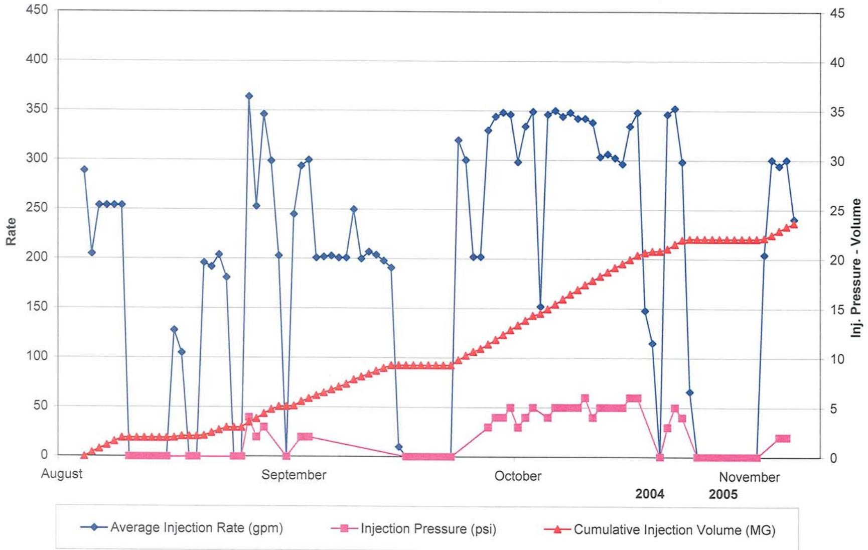
**FIGURE 3-7. PLOT OF INJECTION PRESSURE, RATE, AND CUMULATIVE VOLUME INJECTED INTO ASR WELL 5 DURING CYCLE 5**
