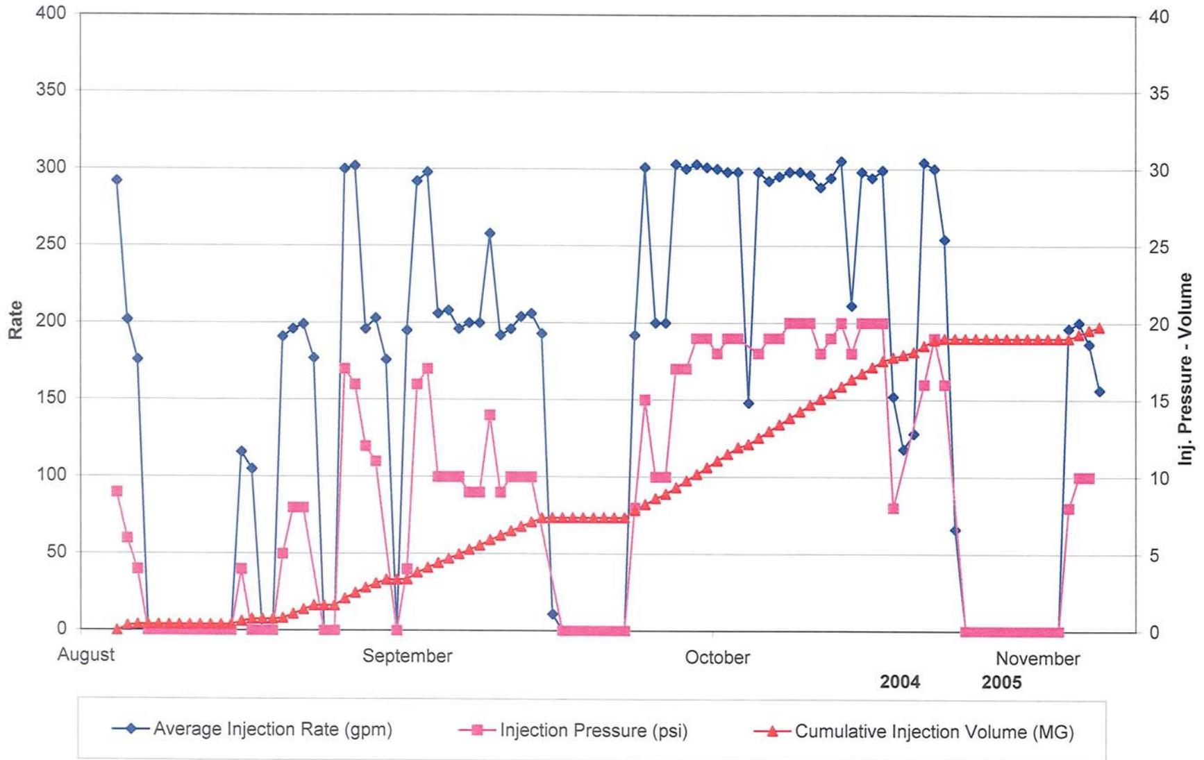
**FIGURE 3-4. PLOT OF INJECTION PRESSURE, RATE, AND CUMULATIVE VOLUME INJECTED INTO ASR WELL 2 DURING CYCLE 5**
