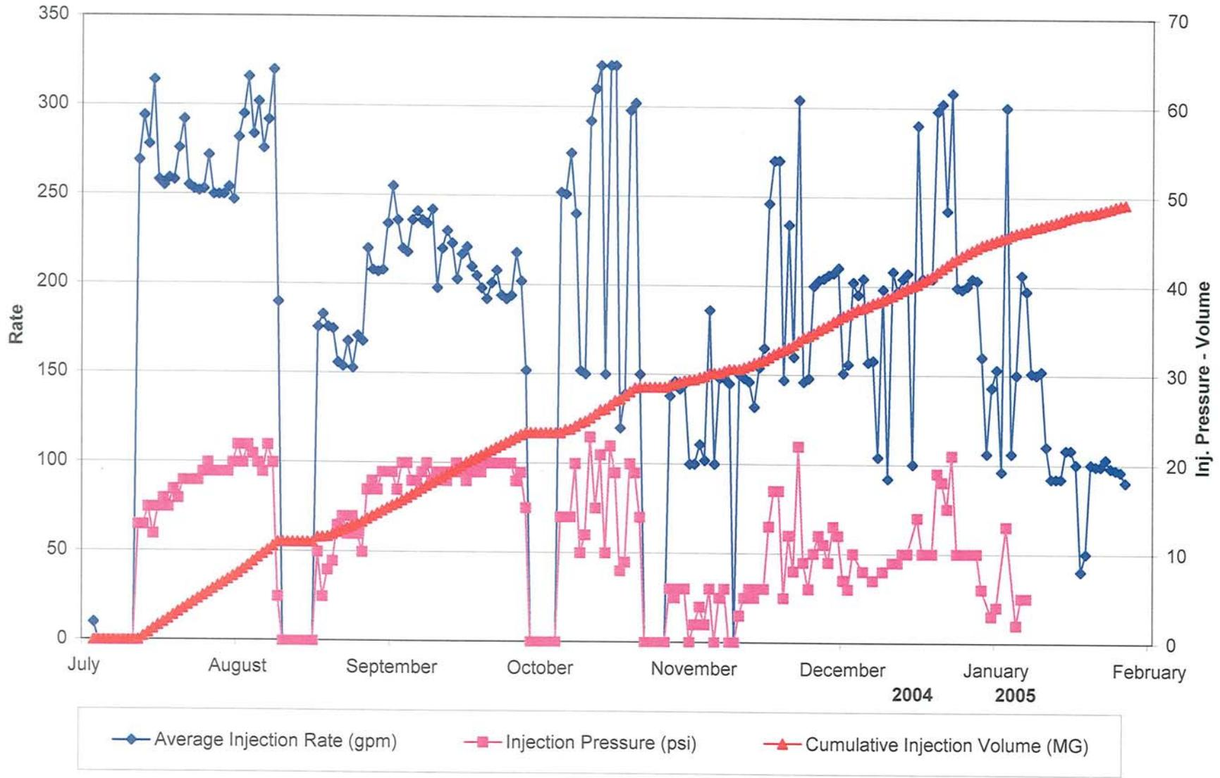
FIGURE 2-4. PLOT OF INJECTION PRESSURE, RATE, AND CUMULATIVE VOLUME INJECTED INTO ASR WELL 2 DURING CYCLE 4
