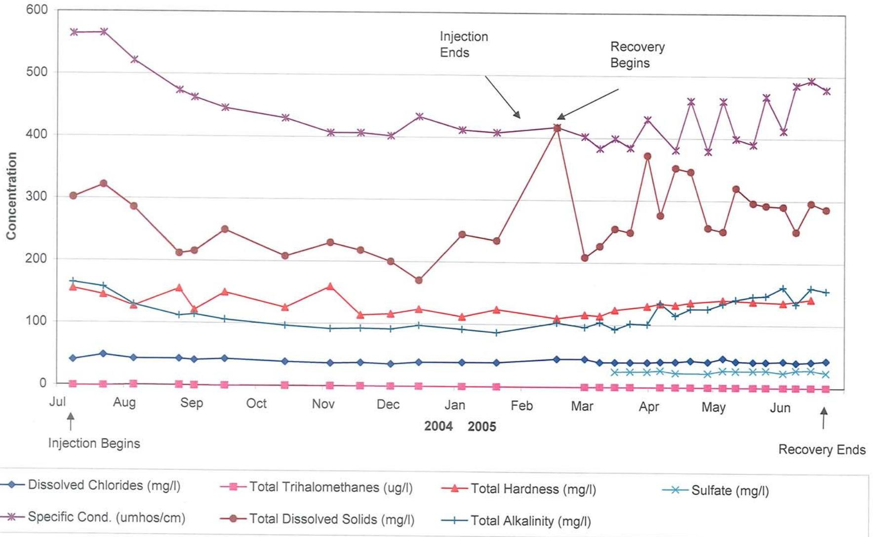
FIGURE 2-10. PLOT OF WATER QUALITY IN STORAGE ZONE OBSERVATION WELL C DURING CYCLE 4 (PART 2)
