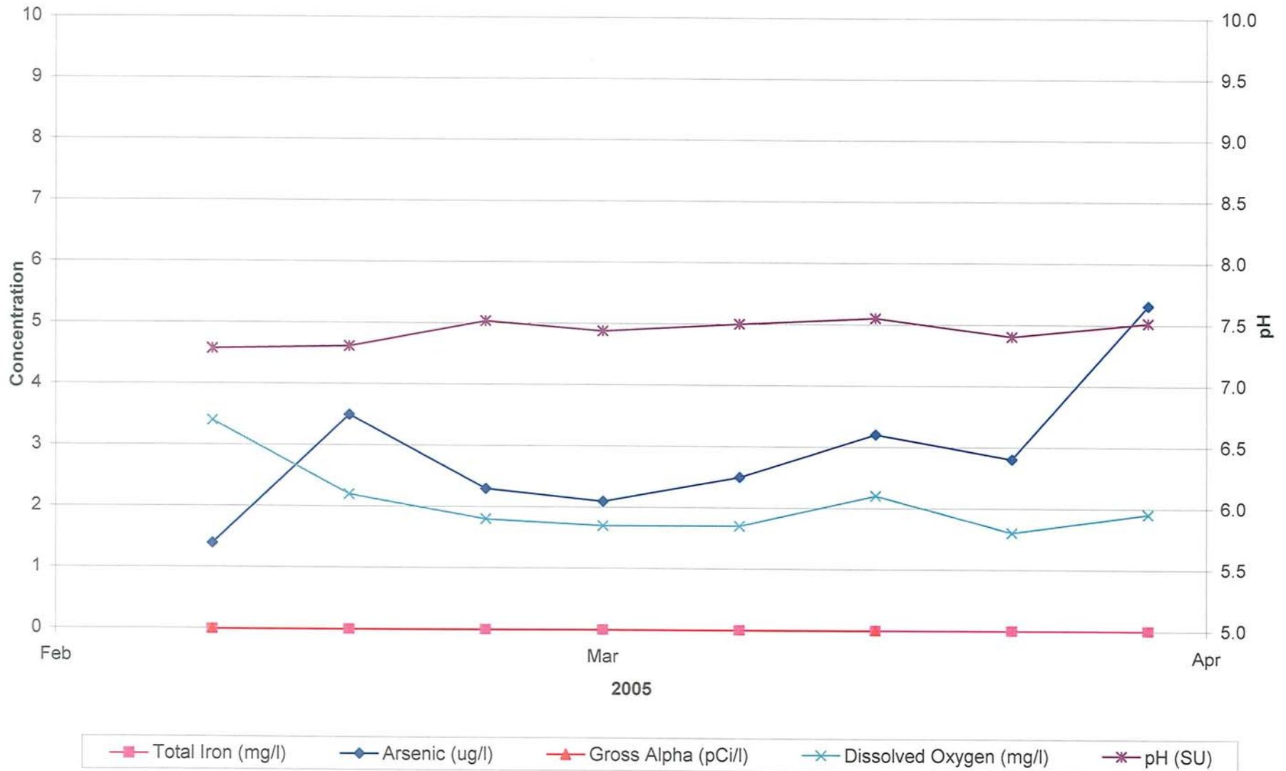
FIGURE 3-21. PLOT OF RECOVERED WATER QUALITY FROM WELL ASR-3 DURING CYCLE 5
