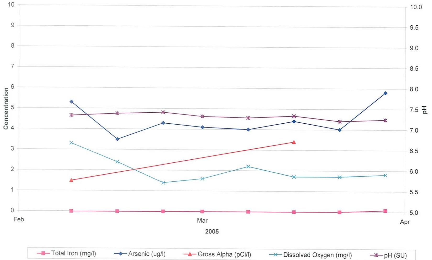
FIGURE 3-23. PLOT OF RECOVERED WATER QUALITY FROM WELL ASR-4 DURING CYCLE 5 (PART 1)
