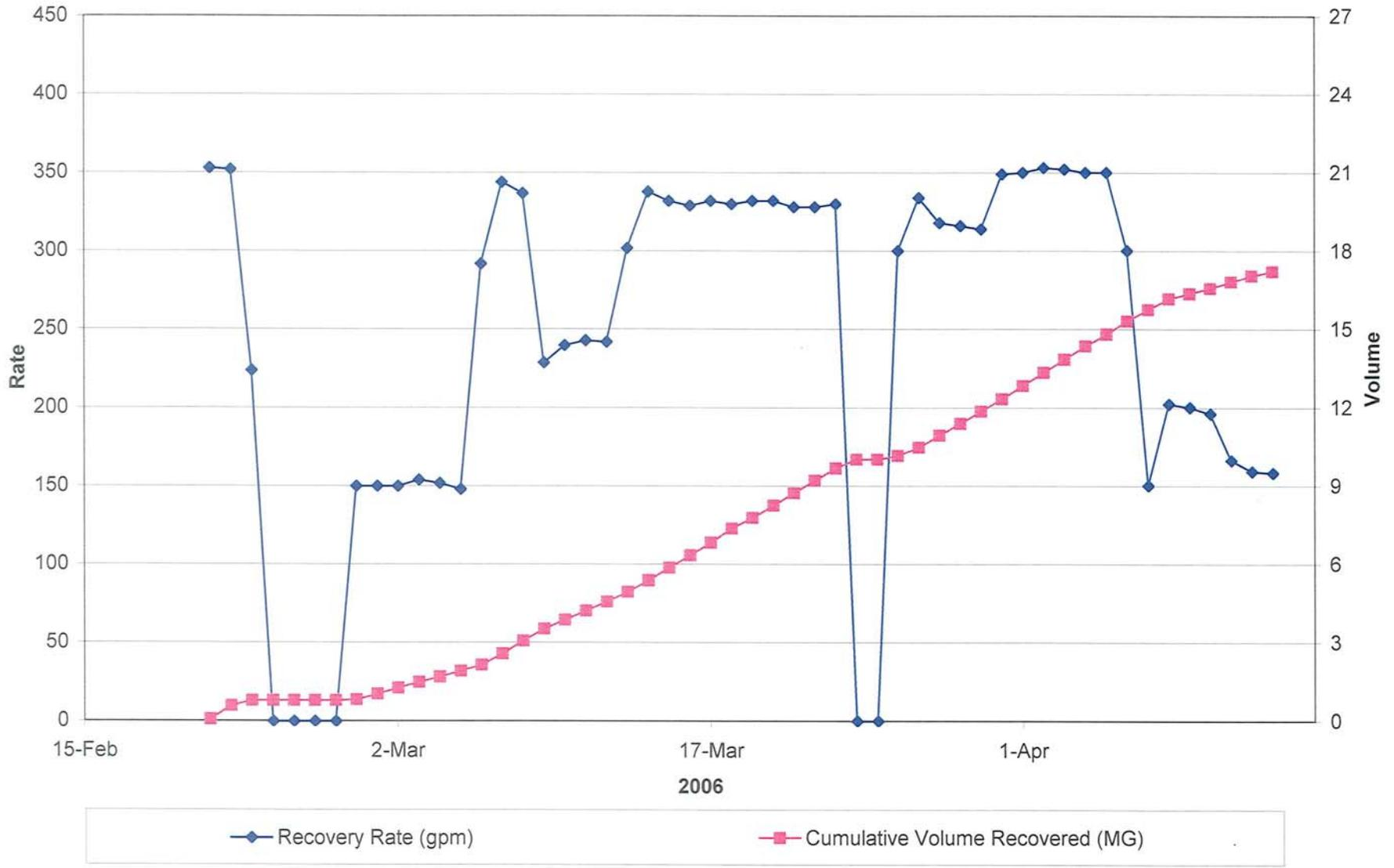
FIGURE 3-33. PLOT OF RECOVERY RATE AND CUMULATIVE VOLUME RECOVERED FOR ASR WELL 5 DURING CYCLE 5
