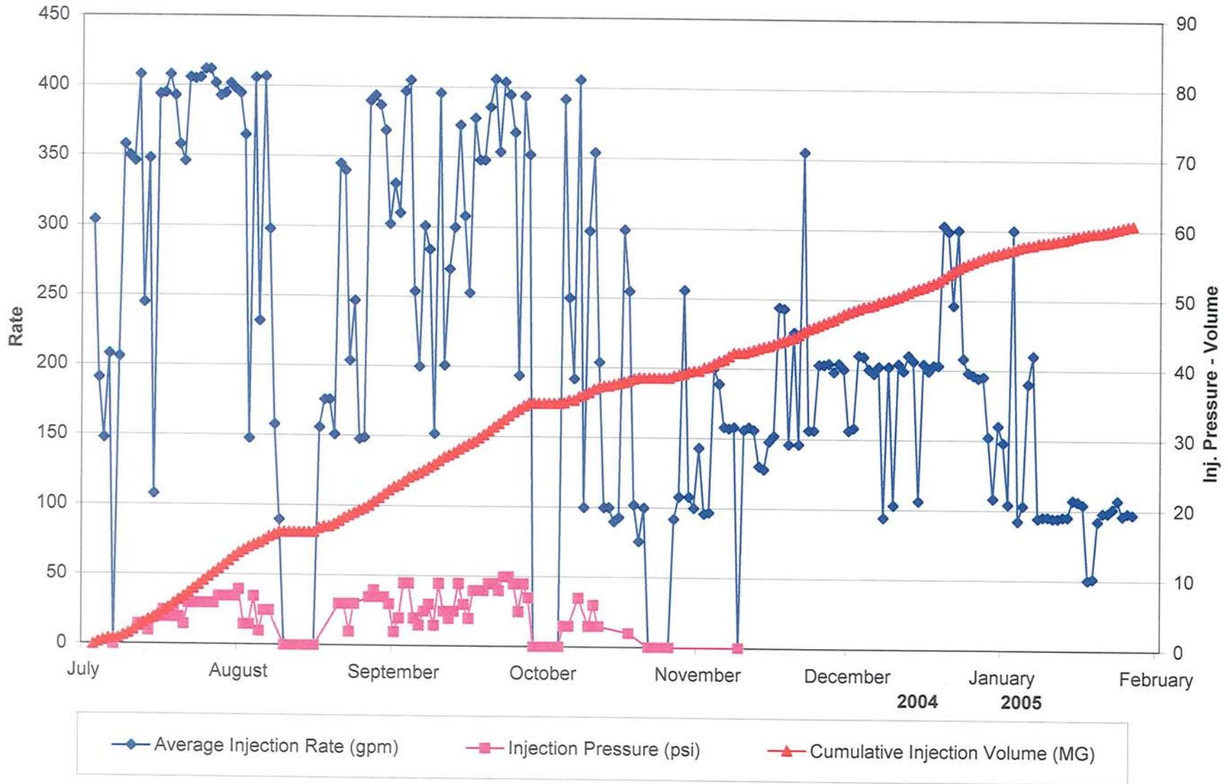
FIGURE 2-7. PLOT OF INJECTION PRESSURE, RATE, AND CUMULATIVE VOLUME INJECTED INTO ASR WELL 5 DURING CYCLE 4
