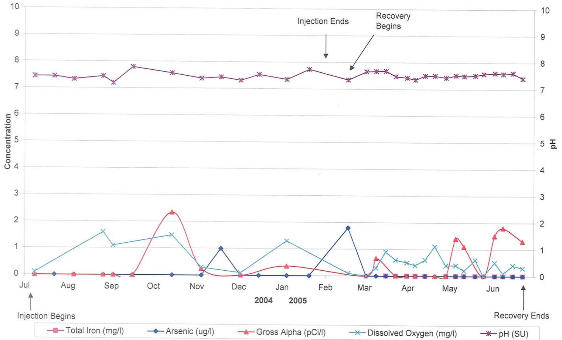
**FIGURE 2-13. PLOT OF WATER QUALITY IN STORAGE ZONE OBSERVATION WELL 3 DURING CYCLE 4 (PART 1)**
