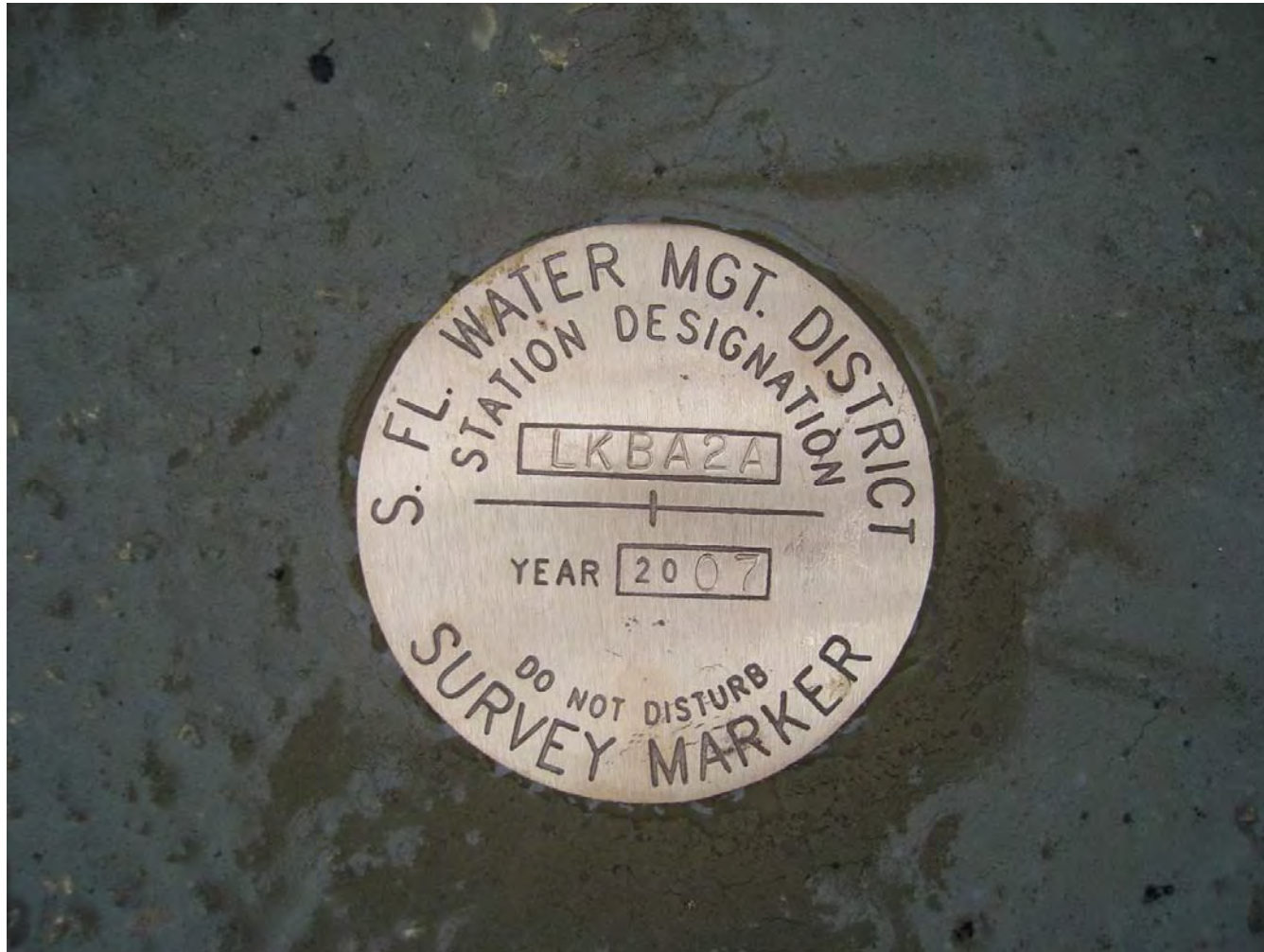
Nick Miller, Inc. Date of Photo: February 15, 2007 View: A top view of the benchmark
