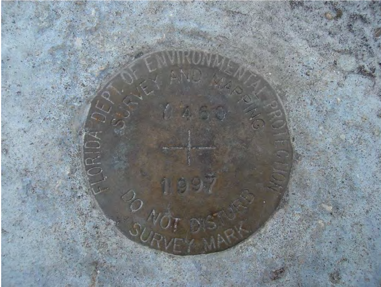
Nick Miller, Inc. Date of Photo: February 15, 2007 View: A top view of the NGS benchmark Y 460
