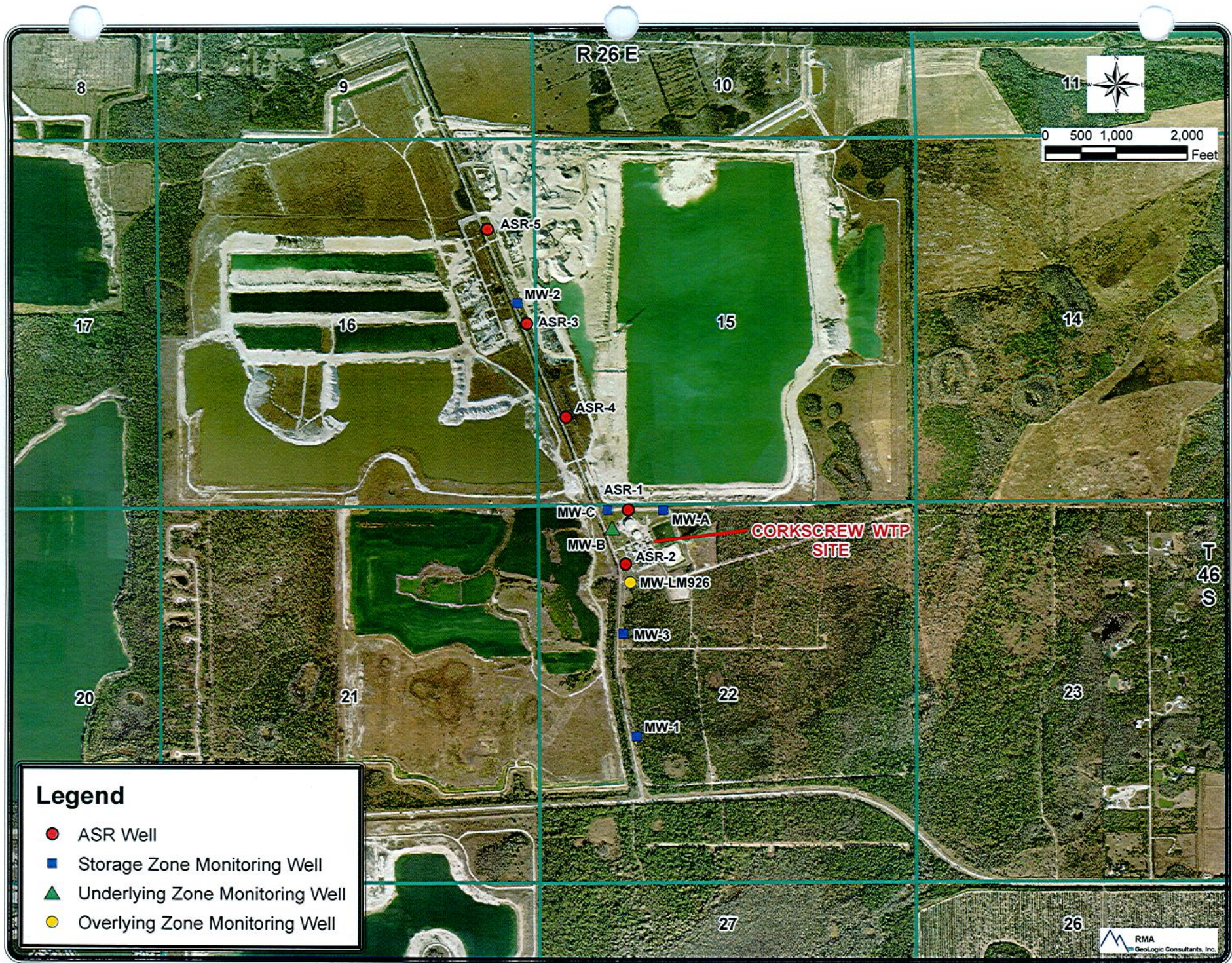
FIGURE 1-2. AERIAL PHOTO SHOWING LOCATION OF CORKSCREW WTP ASR SYSTEM WELLS.
