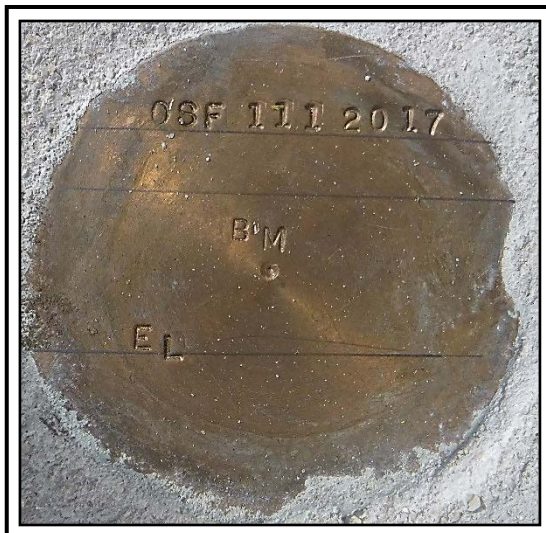
3¼" Brass disk stamped "OSF 111 2017 EL" El.62.594 NAVD88
