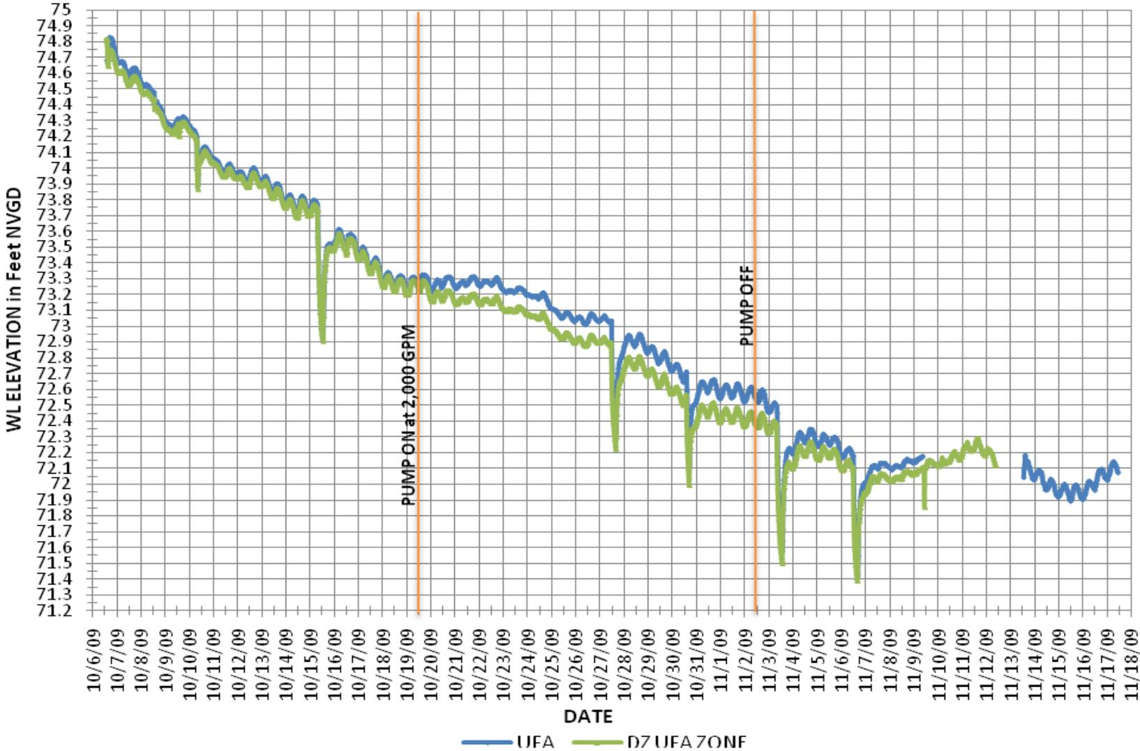
Figure 3-18. Aquifer Performance Test SE-SA-MW1 Water Levels
