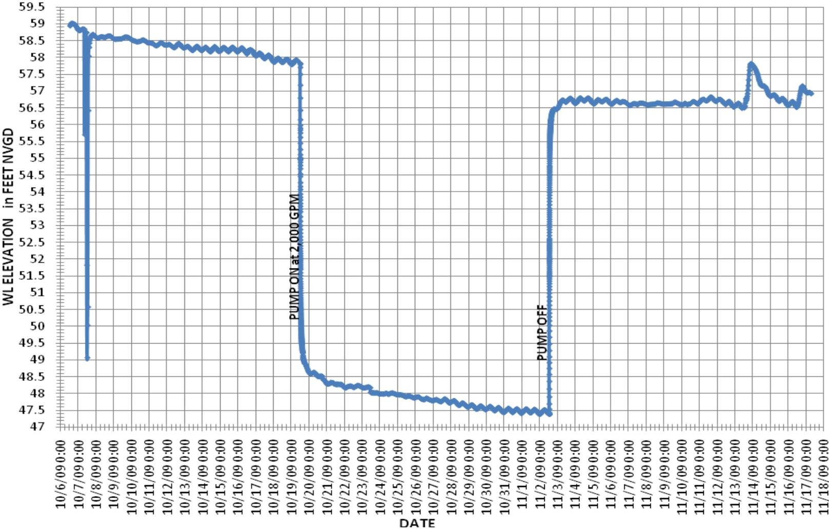
Figure 3-17. Aquifer Performance Test SE-UFA-MW1 and DZ-UFA Zone Water Levels
