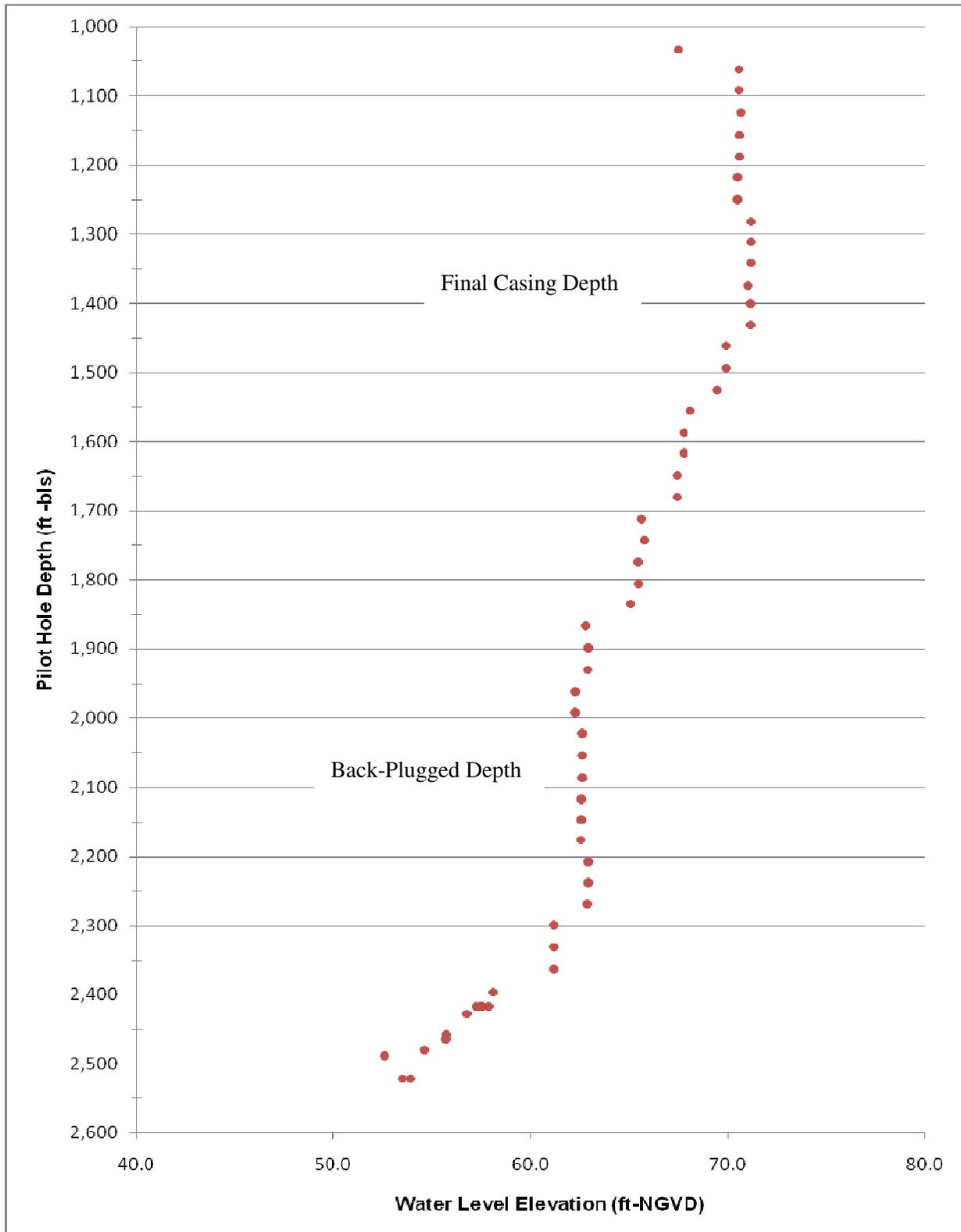
Changes in water level elevations as depicted in **Figure 3-1** indicate that flow in the borehole is downward and changes in formation permeability, and /or changes in water quality occur at approximately 1,250 ft bls, 1,430 ft bls, 1,550 ft bls, 1,700 ft bls, 1,860 ft bls, 2,290 ft bls and 2,390 ft bls.
