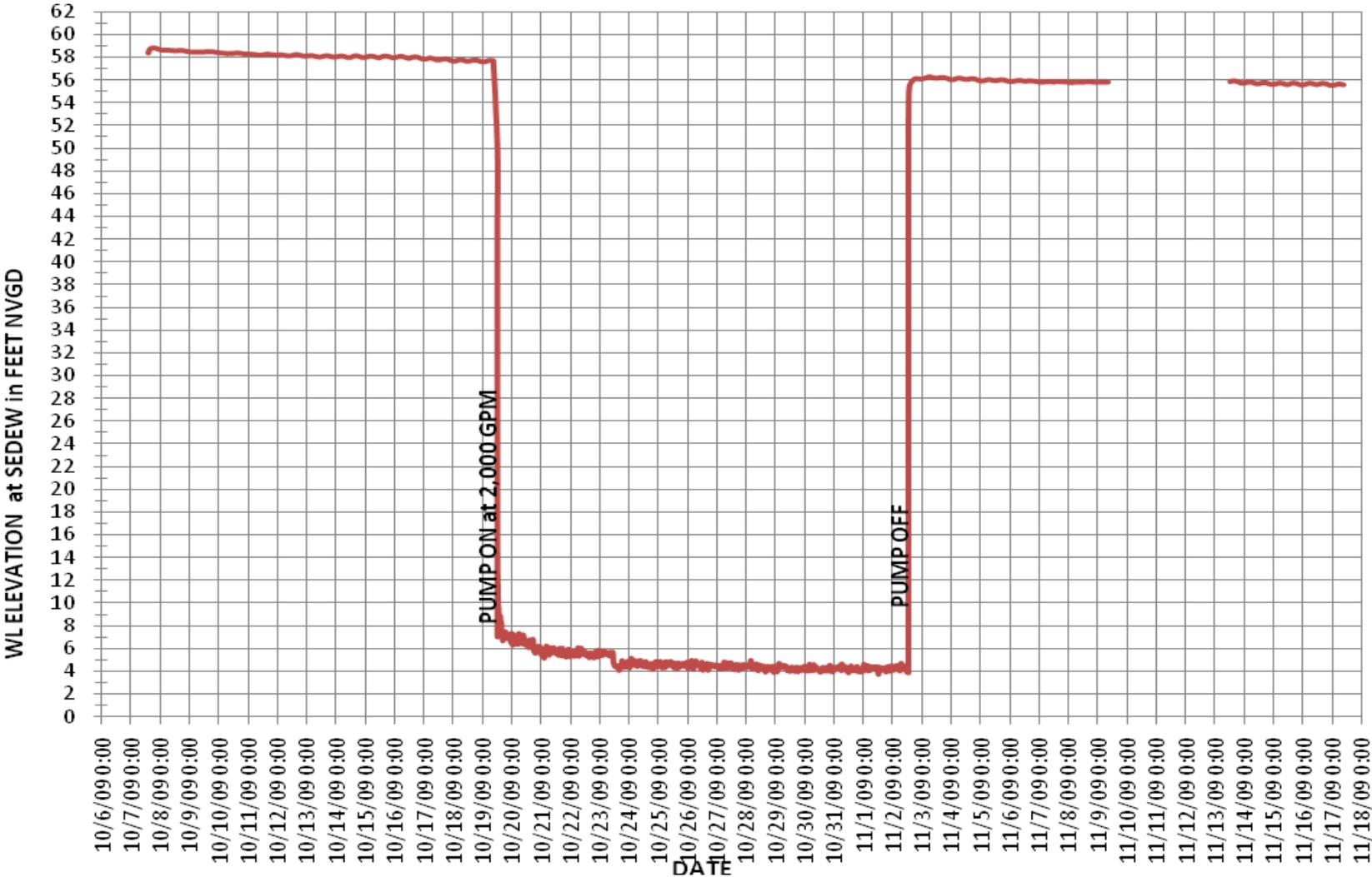
Figure 3-16. Aquifer Performance Test DZ LFA Zone Water Levels
