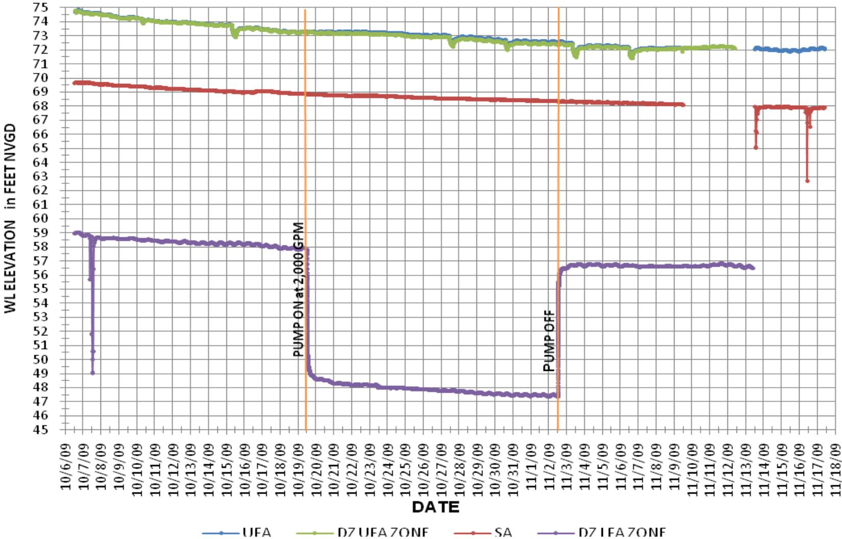
Figure 3-15. Aquifer Performance Test SE-DEW Water Levels
