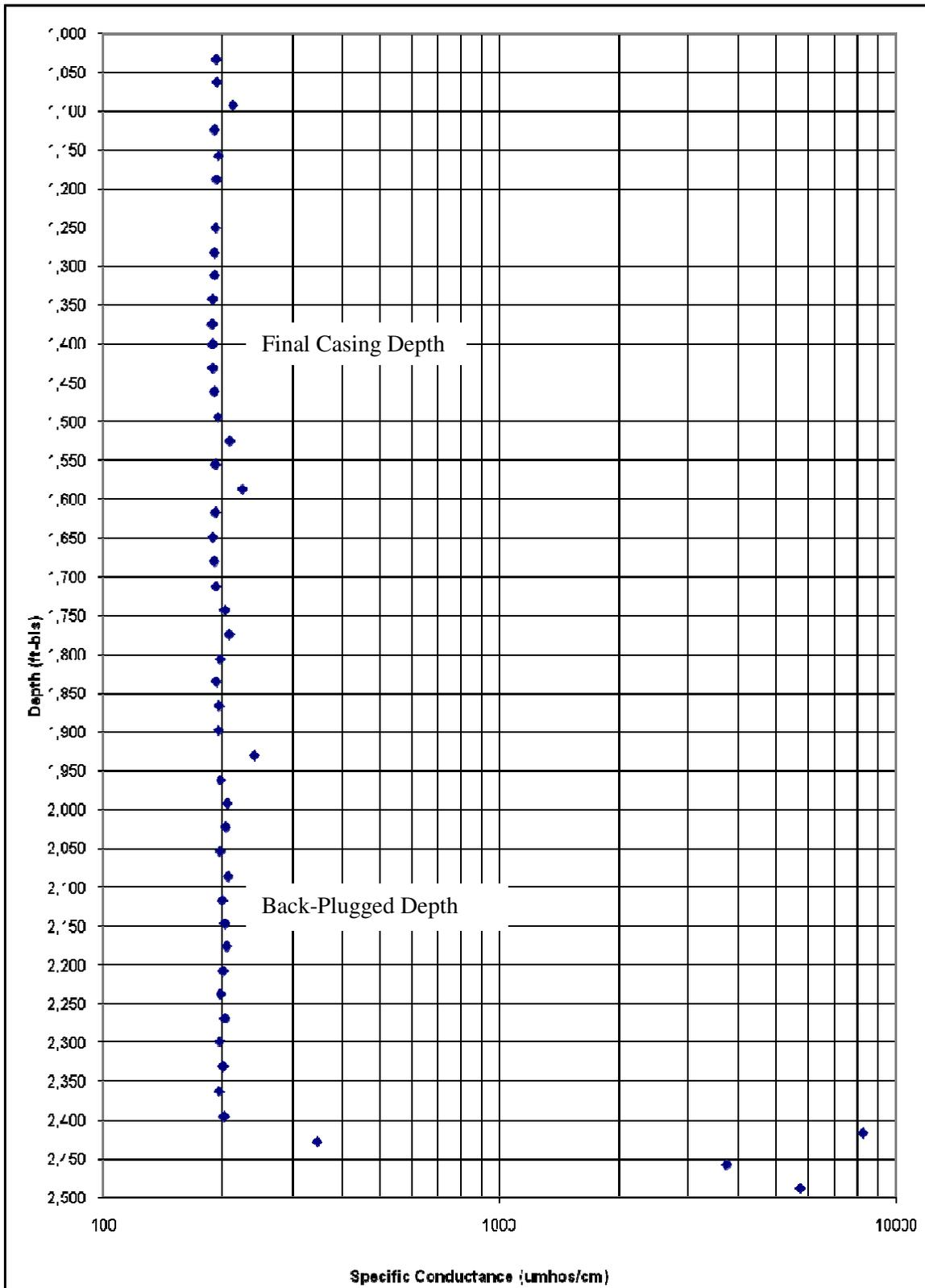
Figure 3-8. Laboratory Specific Conductance ( $\mu\text{mhos/cm}$ ) vs. Depth
