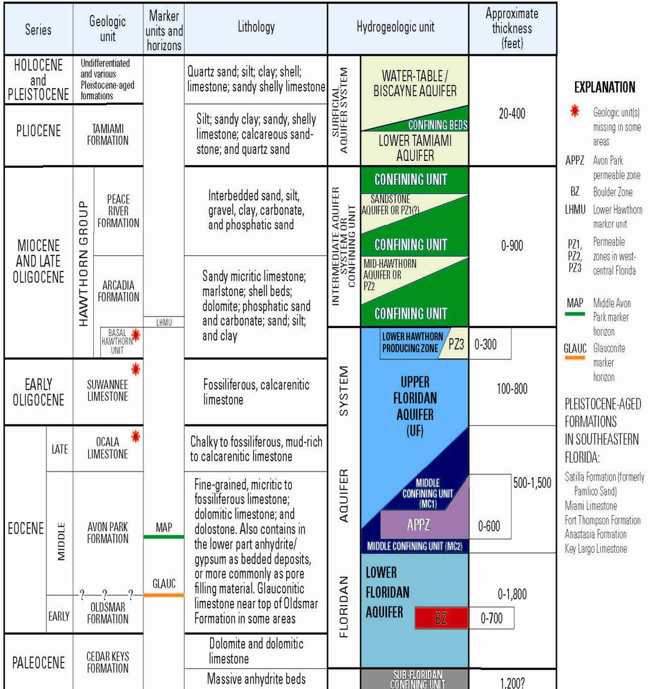
The geologic units that compose the UFA include the Suwannee Limestone, the Ocala Limestone and the upper part of the Avon Park Formation. The surface of the UFA is the remnant of an ancient karst plain, and generally exhibits considerable irregularity throughout Polk County. Sink-hole type depressions on the surface of the aquifer are common. (Spechler and Kroening, 2006).
