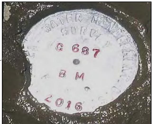
Aluminum cap stamped "C687 BM 2016" El. 23.267 NAVD88
