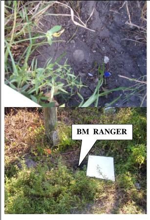
To reach the benchmark from the intersection of Jog Road and S.R. 80, go west on S.R. 80 for 2.4 miles to Sandsburys Way on the right. The benchmark is a Palm Beach County Brass Disk set in concrete and stamped "Ranger". Being 457' north of the centerline of S.R 80, 30' east of the centerline of Sandsburys Way And 3' west –southwest of a witness sign in a wooden power pole and 1 foot below the ground.
