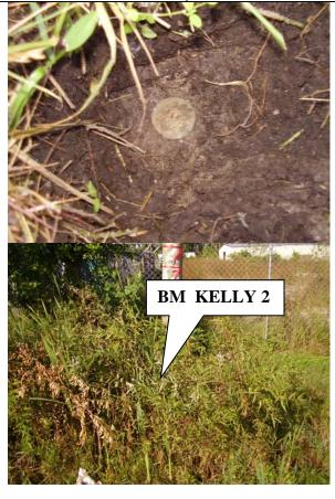
To reach the benchmark from the intersection of Benoist Farms Road S. and S.R. 80, go west on S.R. 80 for 0.25 miles to Kelly road on the right. The benchmark is a Palm Beach County Brass Disk set in concrete stamped "Kelly 2". Being 629' feet N. of the centerline of S.R. 80 (Southern Blvd.), 30.5' W. of the centerline of Kelly Dr. and 2' E. of a witness sign in a wood power pole.
