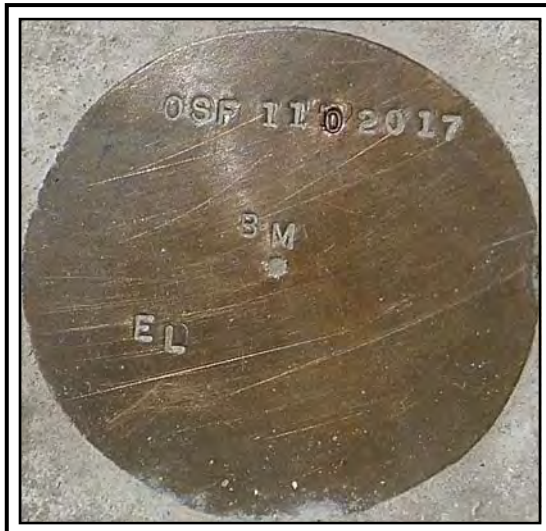
3¼" Brass disk stamped "OSF 110 2017 EL" El. 62.593 NAVD88
