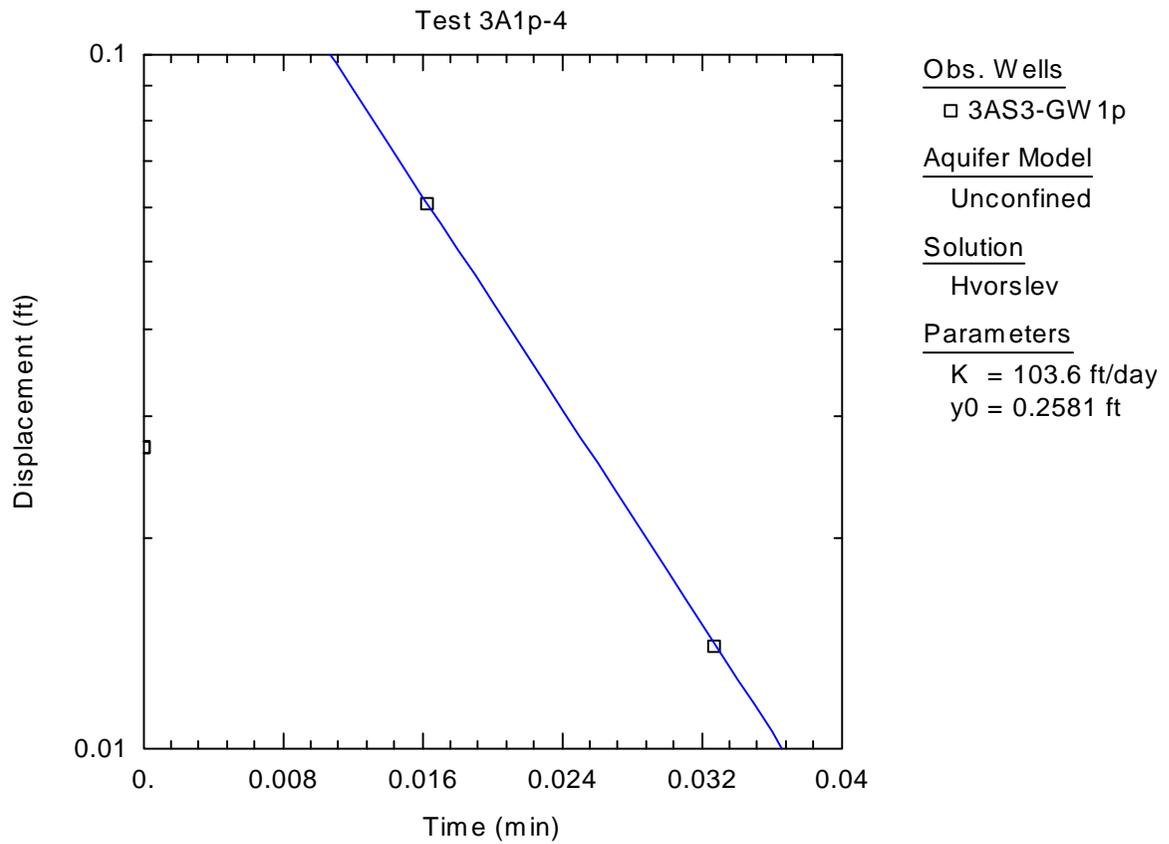
**Figure C-4.** Graphical Representation of Raw Data Obtained from Slug Test of 3AS3-GW1p, Hvorslev Solution
