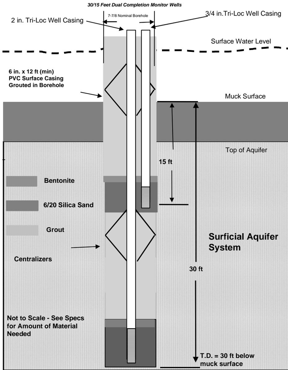
Figure 4. General Schematic of Dual Zone Monitor Well
