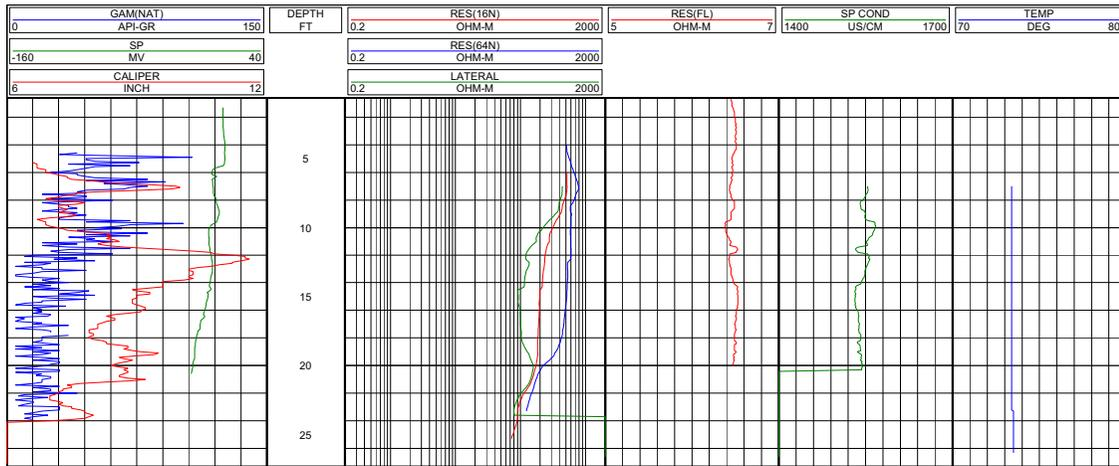
Figure B-33. Geophysical Logs for Well 3AS3-GW2
