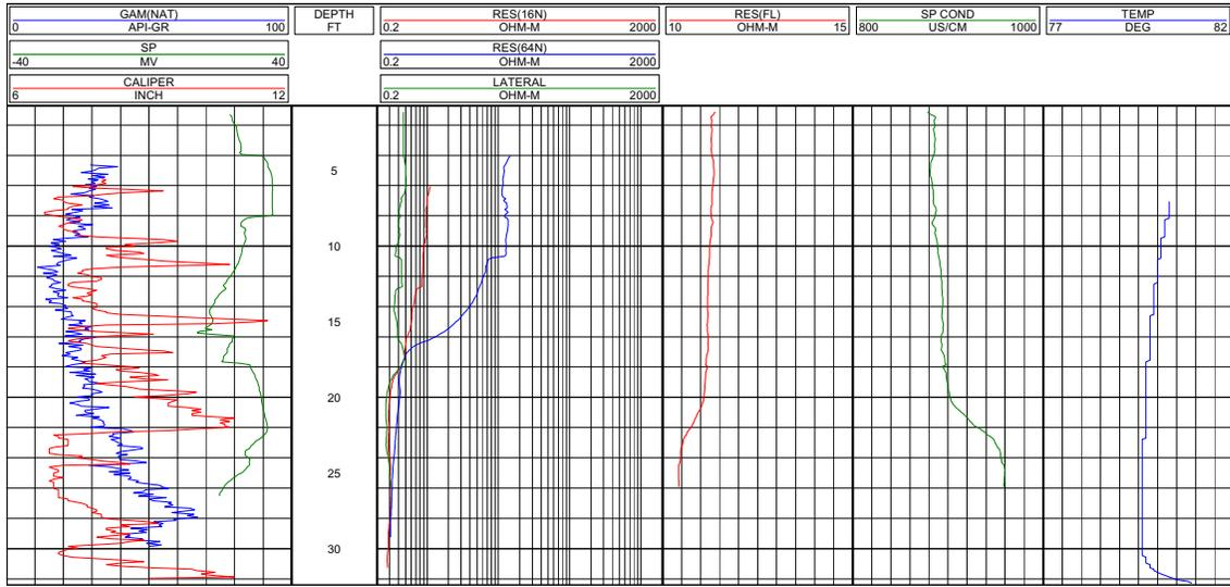
Figure B-36. Geophysical Logs for Well 3BS1-GW1
