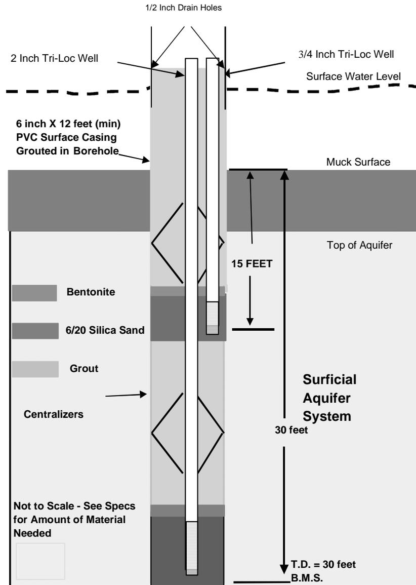
Figure A-10. 30/15-ft Dual Completion Monitor Well
