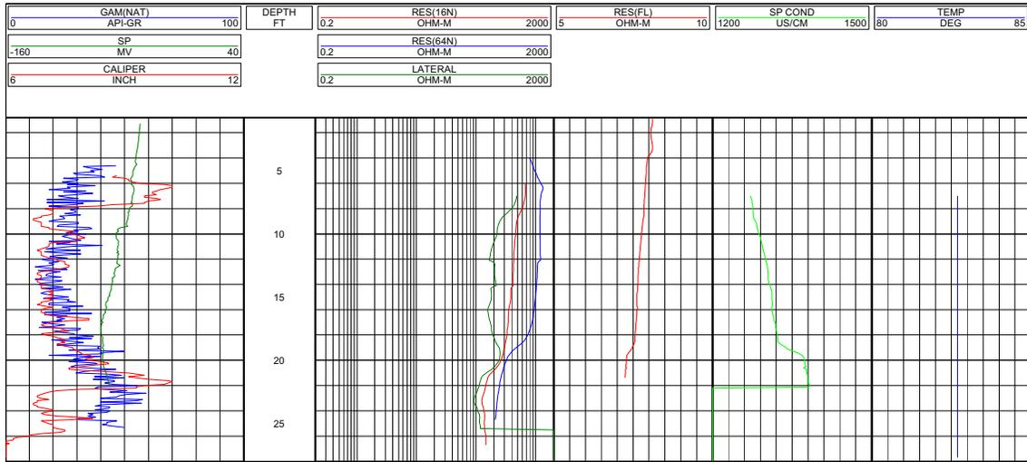
Figure B-38. Geophysical Logs for Well 3BS1-GW3
