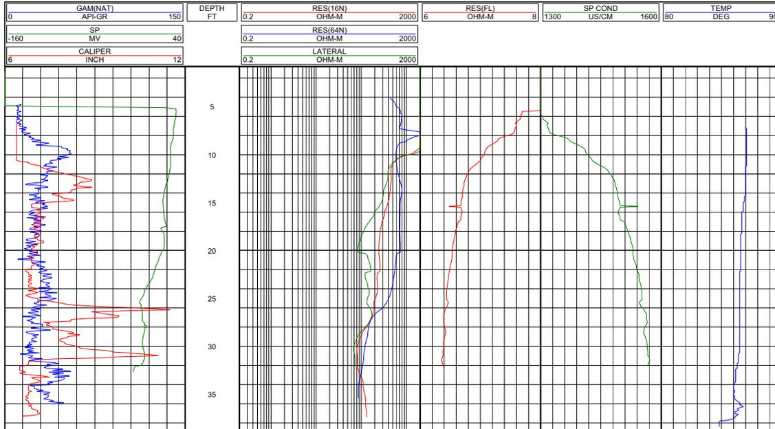
Figure B-39. Geophysical Logs for Well 3BS1-GW4
