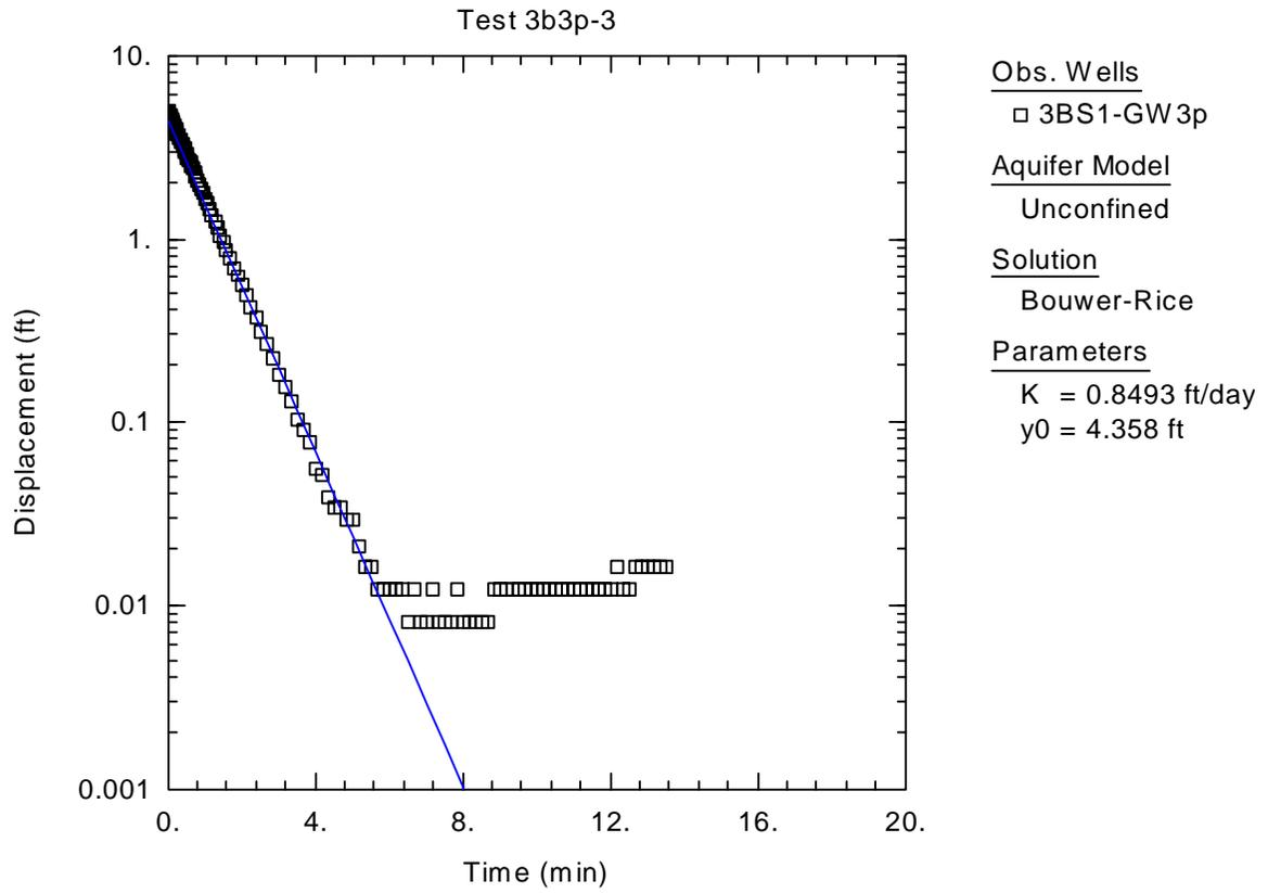
**Figure C-19.** Graphical Representation of Raw Data Obtained from Slug Test of 3BS1-GW3p, Bouwer-Rice Solution
