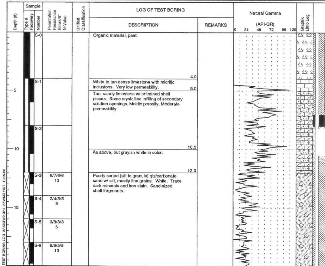
Figure B-18. Test Boring Log for Well 3AS3-GW2 (Sheet 1 of 2)
