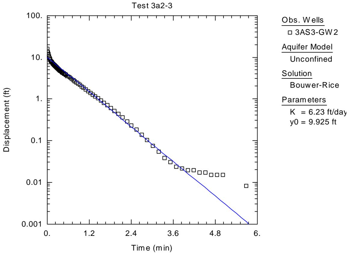
**Figure C-5.** Graphical Representation of Raw Data Obtained from Slug Test of 3AS3-GW2, Bouwer-Rice Solution
