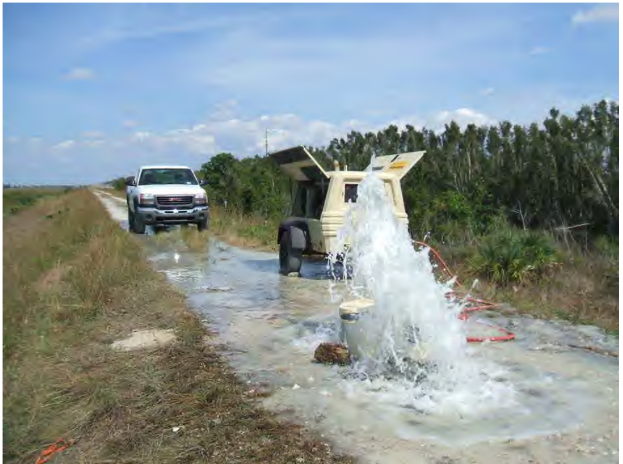
7.5" OPEN BOREHOLES BEING AIR LIFTED WITH COMPRESSOR FOR 3 HOURS EACH PRIOR TO BEING LOGGED BY THE U.S.G.S.
