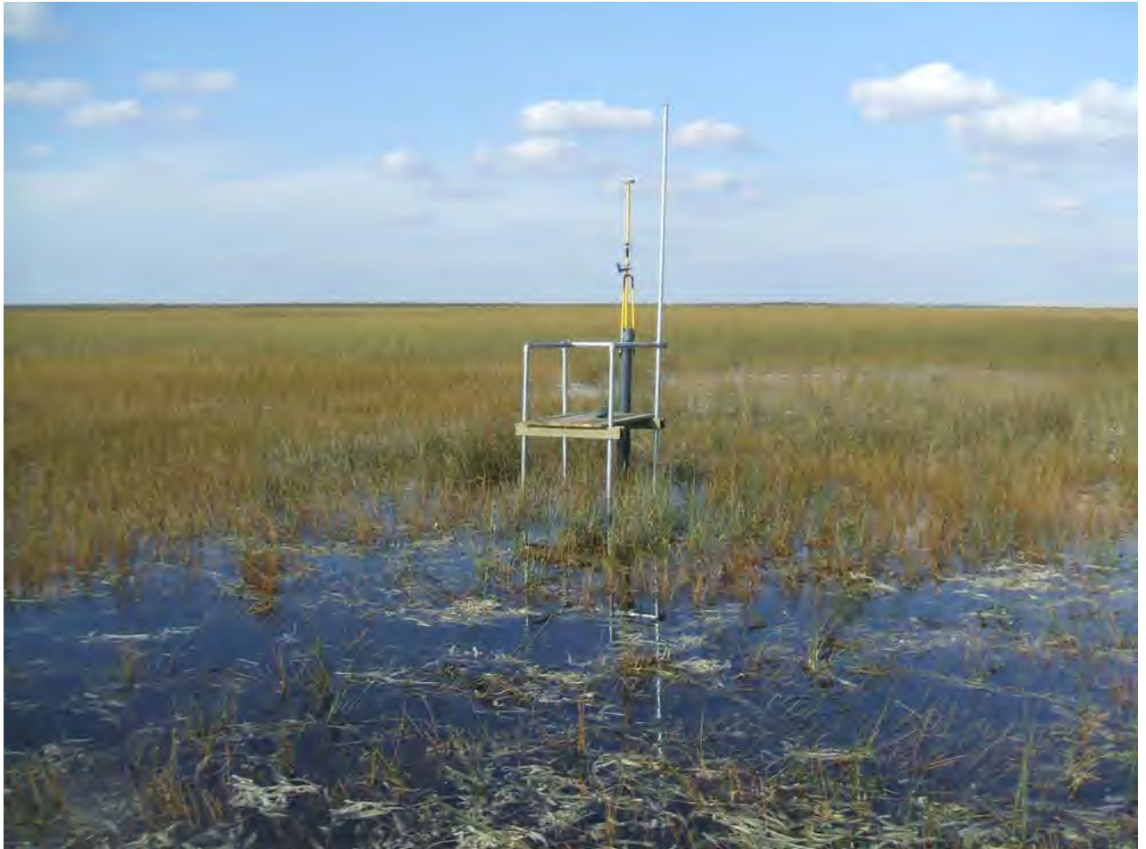
MONITORING WELL PLATFORM
