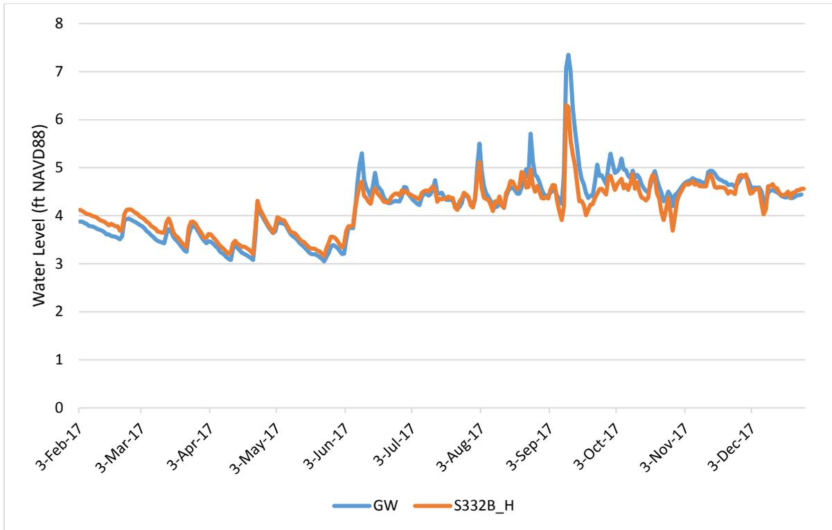
Figure 12. Water levels at site P-6 (L31NW06).
