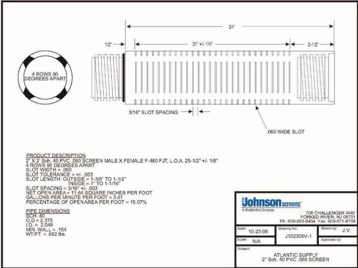
Figure 2. Sample Well Screen Specification
