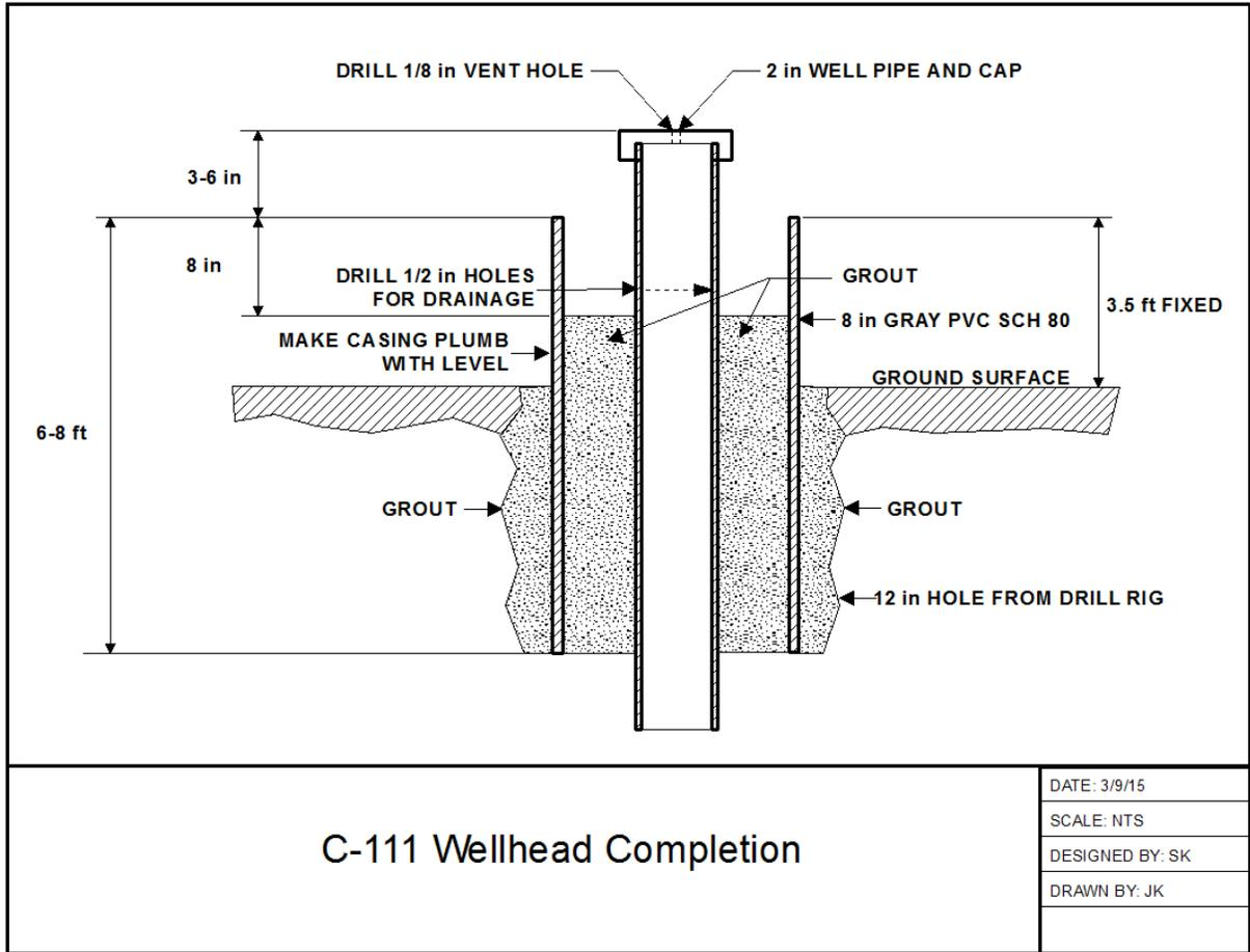
Figure 3. Wellhead Completion Details
