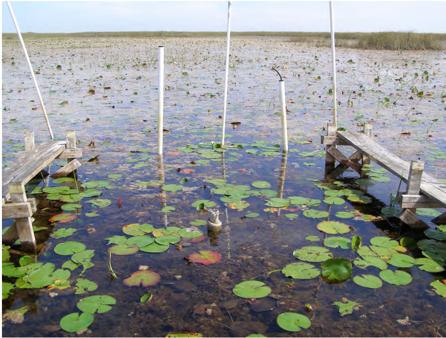
Figure 12: Porewater wells and SET in slough, east of island (view looking north)
