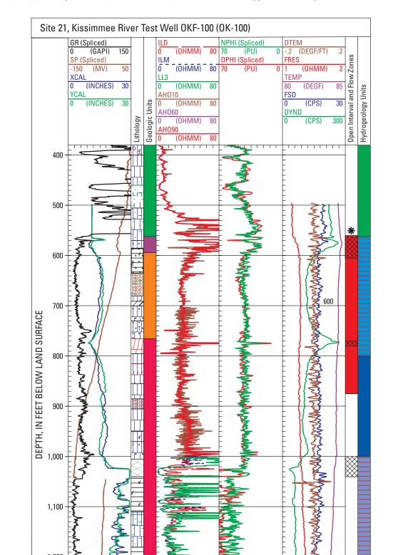
Open interval is for well EXKR-1 (OK-101) at the same site. Well OKF-100 has not been completed, but casing was set at 565 feet.
