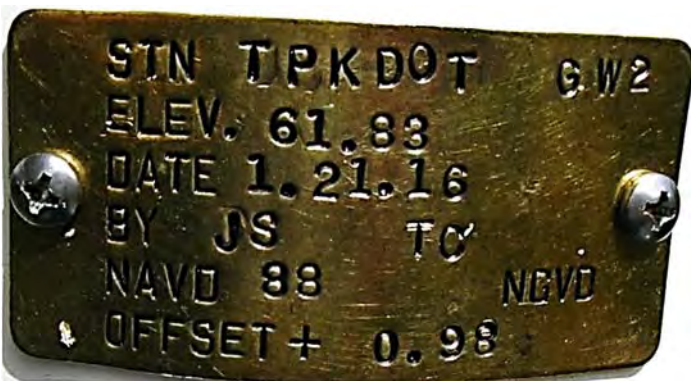
Old NAVD88 Brass Tag (to be removed)
