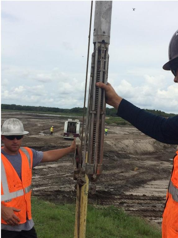
Photo 6. Caliper Tool Close Up With Logging Unit in Background
