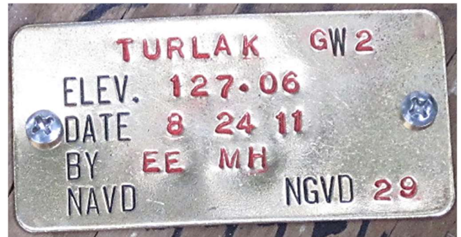
Old NGVD29 Brass Tag Close-up (removed)
